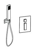
7. Install the shower head using the provided swivel joint. Once secure, tighten the set screw located on the swivel joint using the provided hex wrench.
