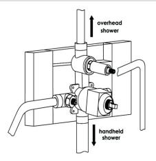
4. Once all piping is routed and connections have been made, use a/2 test plug to perform a water pressure test. Turn on the main water supply to your home and water test the installed plumbing. Ensure that there are no leaks, then shut the water off. Remove the testplug.
