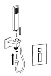
6. Slide the decorative back plate onto the shower arm, and install the shower arm by threading it into its prepared female fitting. Apply thread sealant or plumber's tape to the threads before tightening. Hand tighten firmly.
