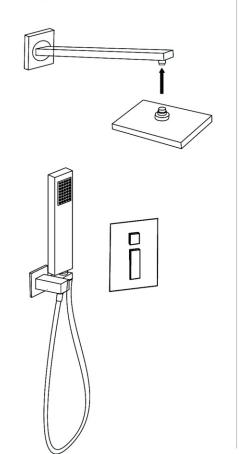
8. Turn the main water supply back on, and test the completed shower system. Ensure that there are no leaks and that all functions are working properly.
