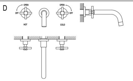
4. The decorative cover needs to be close to the wall, and the outlet is straight down after correct installation like the above figure.
