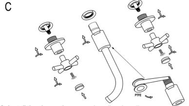
3. Install the decorative cover, handles, handle covers and outlet nozzle on the valve body in turn, after fixing the valve body and restore wall trim. (The thread which connecting the outlet nozzle to the valve body should be twined with Teflon tape to prevent water leakage.)
