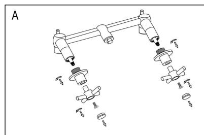
1. Remove the handles and decorative covers to avoid the damage which caused by knock during the installation.
