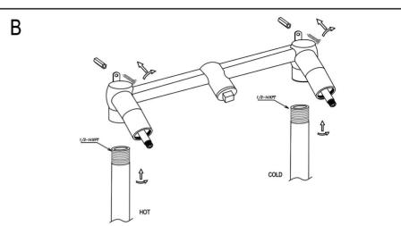
2. Fix the valve body to the reserved water pipe with 1/2-14NPT thread in the wall , connect the hot and cold inlet to the valve body ,and then test for the tightness
