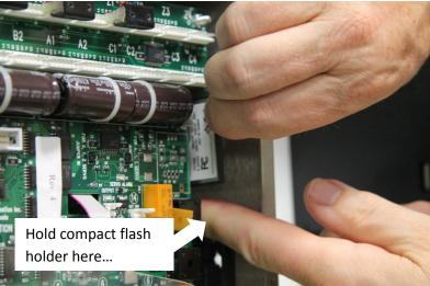
Carefully pull the compact flash out with one hand while holding in the compact flash holder with the other hand as shown.
