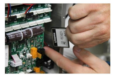
Pull the compact flash out as shown. Carefully observe which way it is installed so you can re-install the new one the same way.
