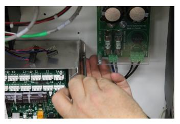
Next put in the top right screw as shown. This is the easiest one to install.
