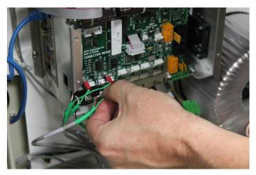
Work your way around carefully unplugging all the cables. Pull the connectors off by grabbing the connectors.
