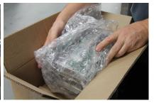
Before packing re-install the plastic cover. This will protect the A2MC during shipping and keep packing material from getting inside the controller. Ship it inside an appropriate box and make sure it is well packed with bubble wrap. Bubble wrap is not enough on its own, the A2MC needs to be in a sturdy shipping box. If using foam, wrap it in plastic first to protect the A2MC from static.
