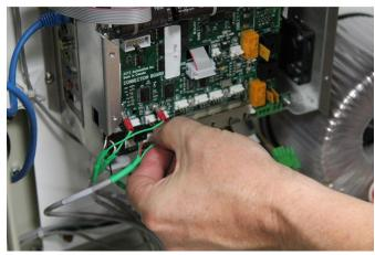
Now plug in all the cables and connectors referencing pictures and notes that you made earlier before un-installing the A2MC.
