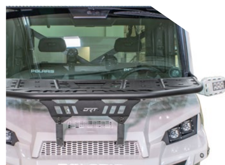
The DRT Ranger XP Hood Rack comes with both 2013-2018 and 2019+ brackets.
