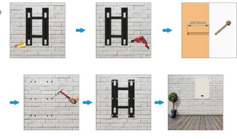
6. Raise the battery a little higher than the mounting frame whilst maintaining the balance of the battery. Hang the battery on the frame through the match hooks.
