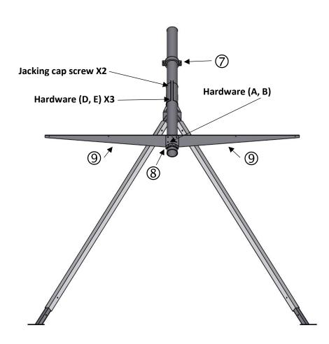
7. Pre-assemble the **Wing mount weldment (8) and Wing Frames (9)** on the ground or a bench with **Hardware (A, B)**. Line up the top of the Wing assembly with a straight edge and torque bolts to **42 ft-lbs.**
