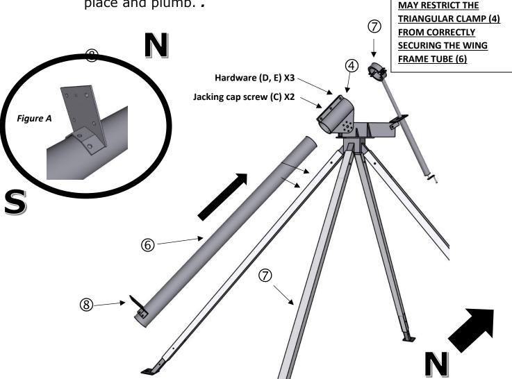
6. Install the *Wing frames (9)* to the lower *Wing mount weldment (8) with Hardware (A, B)*. Tighten by hand and then place a straight edge on top to ensure each component is straight before *torquing Hardware (A, B)* to 42ft/lbs. Once Torqued and the Wing assembly is level completely loosen the *Jacking cap screws (C)* and torque *Hardware (D, E)* and the *Jack clamp (7) Hardware to 64ft/lbs*.
