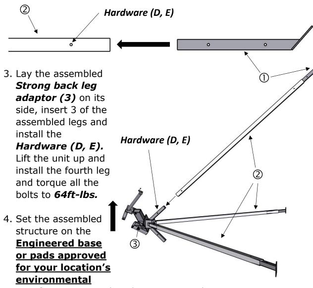
**requirements.** Anchor the 4 points and torque to manufacturer recommended specifications.
