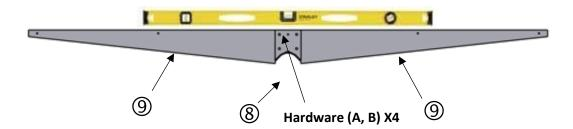
8. Install the top **Wing frame (9)**, **Wing frame weldment**(8) assembly with **Hardware (D, E, F)** place a level on top to find perfect level and **Torque to 42 ft-lbs.** Each Bolt should have a washer on the inside of the **Wing**frame tube (6) and on top of the **Wing mount**weldment (8).
