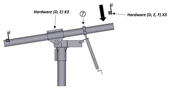
8. Install the remaining Kinetic rails with proper Kinetic hardware and continue with the installation of the solar modules.
