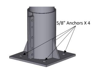
3. Raise the **Post** (2) to a vertical position near the anchored base. Insert the bottom of the post into the **Base plate** (1). Once installed, remove **Jacking cap screws** (C) and toque **Hardware** (D, E) to 64ft-lbs. Check post with a level and shim the baseplate if necessary.
