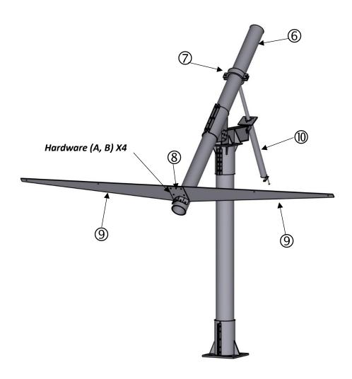
6. Lay out the top **Wing frame (9) and Wing mount weldment (8)** on the ground or a bench. Line up
