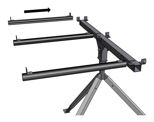
7. Slide the 2 longer lengths of Kinetic rail into the Kinetic Stud + Square nut on center and tighten hardware.
