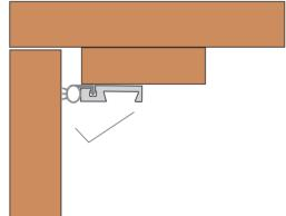
**4.1** Test the door for correct fitment by inserting a sheet of paper between the door and the door seal. Shut the door and adjust the seal to ensure a consistent seal
