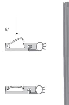
**5.1** Once installed correctly, fit the cover cap over the screws by inserting one end first then the other.
