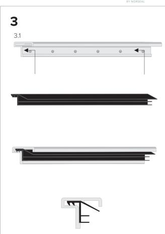
${\bf 3.1} \ {\it Place} \ the \ gasket into \ the \ holder, \ push \ firmly \ along \ the \ whole \ length \ of \ the \ insert \ ensuring \ its \ firmly \ in \ place.$
