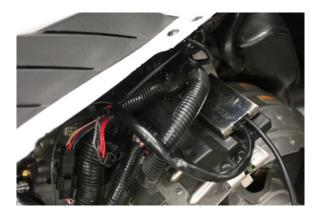
12. Using the supplied velcro attach the EZ-Jacker enclosure to the factory ECU enclosure.
