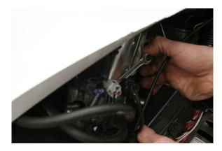
9. Using a 10 mm wrench remove the nut on the engine side of the Boost Solenoid. Attach the ground connection on the EZ-Jacker and re-install the 10mm nut.
