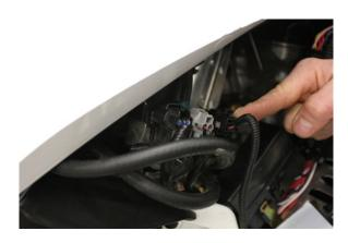
7. Locate the stock Boost Solenoid connector
