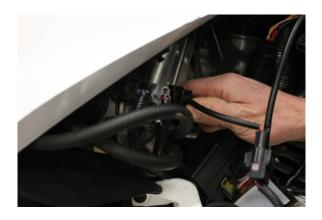
8. Plug the matching EZ-Jacker connectors inline with the EFI connector.
