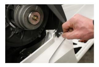
2. Un-fasten the dzus fastener on the bottom of the rear cowl next to the footwell.
