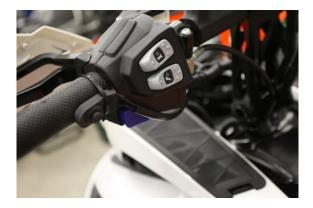
10. Install the supplied push button onto the handlebar. The push button can be installed using a zip-tie as shown in the image or super glued to the switch pod bellow the thumb warmer switch.
