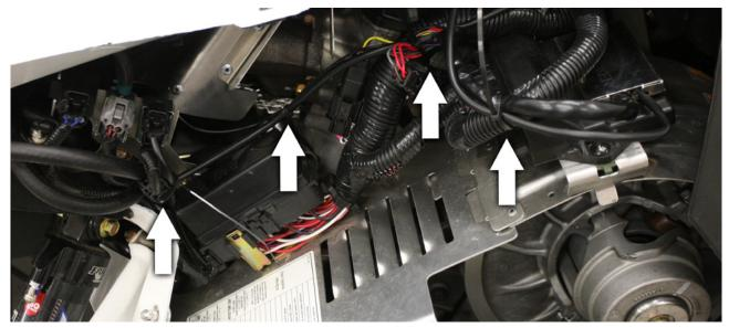
13. It is very improtant to secure the EZ Jacker wiring so that is out of the way of heat and moving parts. Using the supplied zip-ties we recommend securing the harness in the locations shown above.
