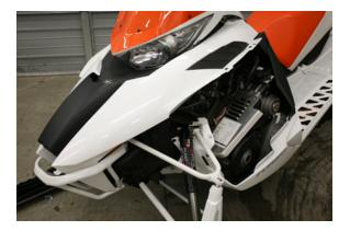
1. Remove side-panel on clutch side by removing the cotter pin located behind the upper a-arm.
