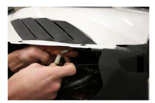
11. Route the push button wiring down the steering column to under the hood and connect to the matching connector on the EZ Jacker.
