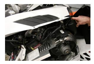
3. Pull back the cowl and locate the MAP sensor. Remove the stock connector from the MAP sensor.
