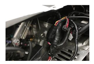
6. Plug the matching EZ-Jacker connectors inline with the EFI connector.
