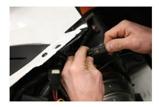
4. Plug the matching EZ-Jacker connector into the MAP sensor and the stock MAP sensor connector into the other matching EZ-Jacker connector.
