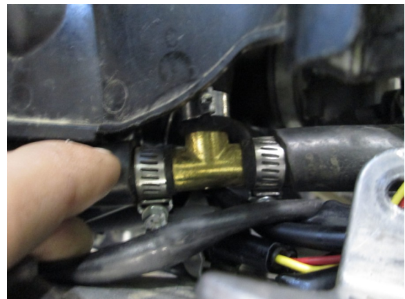
18. Cut stock fuel line on the straight part of the line. Elsewhere might leak. Install auxiliary injector and clamp both cut ends of stock line.
