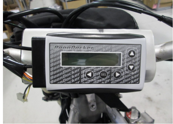
2. Mount control box to handle bars. Route along stock wire harness to the air box area.
