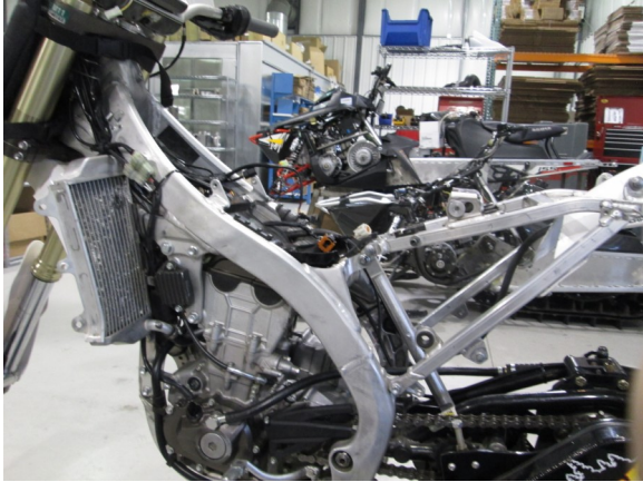
1. Remove seat, panels, tank, air box, silencer & header.
