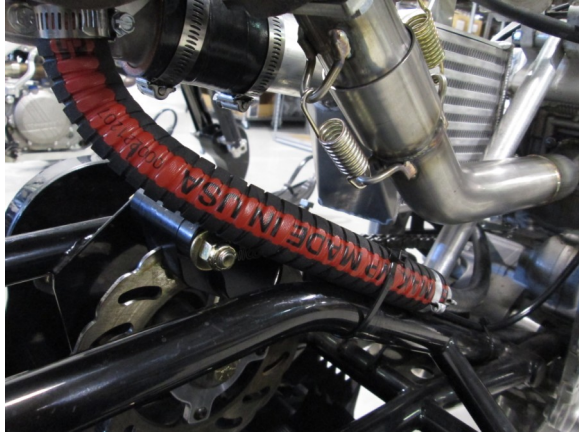
13. Rout oil drain line as shown and zip tie to Timbersled frame. Hook into the bottom of the turbo.
