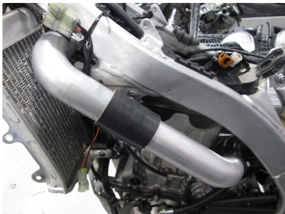
17. Install 90 deg. Charge tube and 90 deg. Silicone with 2 hose clamps on each silicone piece. Tighten all charge tube and intercooler clamps where they will not rub on anything after being positioned.
