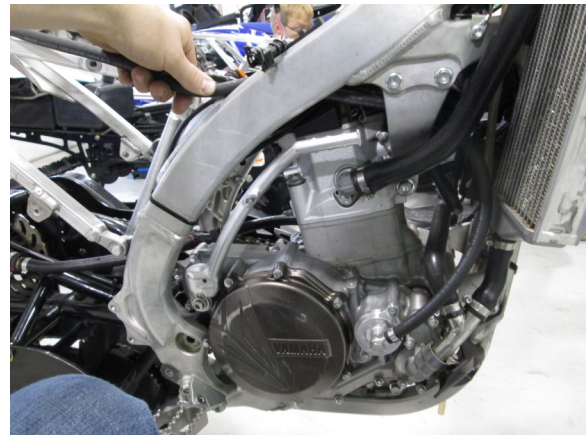
4. Install filter cover & oil feed line. Route line through frame to the sub frame & zip tie as shown above .
