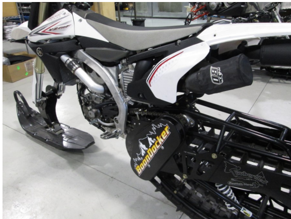
21. Install front side panels, tank, side panel and seat.
