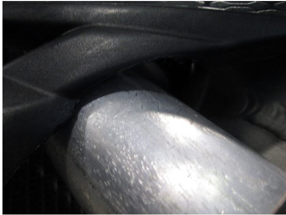
19. force left front panel to fit over charge tube.
