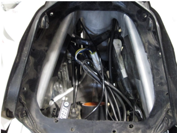
3. Remove air box components. Routing harnesses with the stock wiring harness Zip tying as needed.
