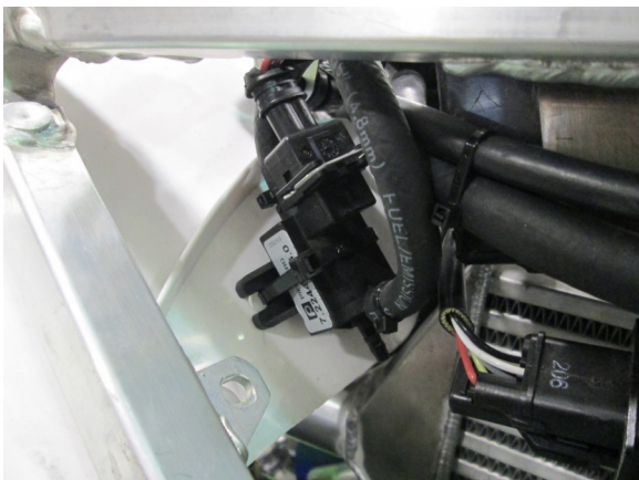
17. Drill holes & mount the Actuator solenoid on the rear fender. Plug in connector from the BoonDocker control box. Hookup lines as per control box instructions.
