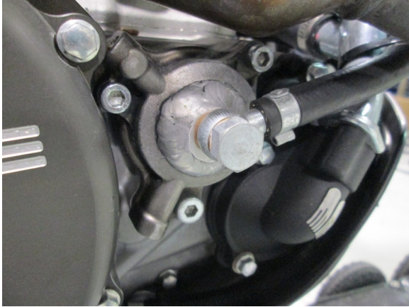
13. Install the oil feed cap for the oil feed line for the turbo. Install the oil feed line. NOTE: Make sure filter is installed correctly.
