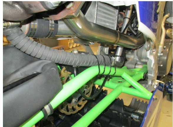
16. Route the oil drain line & zip tie in place. Install the drain line on to the turbo with supplied hose clamp.
