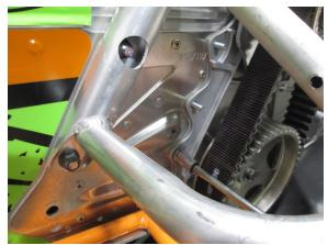
1. Remove front cross shaft bolt, and 4 belt drive case nuts.
