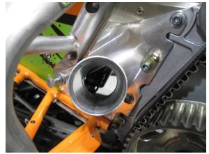
4. Install exhaust outlet tunnel support and 2 spring tabs both facing up.
