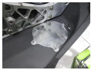
6. Rivet muffler block off plate in.
