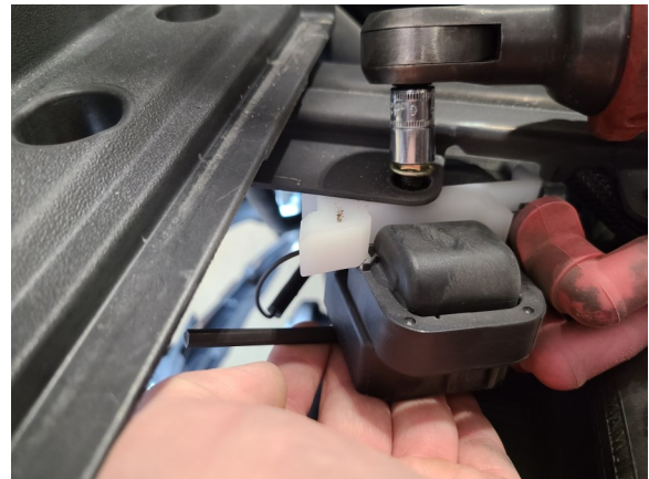
4. Using a 5mm allen and 10 mm wrench Remove the stock coil assembly.
