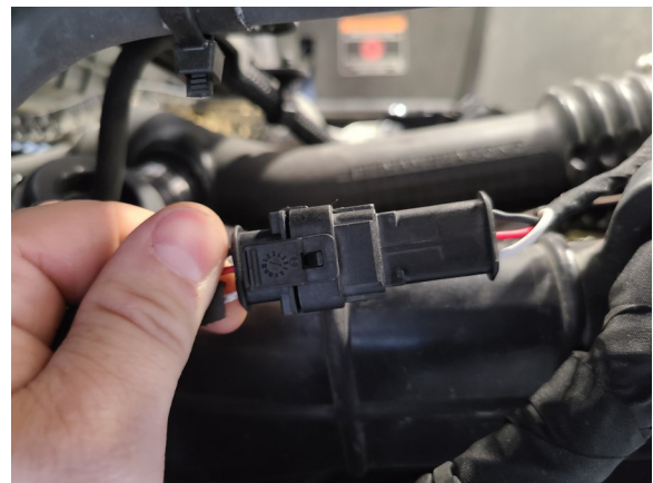
12. Plug wire harness into factory wire harness where previous coil assembly plugged into.
