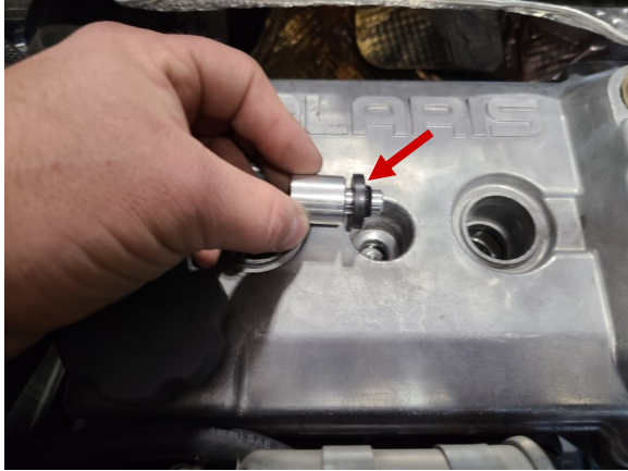
7. Install supplied aluminum spacer with valve cover isolator into center bolt hole of valve cover.
