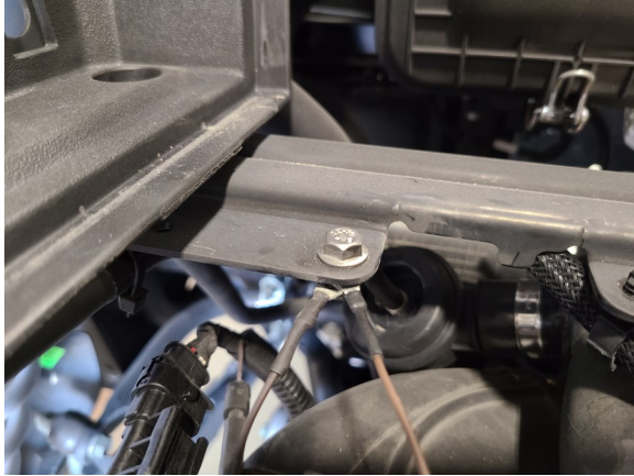
13. route and install both, factory ground wire and ground wire from supplied wire harness, to stock coil mounting position using supplied short flange bolt and nut.
