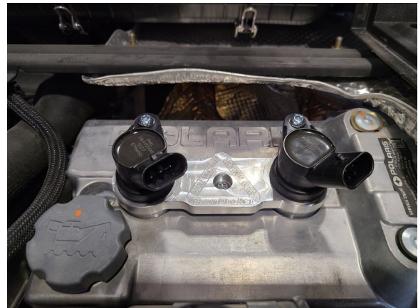
10. Install coils to mount using supplied short T30 bolts. (NOTE) Torque spec is 7FT LBS (10NM)
