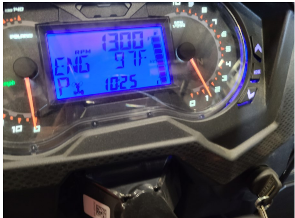
16. Start vehicle and verify Engine is idling properly
