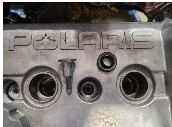
6. Using a T40, remove the center valve cover bolt and valve cover isolator.
