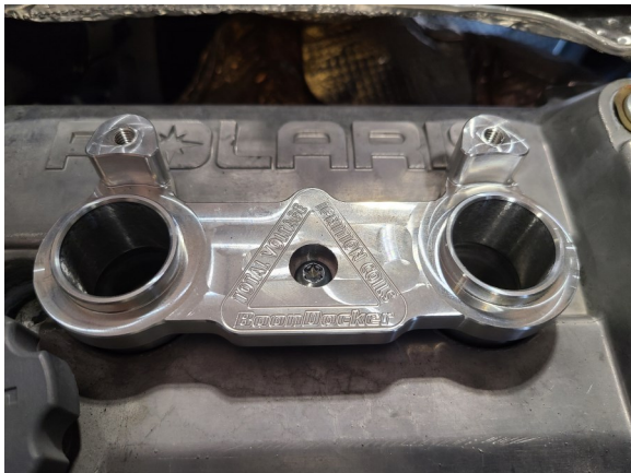
9. Install Total voltage billet aluminum bracket to valve cover using supplied long T30 bolt. (NOTE) Torque spec is 7FT LBS (10NM)
