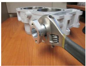
3. Use a wrench to tighten the housing until it is snug against cylinder (Do not over tighten).
