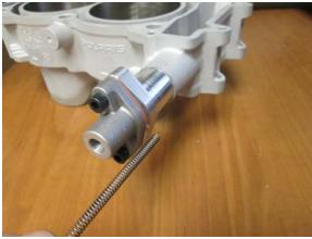
7. Before installing the tensioner spring assembly, check that all timing components are placed and correctly in time, then insert a small screw driver into the hole to push the plunger shaft making sure the plunger moves freely.
