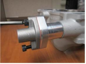
6. Tighten the tensioner onto the plunger housing using the M6 x 25 bolts, tighten to 7 ft-lb.
