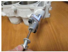
8. Install the tensioner spring assembly into the tensioner body and torque to 12 ft-lb.
