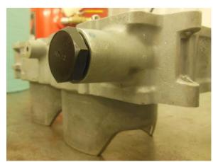
1. Locate and remove the stock timing chain tensioner on the MAG side of the cylinder.
