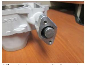
4. Cover the plunger with engine oil then push into the tensioner body as shown.
