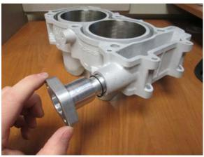
2. Place the included washer between cylinder and tensioner body, then screw the tensioner body clockwise keeping O-ring centered.
