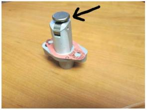
5. Install gasket onto tensioner. MAKE SURE THE TENSIONER CYLINDER IS PUSHED ALL THE WAY INTO THE BODY OF THE TENSIONER.
