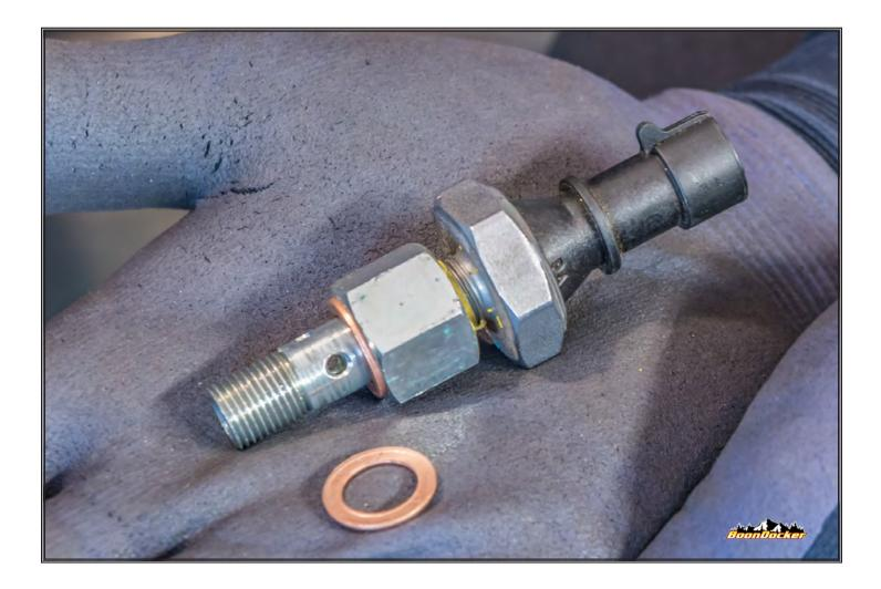
Install provided copper washers on the oil feed-line fitting.
