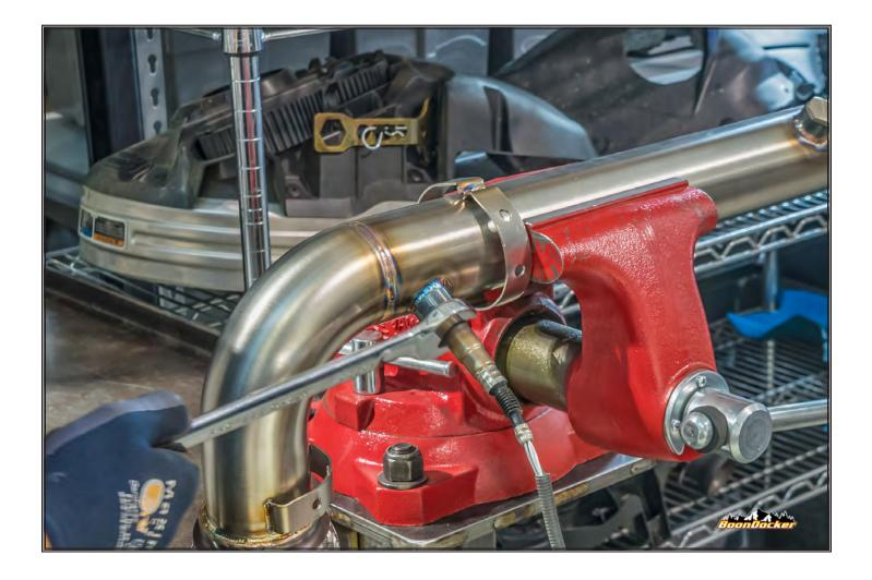
Remove OEM O2 sensor from old down-pipe and install on the provided new down-pipe.
