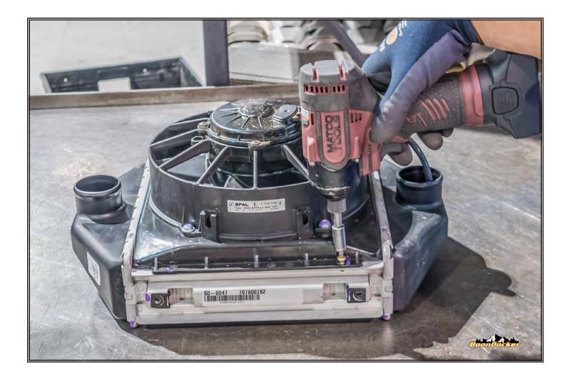
Unfasten screws holding fan to intercooler. Set the fan aside for later use. The intercooler core will not be used again.
