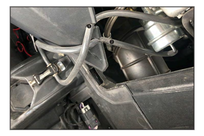
Properly connect the boost-Tee to the wastegate. Pay attention to the orientation arrows on the boost-Tee. Connect line 1 to the boost reference fitting on the turbo fitting. Connect line 2 to the wastegate actuator as shown. Reinstall turbo-access panel. Verify that the hoses aren't kinked.
