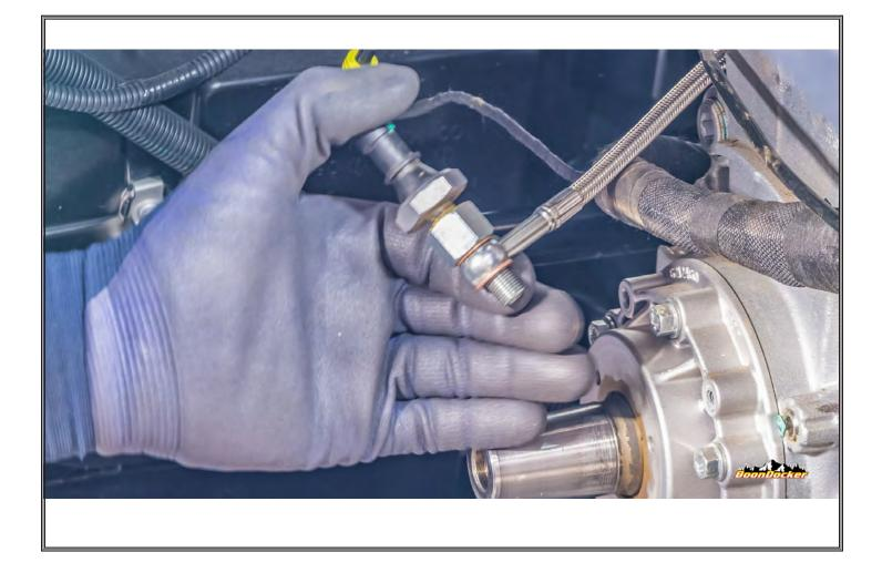
Install oil feed-line onto oil-feed fitting using the provided copper washers, as shown, and re-install into the PTO-side of the engine.
