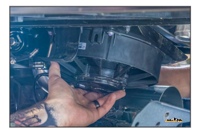
Place intercooler on top of fan, and fasten fan to intercooler
