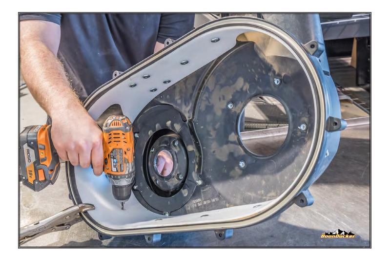
Place liner into clutch cover and drill out corresponding holes in liner then rivet liner in place.
