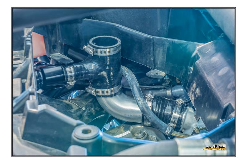
Install Charge tube and provided silicone Tee as shown (BOV is installed in a future step).
