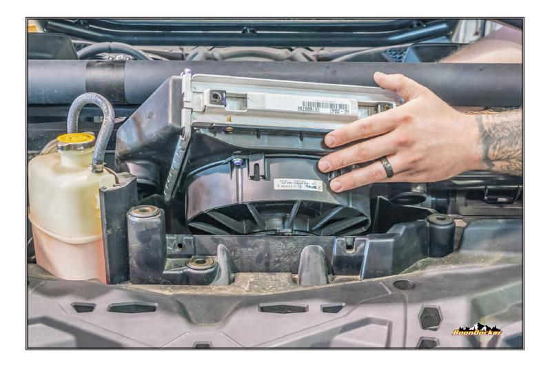
Pull intercooler assembly (intercooler & fan) out of car
