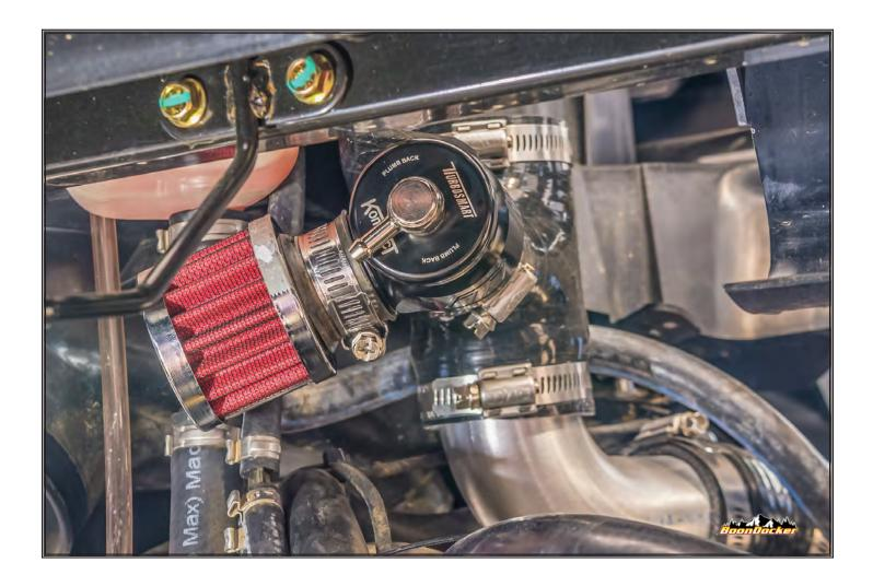
Place blow-off valve as shown. Tighten hose clamps.
