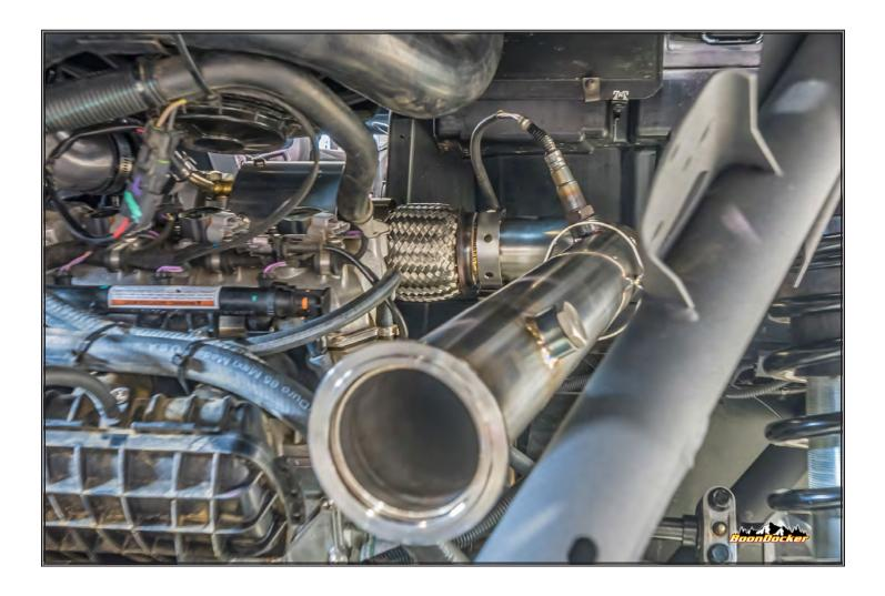
Roughly align down-pipe in a horizontal fashion so that you can attach heat-shielding.
