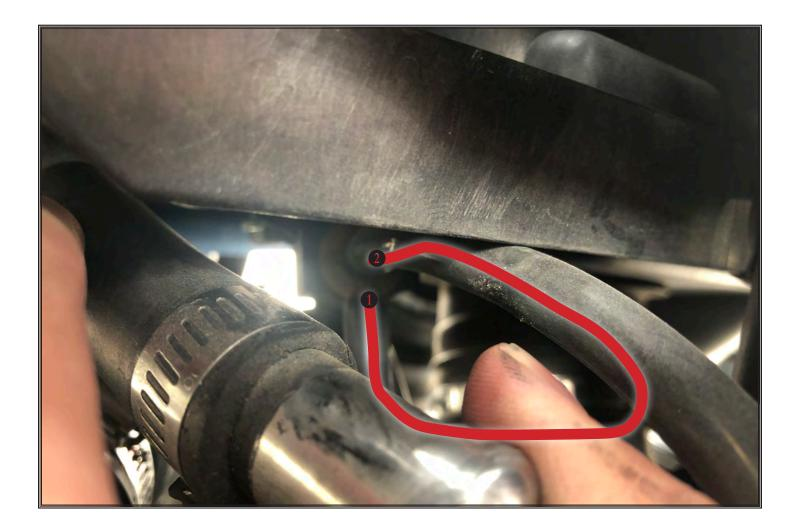
Loop the boost reference line from the boost solenoid back to itself (1 to 2) to prevent the solenoid from getting dirt or debris inside it. The boost solenoid is no longer used with this kit, and has been replaced with the manual boost Tee. For reference, one barb on the boost solenoid will return to the cold-air box, and the other two barbs will be connected to
