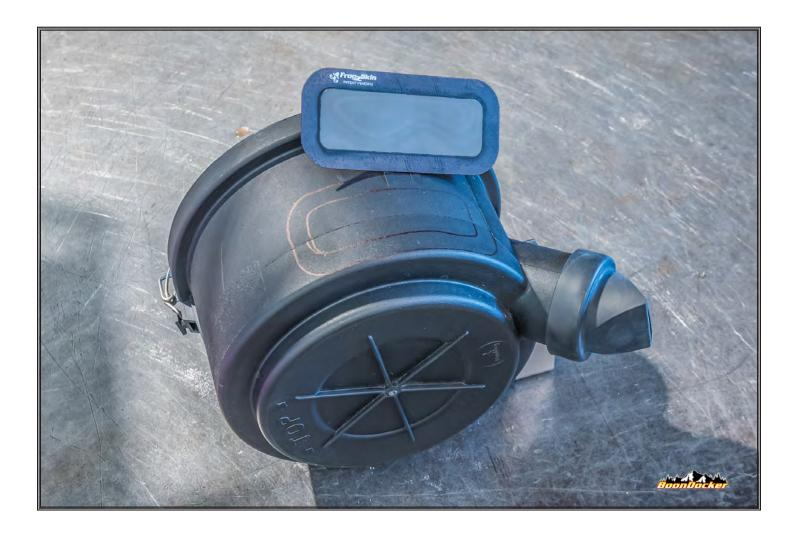
Trace the three provided Frogskins evenly spaced around the airbox. Don't worry about placement, other than making sure all three "fit". Leave sufficient room for the adhesive edge of the Frogskins as shown.
