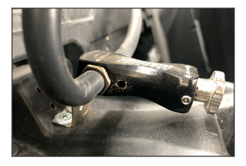
Install manual boost-Tee on top of the console, just in front of the turbo-access panel.
