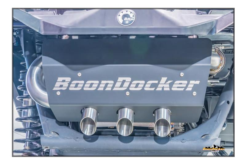
Install muffler cover. We suggest using a little bit of RTV or high-temp silicone to create a barrier between the muffler cover and the back-plate to prevent vibration noise.
