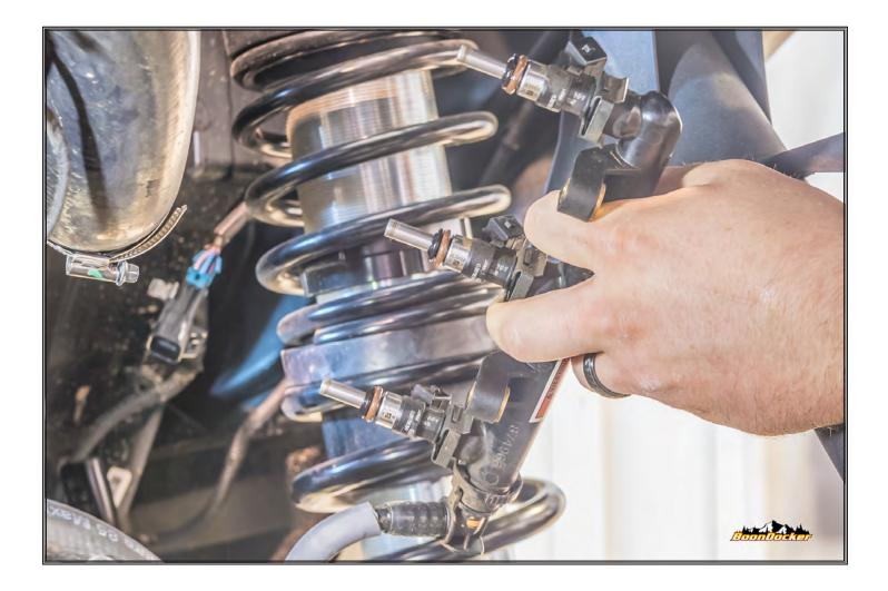
Remove hardware to allow you to remove the fuel rail with injectors.
