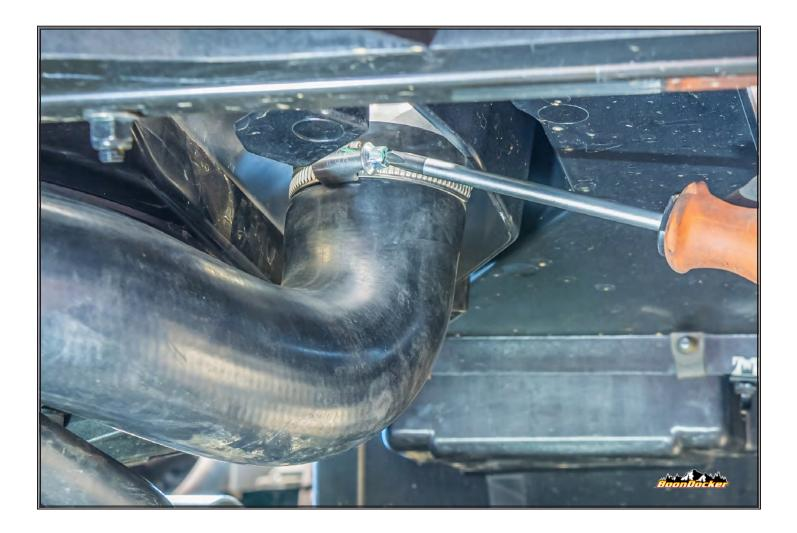
Re-fasten hoses to intercooler. Secure with hose clamps.
