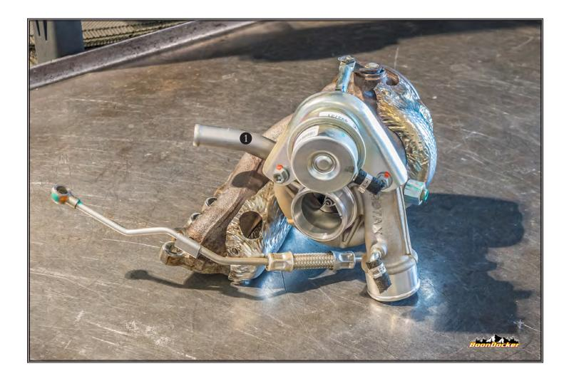
Remove oil drain line ① from OEM turbo and install on your new BoonDocker Dominator turbo.
