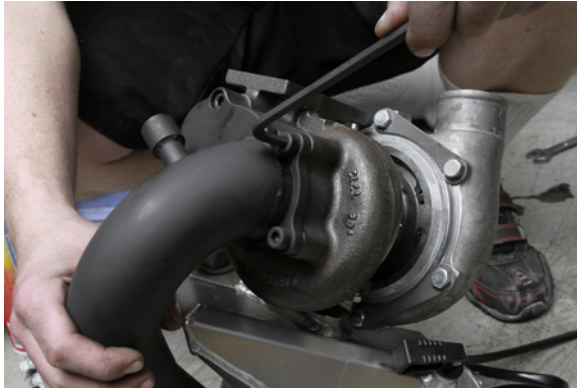
25. Bolt the turbo exhaust outlet to the turbo housing.
