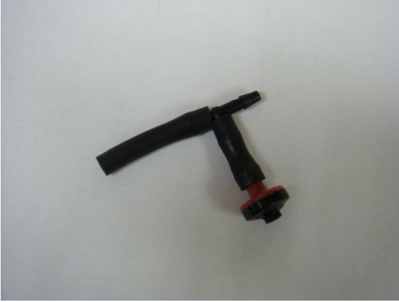
1. Red and Black check valve assembly with 3/16" plastic vacuum T and hose.
