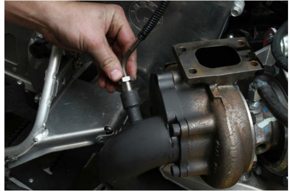
28. Install the stock probe into the exhaust outlet.
