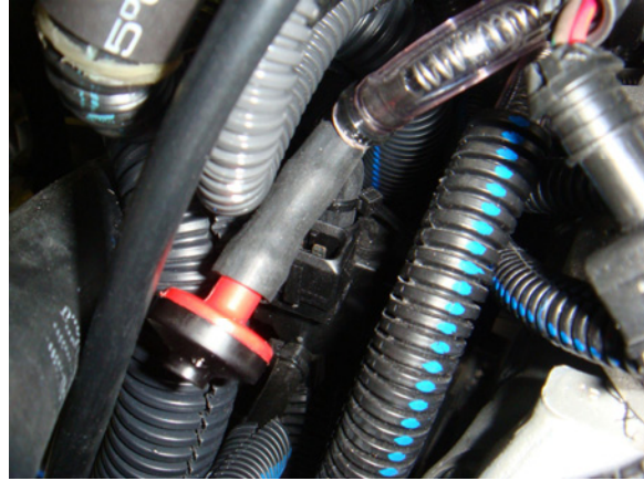
2. Install red and black check valve assembly to the metal (chrome) port on the RAVE valve solenoid, and reconnect the clear RAVE valve hose to the red and black check valve assembly.
