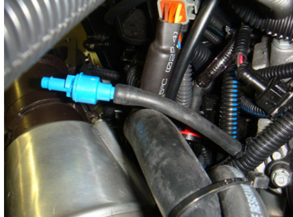
4. Cut the hose to the RAVE valves before RAVE valves, install blue check valve assembly into RAVE valve hose . Do not do not connect anything to open end of the blue check valve.
