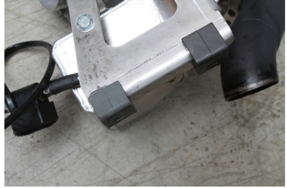
26. Install the rubber bumpers from the original silencer on to the turbo assembly. Check that the other stock silencer rubber mount is attached to the chassis.
