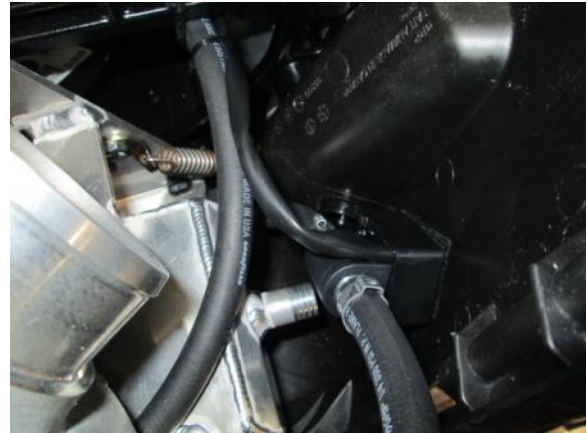
34. Route the outside turbo coolant hose under the bulk head cross member to coolant bottle. Clean the belly pan & attach oil pump Velcro. Heat the glue on the Velcro for best adhesion.
