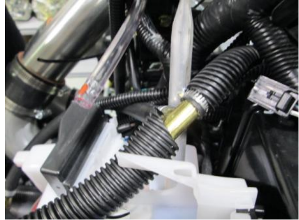
20. Cut and splice into the return fuel line, install T into fuel and tighten clamps. Position for clearance, zip tie & secure.
