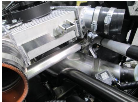
24. Install intercooler using 2- hose clamps on cross bar, do not tighten, install fan route power to adapter harness , install 90 degree boost fitting in to inner cooler tank
