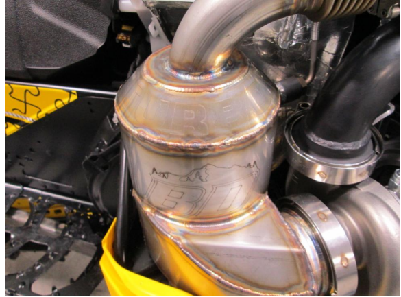
44. Install Tial muffler. NOTE when installing the muffler rotate the top of the can to the inside of the snow machine for a equal clearance to both the side panel, chain case & stock oil tank.
