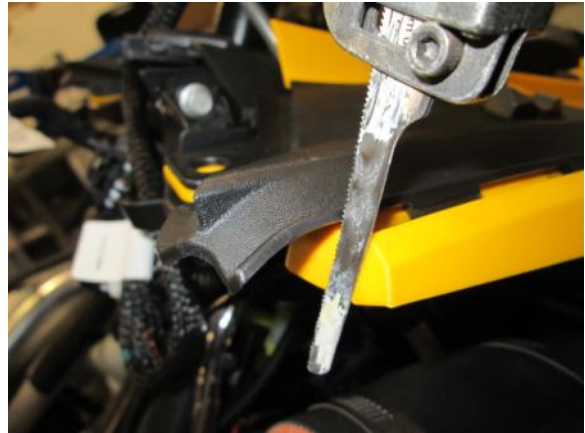
46. Cut the shroud just enough to run control box wiring & boost reference line through this area. Zip tie wires as needed to hold wires & boost line.
