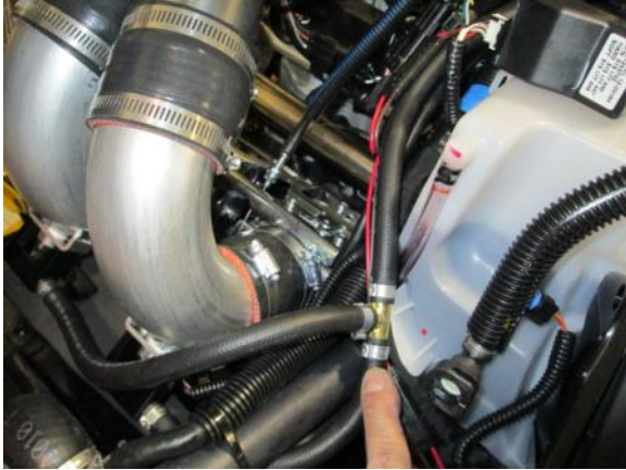
19. Zip tie fuel lines so they do not kink & zip tie the wire harnesses securely.
