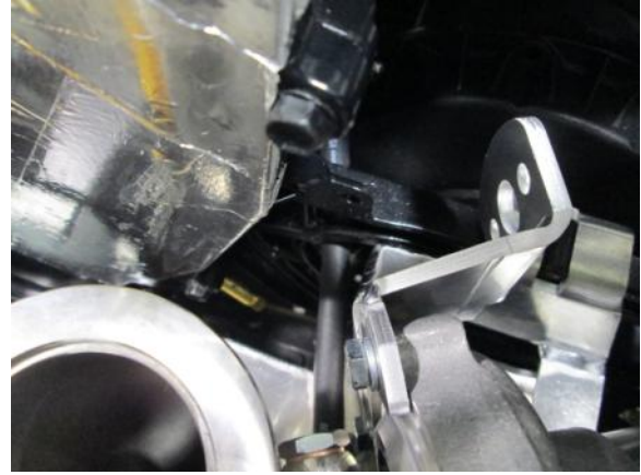
32. Route the inside coolant line under the bulk head bracket as seen. Route up to the back side of coolant bottle.
