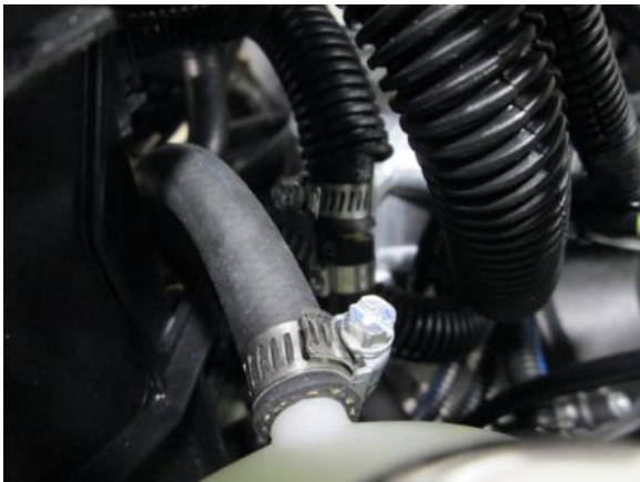
35. Route & hook up power for oil pump to power harness. Route coolant hose to coolant bottle. Zip tie the hose & power harness away from any hazard. Tighten coolant hose clamps.
