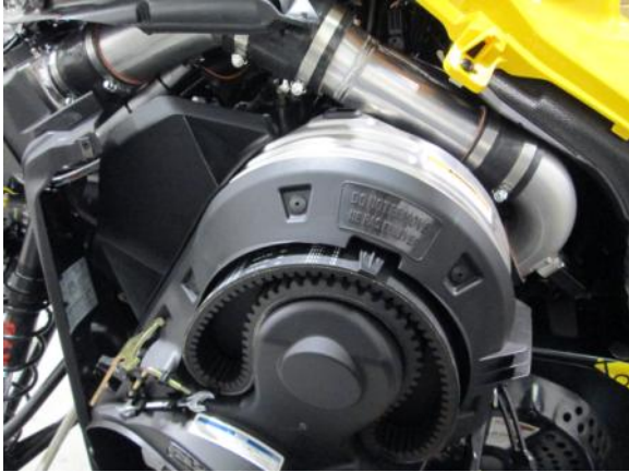
43. Check for clearance on the clutch cover & on the head light to 3" charge tube. Tighten all air box & charge tube hose clamps.
