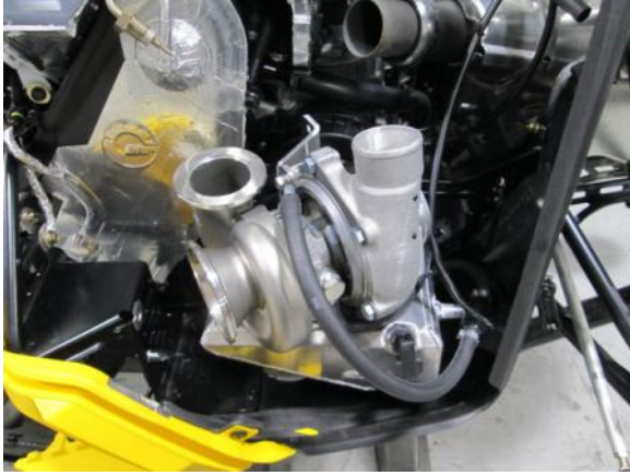
31. Install the turbo assembly as seen in the picture. Install the spring supplied for turbo bracket tab to bulk head spring tab.
