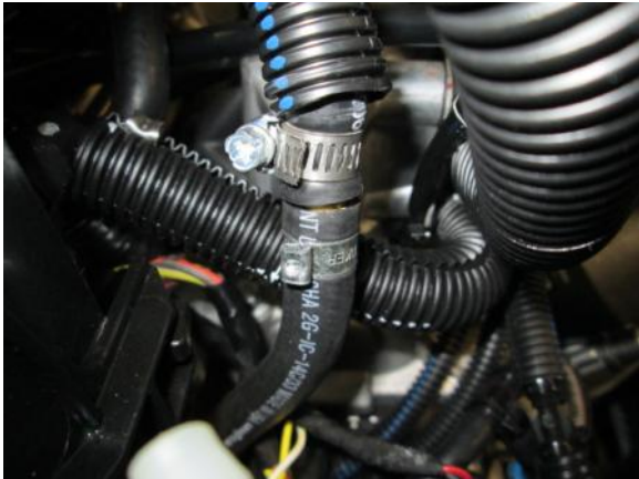
33. Remove the small coolant line from the back of the coolant bottle. Then route to the coolant hose you just removed. Make sure you secure hose so it won't chaff wires or hose.
