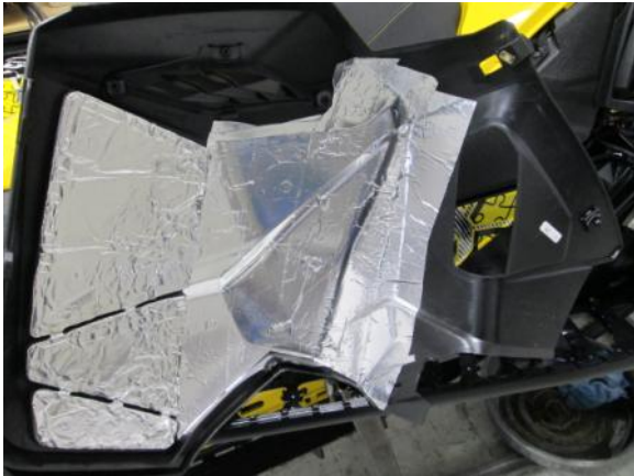
45. Cut & remove the stock heat tape/insulation from the side panel & install the heat tape as seen in the picture.
