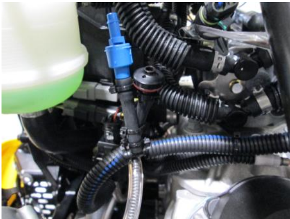
23. Cut hose between rave valve & solenoid. Install the check valve inline Turn the check valve down & zip tie lines on. Make sure routing of hoses have good clearance.
