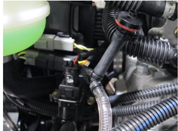
22. Remove the clear line on rave valve solenoid & Install check valve. Turn the blow off to down position. Zip tie the hoses on.
