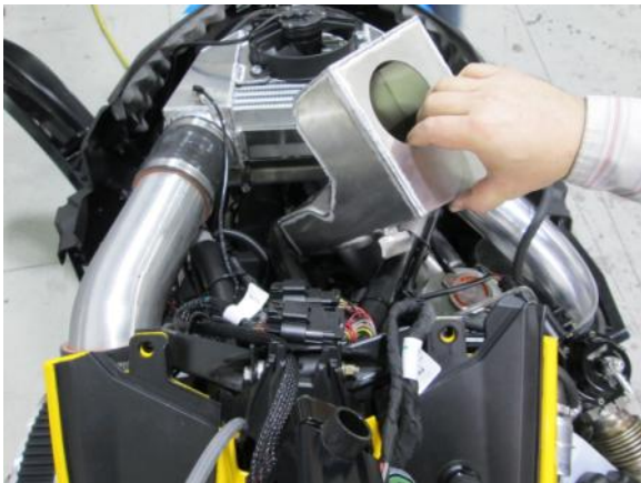
47. Turn handle bars all the way to the left & install the cold air intake as seen in picture to fit.
