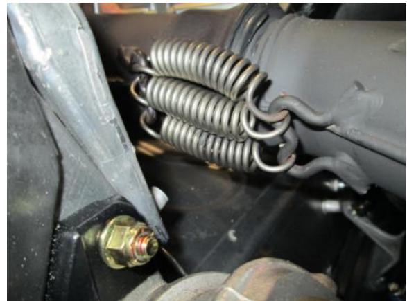
36. Remove the pipe off of the doughnut apply high temp silicone on both sides of the doughnut & reinstall pipe. Triple up the springs on the pipe as seen in the picture.
