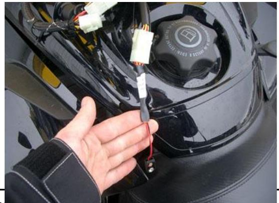
Jumper connector - the injectors are now connected directly to the sled's ECU.
