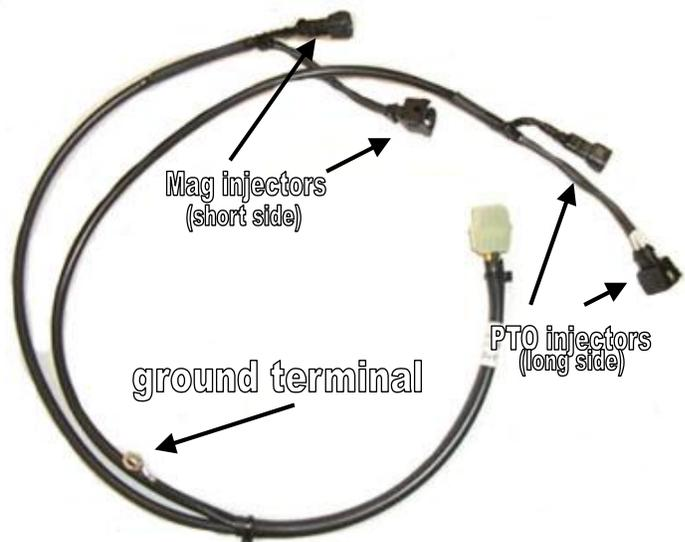
2. Plug each EFI Control Box harness fuel injector connector (female) on to the fuel injector. The connector with tan wire and two red wires coming out of the female housing plugs on to the fuel injector on the MAG side (shorter side on harness).
