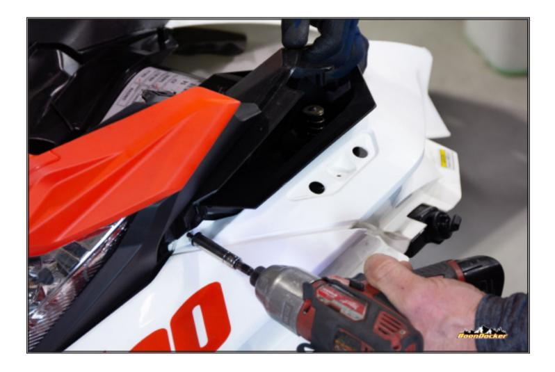
Remove vents and remove hidden screw underneath vents.
