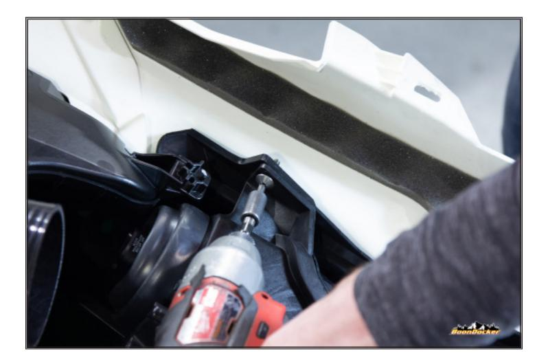
Remove black threaded clips from intake plenum and re-install inner headlight bolts using clip.
