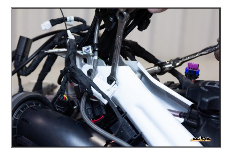
Remove upper gas tank shroud bolts.
