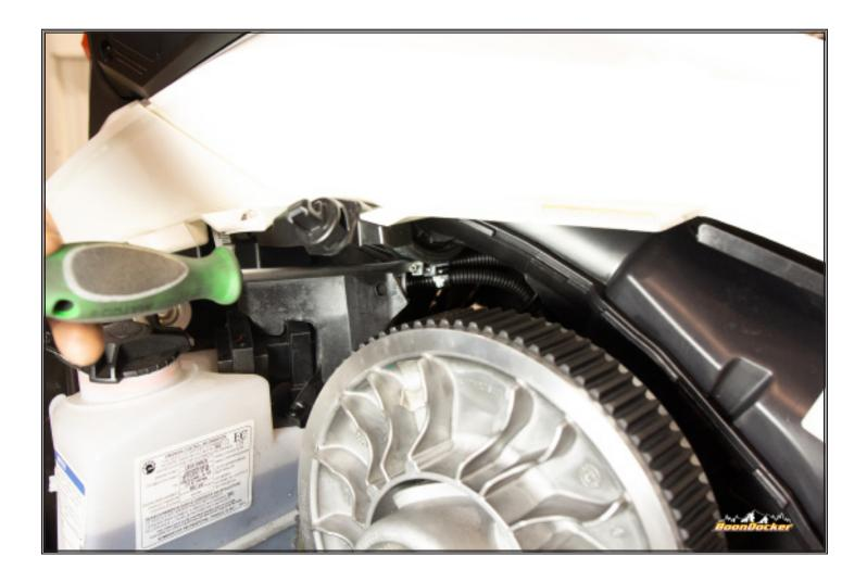
Loosen clamp from airbox to hood.
