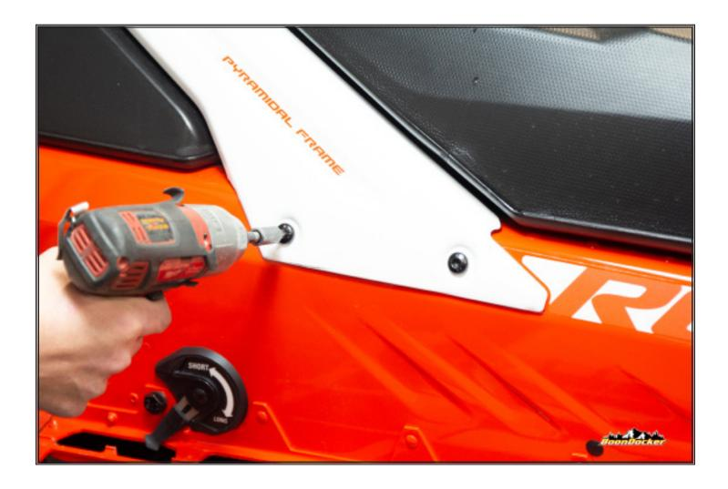
Remove black torques head bolts from bottom of gas tank shroud.
