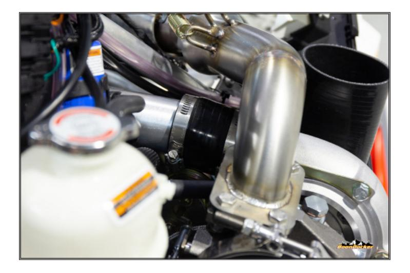
Install charge tube to turbo using supplied silicone and hose clamps.
