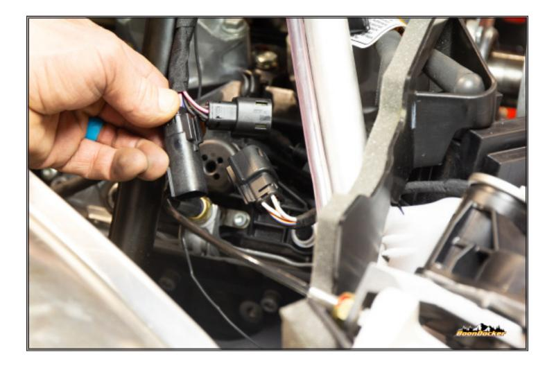
Unplug coil pack and plug BoonDocker harness into both connections.
