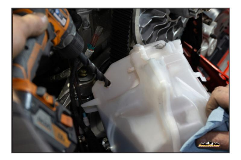
Drill 1/2" hole on rib close to bottom of oil tank.
