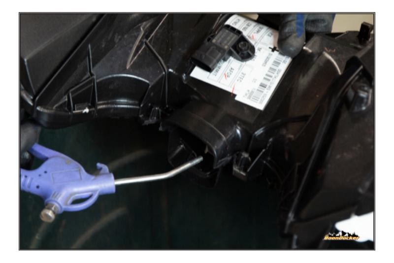
Blow air intake box out ensuring no debris is in the box
