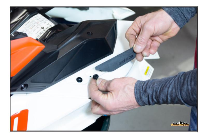
Remove Ski-Doo plastic protector and remove screw underneath.
