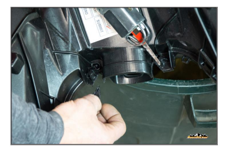
Cut corner pieces off of intake delivery tube allowing the silicone boot to slip on
