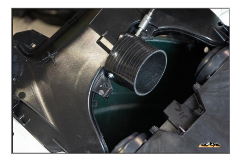
Install silcone with provided 3 self tapping screws and washers.
