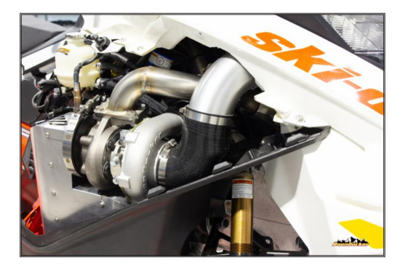
Install cold air intake tube to silicone 90.
