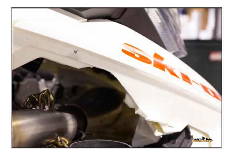
Trim out notch on hood to allow room for cold air intake and re-install hood.
