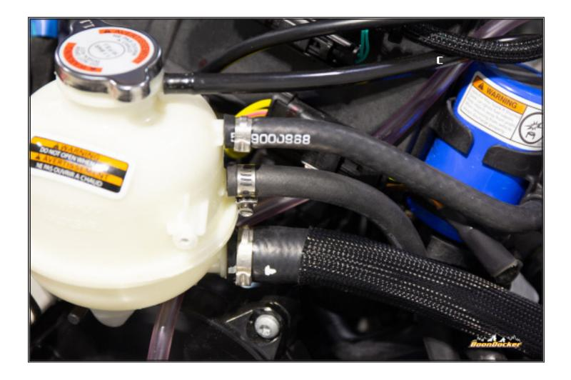
Route lower turbo coolant line to bottle and fasten with supplied hose clamp.
