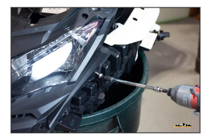
Remove 2 remaining bolts holding plenum to hood.
