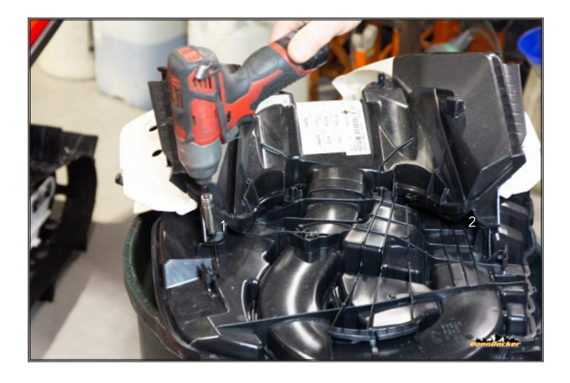
Remove 2 screws holding intake plenum to intake box.
