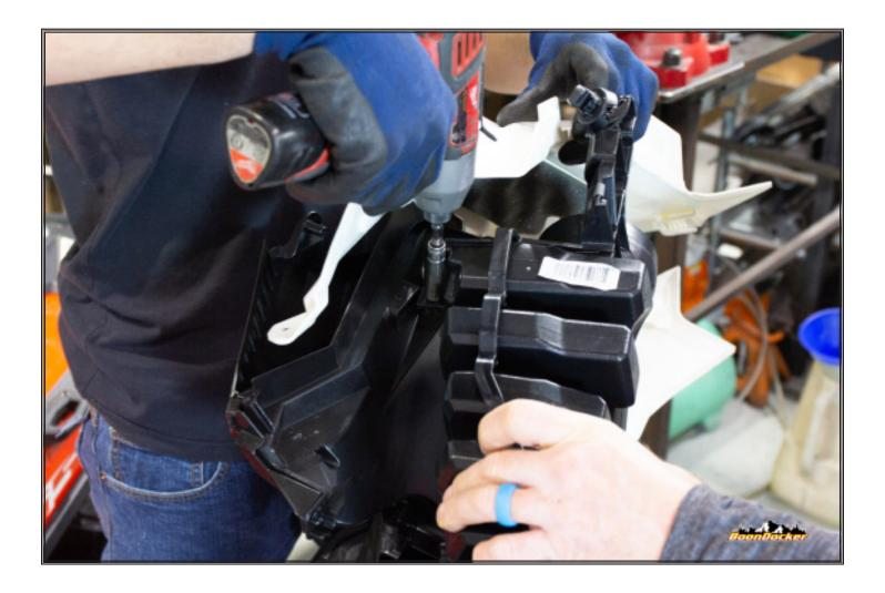
Remove hidden screws underneath intake vent holes and split both plenums.
