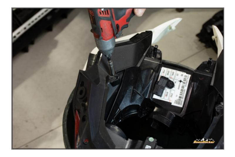
Re-install top screws holding hood to air intake box.
