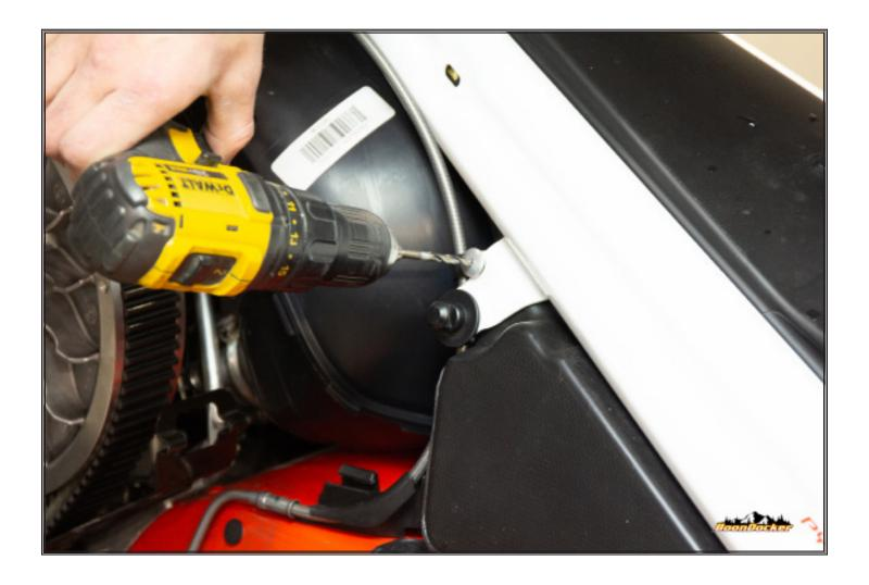
Remove rivet with 3/16" drill bit.
