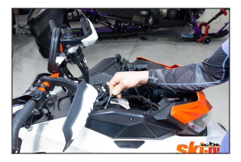
Unbolt two top screws holding hood to steering structure.
