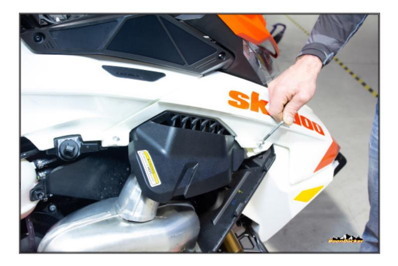
Remove two screws holding hood to main chassis.
