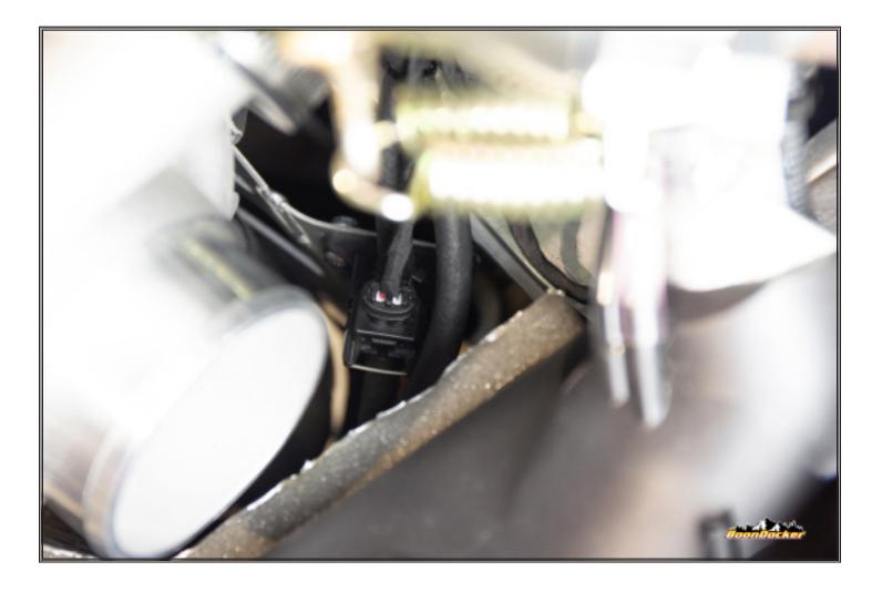
Plug control box wire harness into solenoid.
