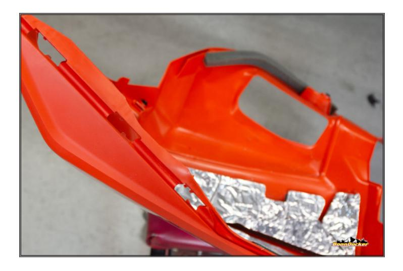
Trim side panel to allow clearance for silicone 90 on turbo.
