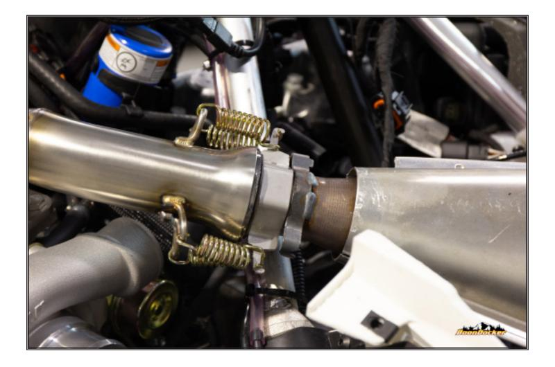
Install the spring tab re-enforcement kit to pipe and spring to inlet with supplied short gold springs.
