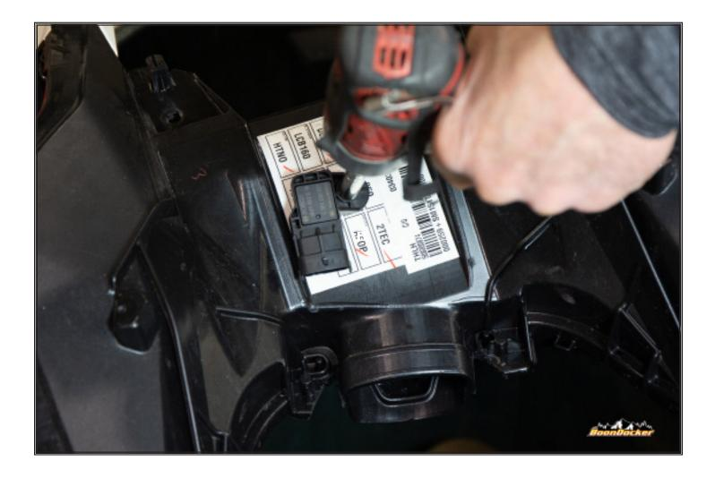
Install factory T-BAP sensor into 1/2" hole.
