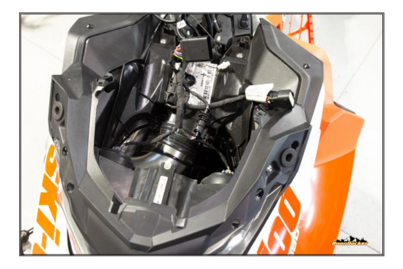
Attach cold air intake to hood with provided hose clamp and plug BoonDocker control box into factory T-BAP sensor and factory wire harness.
