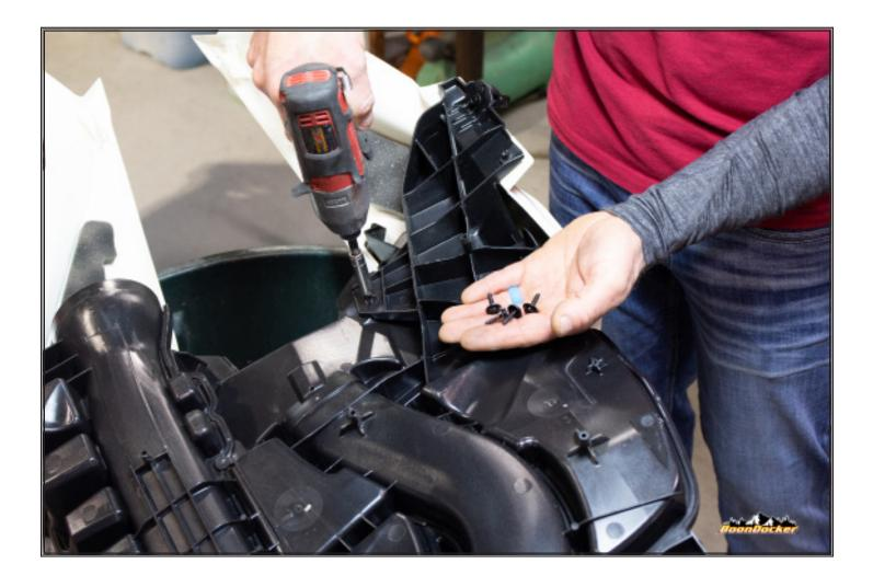
Remove all screws from intake plenum holding it to hood.
