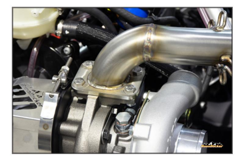
Install inlet with supplied gasket and hex bolts.
