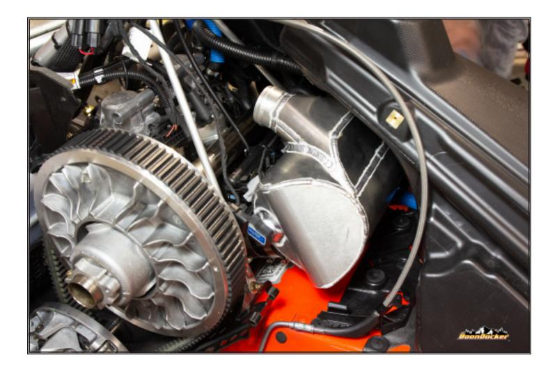
Install airbox and plug wire harness into boost sensor on airbox.
