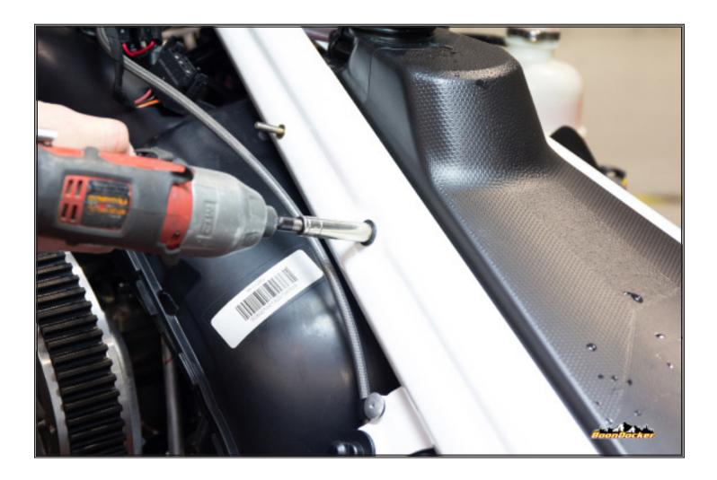
Remove center tank shroud bolt.
