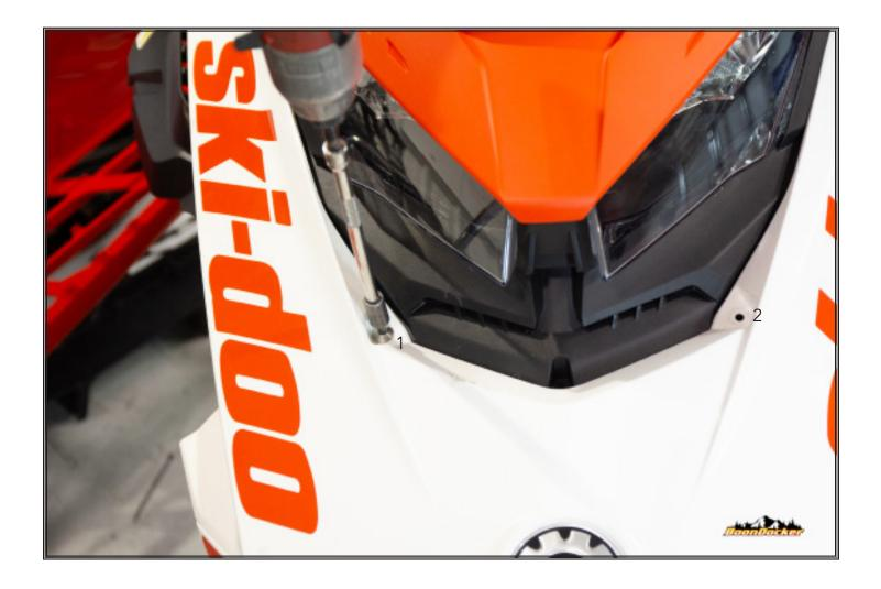
Remove two front hood bolts and nuts.
