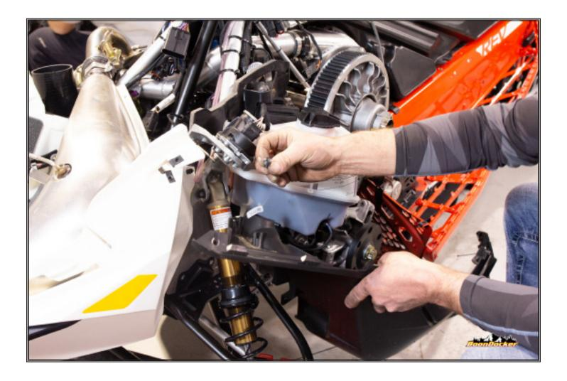
Unscrew and remove clutch side belly pan from vehicle.
