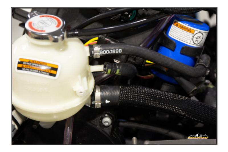
Cut clamp and remove coolant line from bottle.
