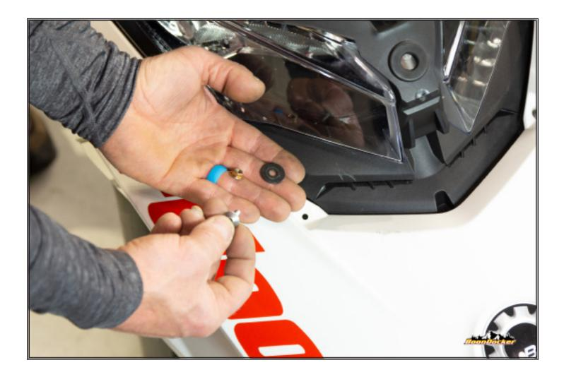
Re-install front hood shroud with factory bolts, washers and nuts .
