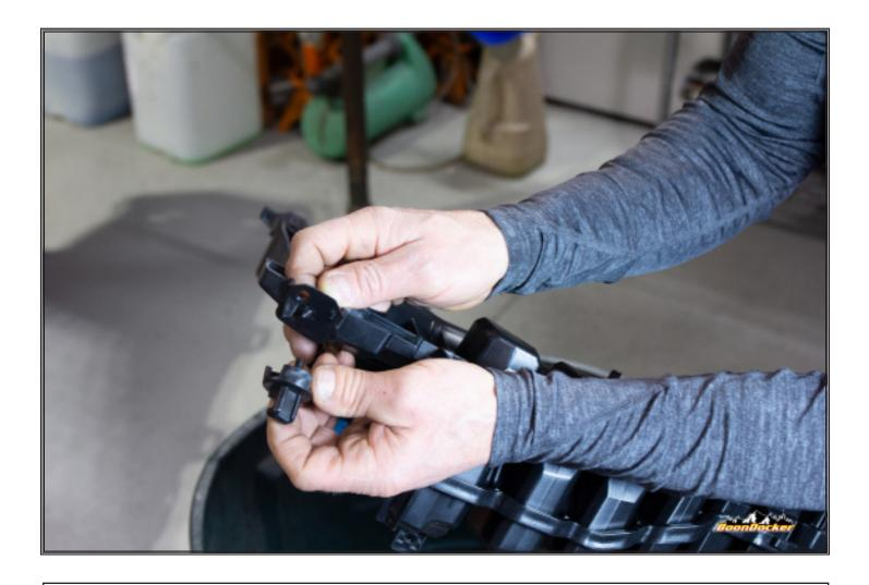
Remove plastic locking tabs from intake plenum.
