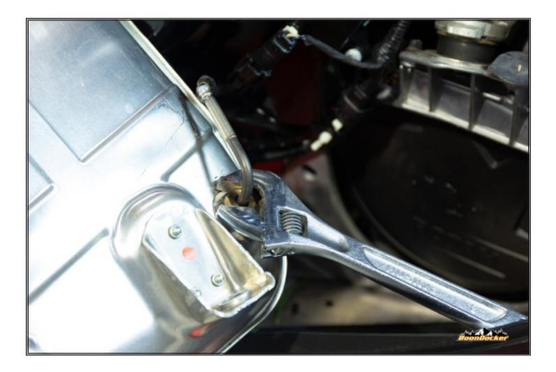
Remove exhaust temp sensor from muffler.
