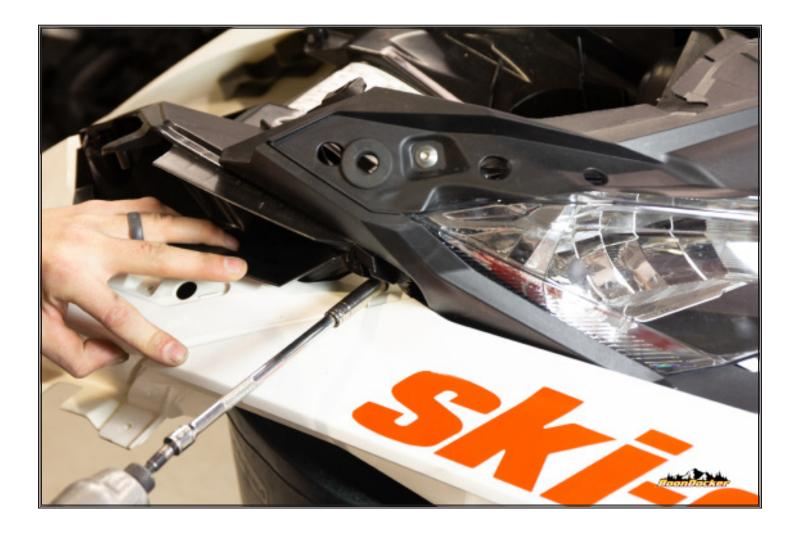
Re-install hidden bolt under intake vents.
