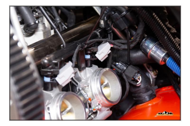
Plug BoonDocker injector wires into injectors ensuring yellow wire goes to MAG and green wire goes to PTO.
