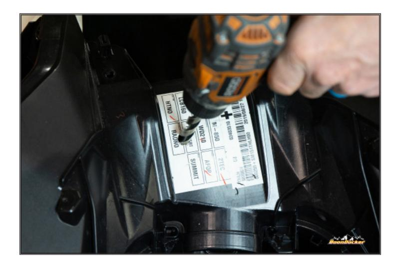
Drill 1/2" hole into intake airbox.
