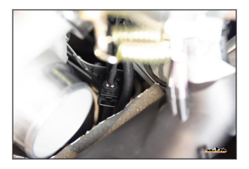
Plug control box wire harness into solenoid.
