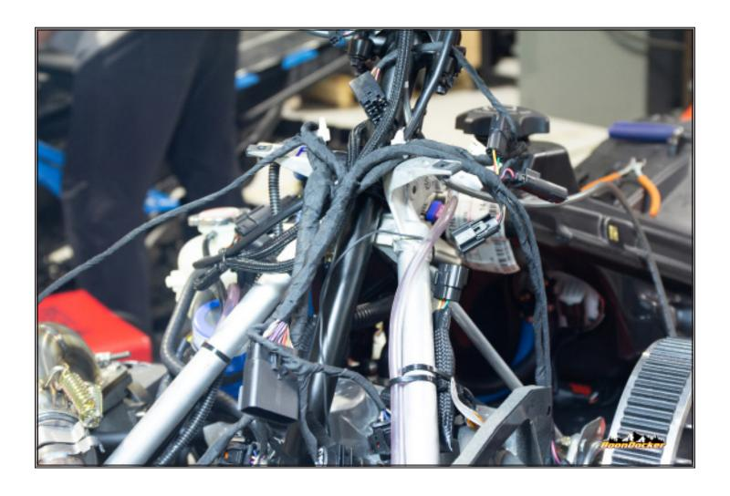
Lay control box harness over steering structure routing solenoid, oil pump, injectors down turbo side of sled and routing coil pack wires and T-BAP wire down clutch side of sled.
