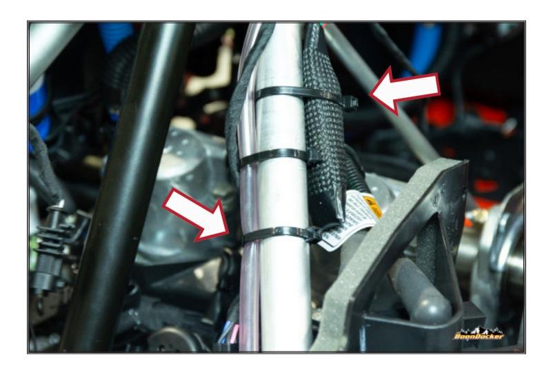
Zip tie wire harness and resistor as shown.
