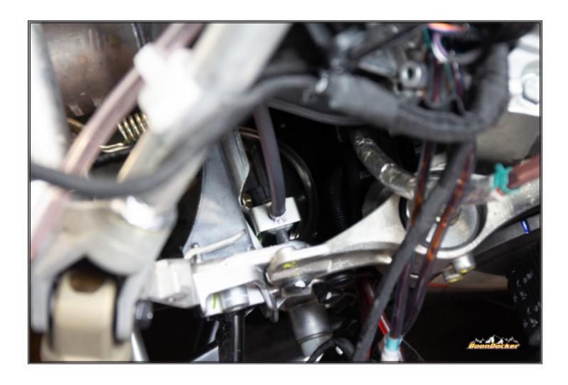
Route control box wire harness following clear oil underneath Y-Pipe to auxillary oil pump and plug in.
