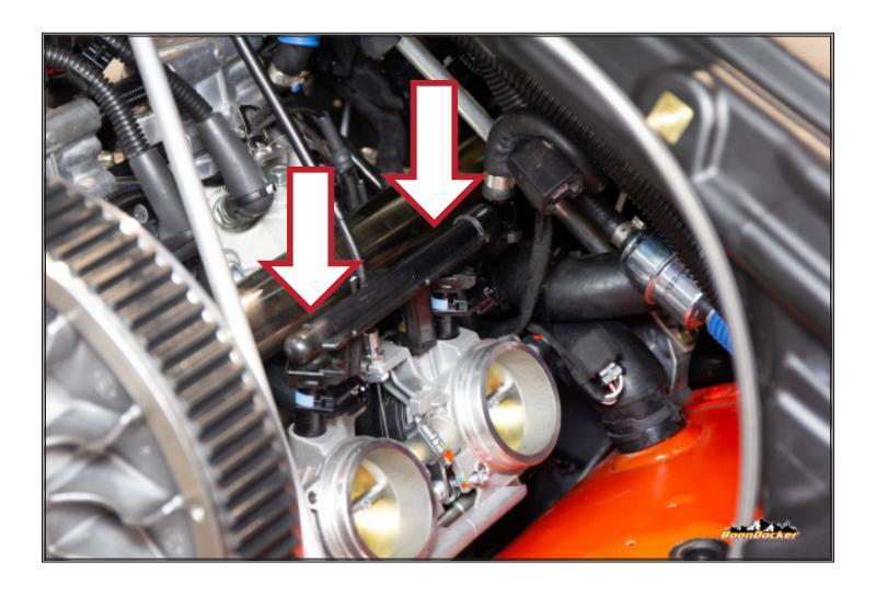
Unplug factory injector harness from injectors.
