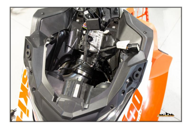
Plug BoonDocker control box into factory T-BAP sensor and factory wire harness.
