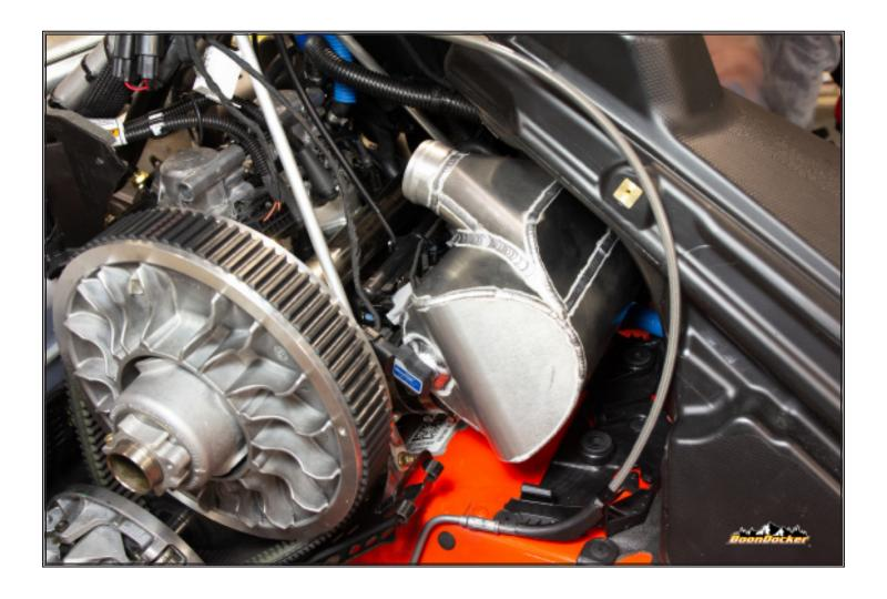
Plug control box wire harness into boost sensor on airbox.
