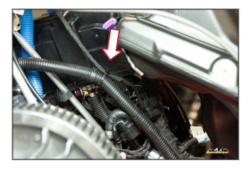
Plug BoonDocker green wire harness into factory injector wire and zip tie as shown.
