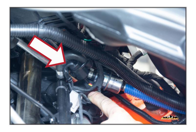
Plug yellow wire harness into factory MAG side injector wire harness and zip tie as shown.
