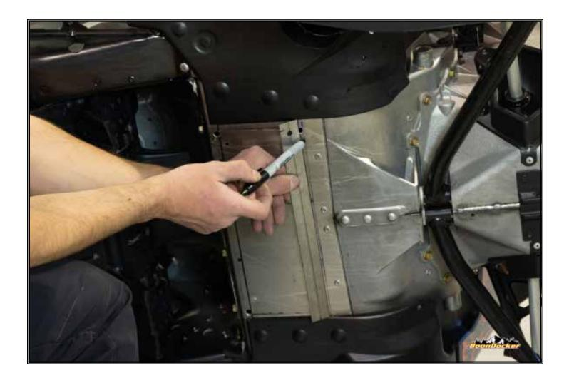
Measuring from rar of belly pan, sharp edge, next to the track mark 1" and 5" in multiple spots, then use a straight edge to complete lines. Measure 3/8" from the cut outs on either side of the sled and use a straight edge to finsih marking the cut out for the cooler.
