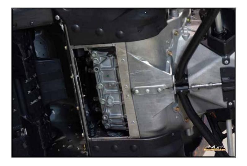
Clean up edges with a deburring tool and prepare to install the cooler. Take radiator and place in reshly cut hole and mark mounting holes to be drilled out.
