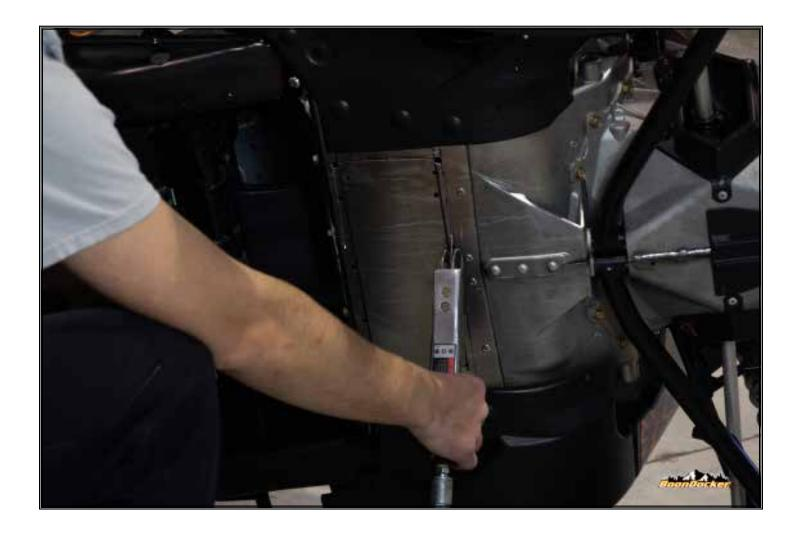
Using an air saw, or preferred cutting method, cut out the marked area staying inside the lines. Make sure you don't cut too deep into engine bay to avoid dammage. We used a very short blade to do this.
