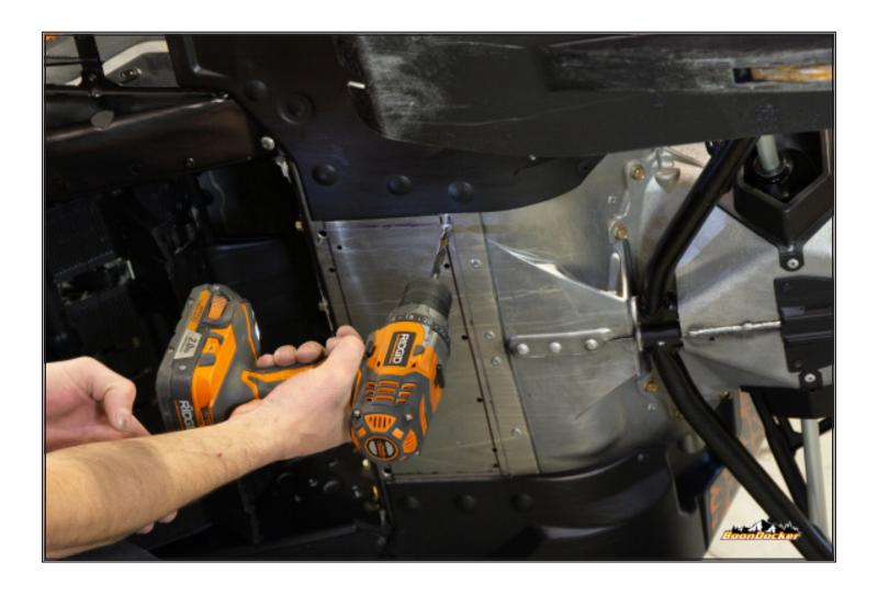
Using s 3/8" drill bit make holes in corners of marks to commadate air saw blade. Be sure to stay INSIDE your marks.
