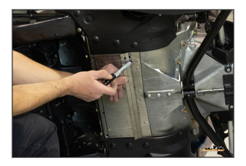
According to supplied instructions mark and measure out the intercooler cut-out.
