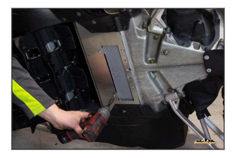
Loosely install small self threading screws and loosen 3 previously installed self threading screws.
