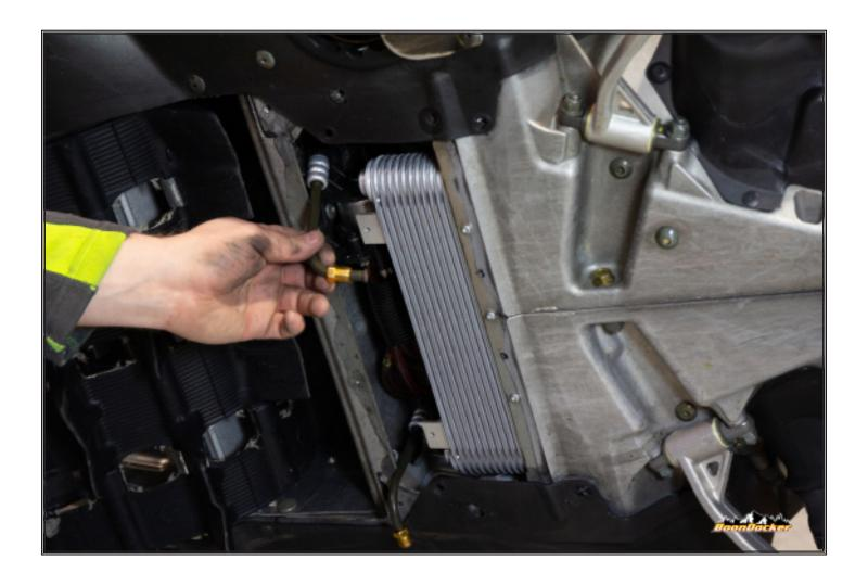
Route MAG side coolant line towards factory coolant line.
