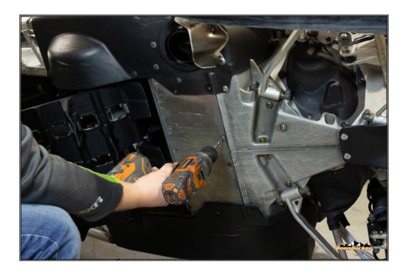
Remove the 8 small head rivets holding belly pan to chassis and 5 large rivet heads that hold plastic to belly pan.
