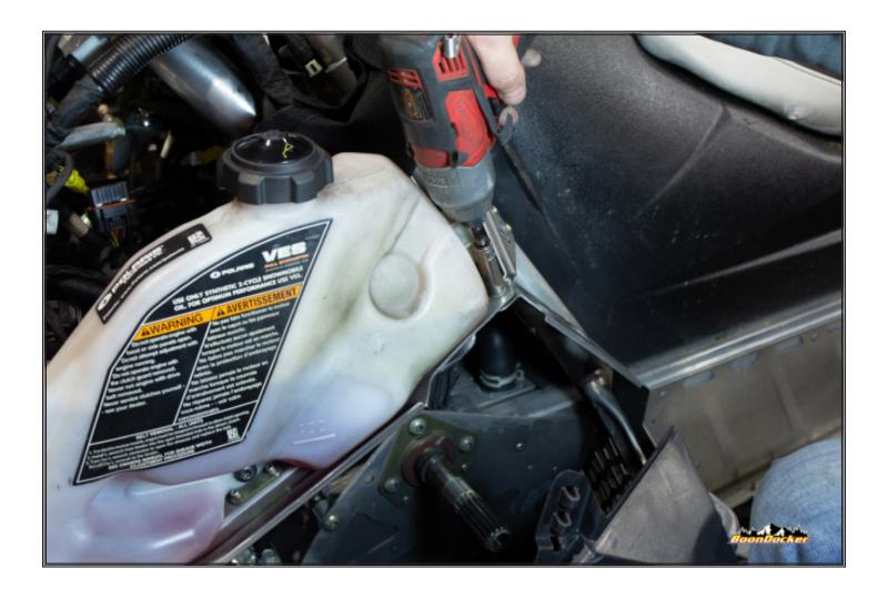
Re-install oil tank plate.
