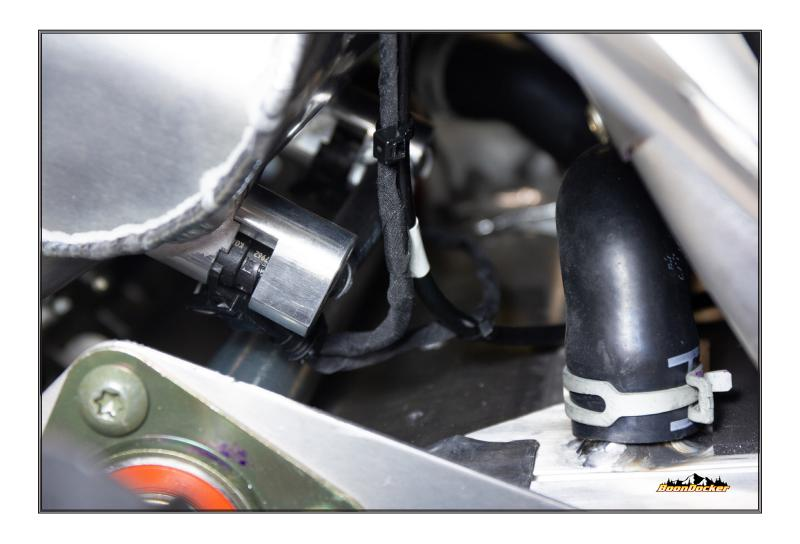
Plug auxillary fuel injector harness into fuel injectors and zip tie as shown.
