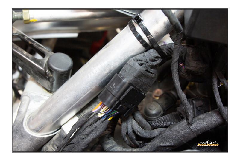
Connect the stock ECU plug into the fuel controller, and zip tie as shown.
