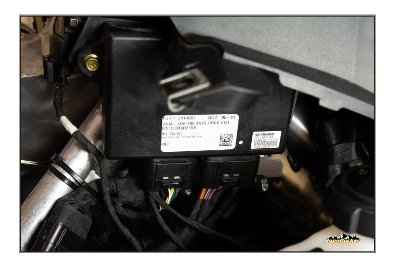
Plug the BoonDocker Fuel Controller directly into the ECU and velcro controller to the ECU.
