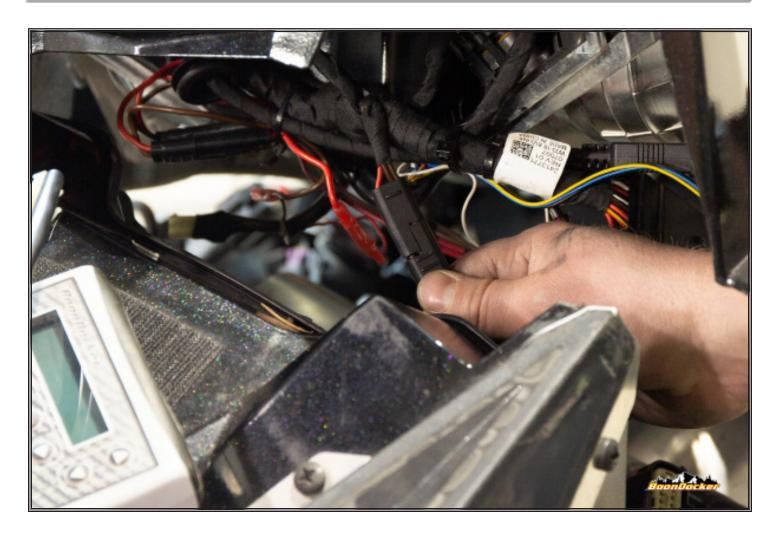
Re-install cold air plenum and hood. Route coolant pump wiring harness to factory ACC power on hood.
