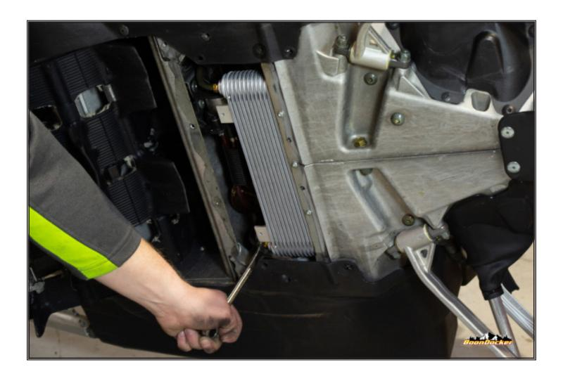
Ensure lines are routed so they are not rubbing against any sharp edges and tighten fittings.
