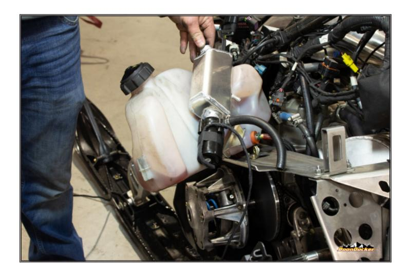
Place coolant bottle on oii tank as shown.
