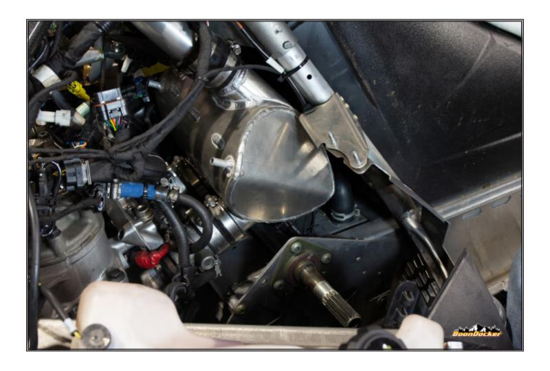
install water to air airbox to throttle bodies and charge tube. Ensure injectors are plugged in and all clamps are fastened tightly.
