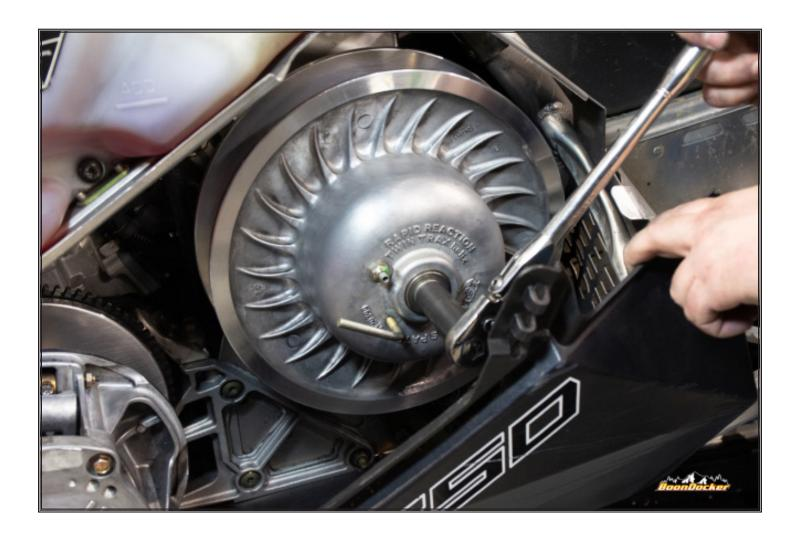
Re-install secondary clutch.
