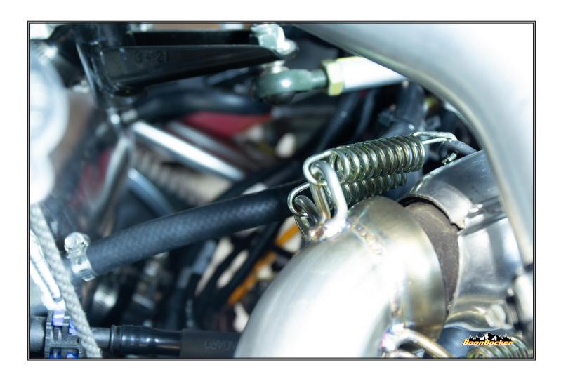
Route coolant line over engine following factory coolant hose to MAG side of airbox.
