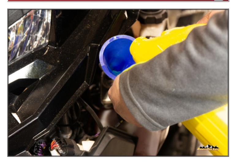
Fill coolant botle and start sled, continue to fill coolant bottle until coolant level is at bottom of threads, leave space to prevent leaking during pressurization.
