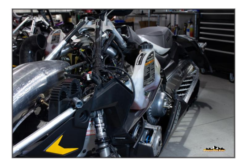
Remove side panels, hood and cold air plenum.
