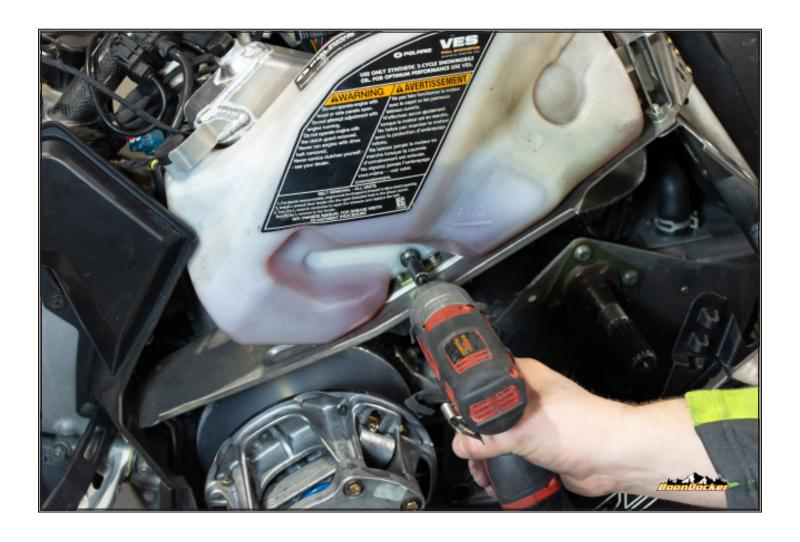
Install coolant and oil tank using factory bolt
