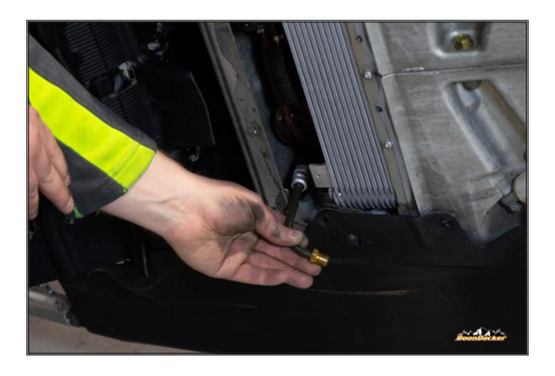
Route PTO side coolant line following factory oil line.
