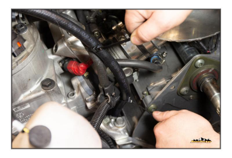
Route PTO coolant line following factory coolant line, ensuring its out of the way of all clutching.
