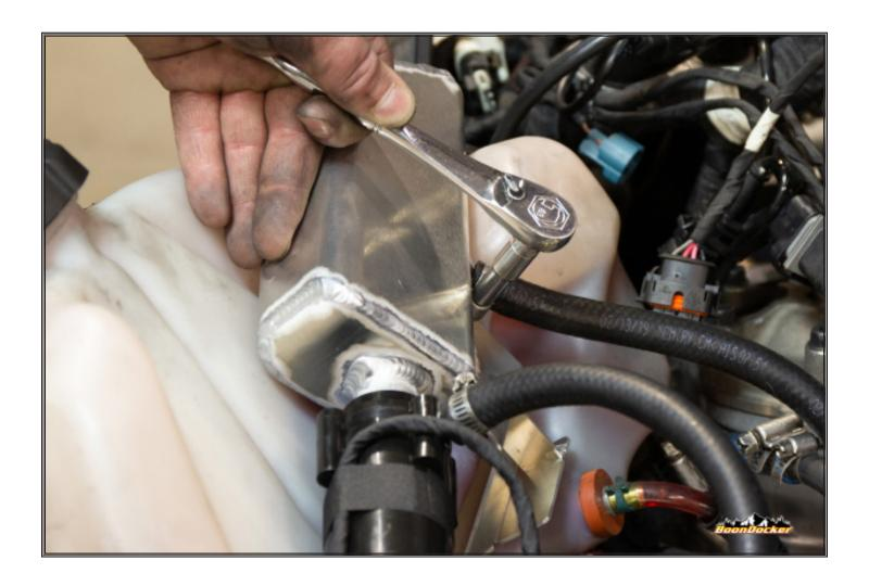
Install PTO coolant line to nipple on coolant bottle.
