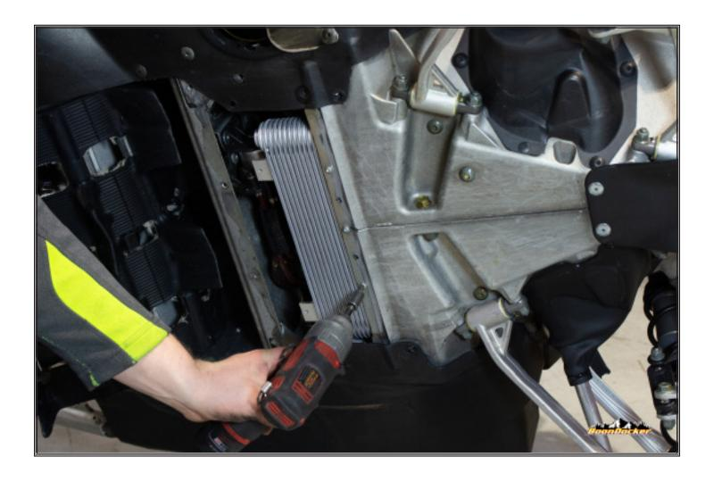
Flip intercooler and install using 3 small self-threading screws provided
