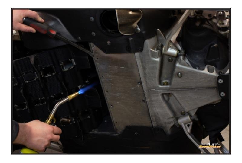
Heat plate to loosen glue and gently pry away from belly pan.
