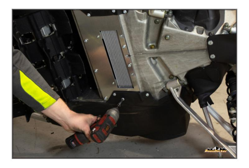
Loosely install large self threading screws.
