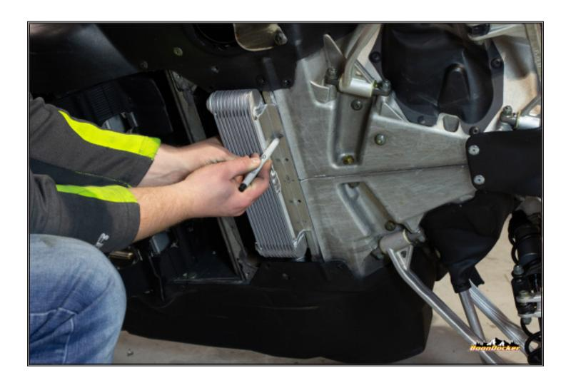
Line up 3/16" holes on intercooler core with 3/16" holes on sled and mark center of smaller holes as shown.
