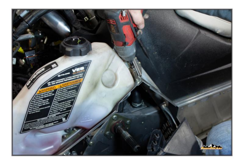
Re-install oil tank plate.
