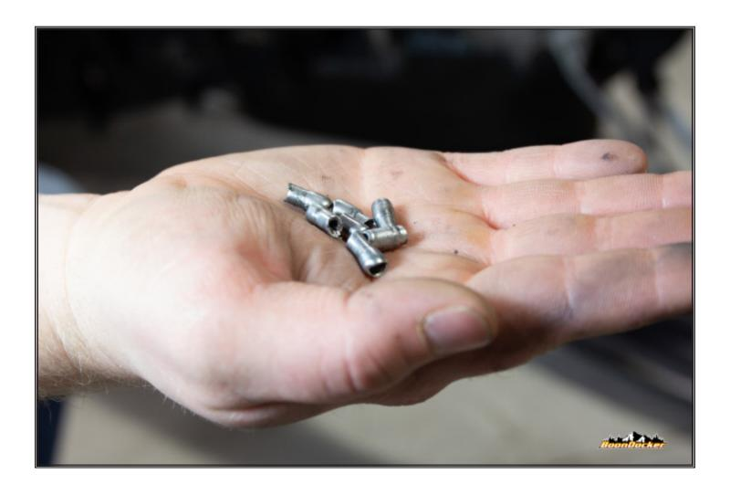
Locate and remove all rivet heads from chassis.
