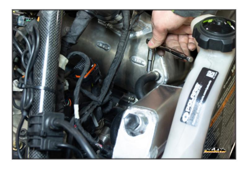
Route water tank line to PTO side of airbox and tighten hose clamp. Cut line if needed to prevent kinking.
