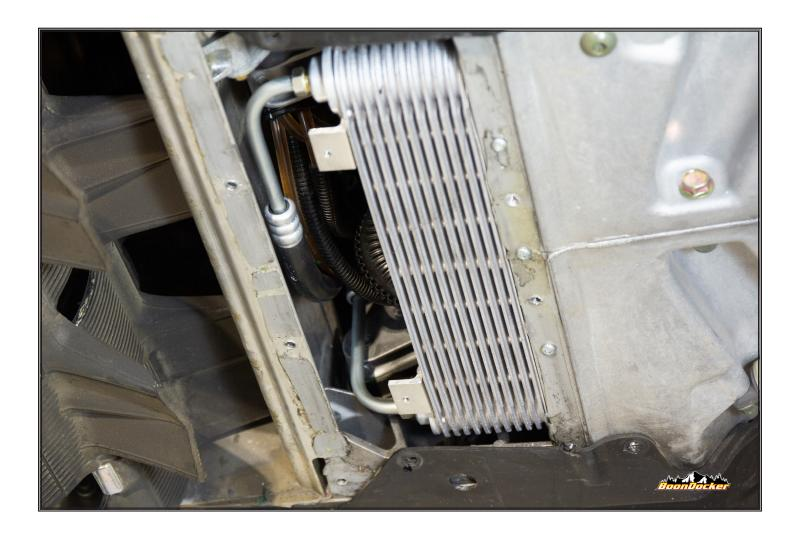
Route MAG side coolant line over to PTO side following factory oil line.
