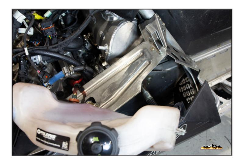
Unbolt oil tank from oil plate.
