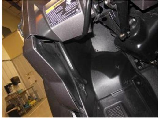
After removing side panel route wires through the hole underneath the dash behind the steering wheel.
