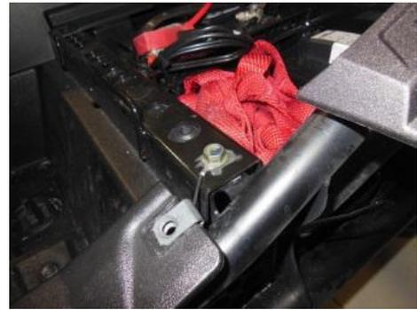
Route the harness alongside of the frame and turn in toward the clutch and follow the stock wire harness over the clutch cover to the back of the machine.
