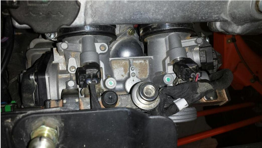
Install Boondocker box in-between factory harness and injectors. The MAG injector (on right) corresponds with the Yellow and Tan wire on the Boondocker harness. The PTO injector (on left) corresponds with the Green and Brown wire on the Boondocker harness.
