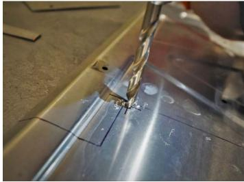
Using an air saw or similar, cut out the heat shield along the lines as shown.
