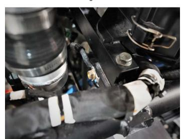
Install the 2 piece charge tube between throttle body and intercooler outlet. (Note: The V shaped aluminum tube has 2 different angles on it, the 90 degree angle faces down)
