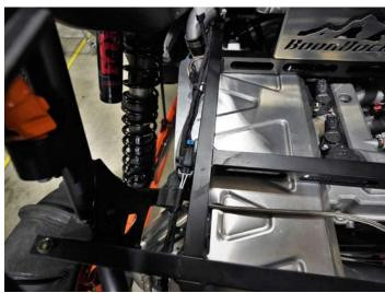
Unplug factory tail light connector on the drivers side and plug fan harness into both the tail light and the factory connector you just removed.
