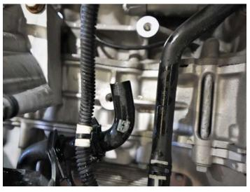
Install turbocharger coolant lines in place of the removed section. It does not matter which hose connects to each side.
