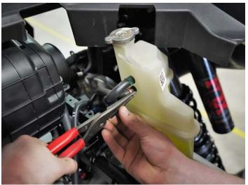
Install coolant line extension included in your turbo kit with a brass barb onto lower coolant line with red clamp and secure with provided hose clamp. Reconnect extended line to coolant bottle with provided clamp
