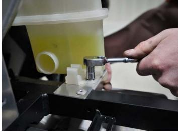
Install intercooler fan using provided allen head bolts. (Note: Wiring lays towards left side of vehicle)
