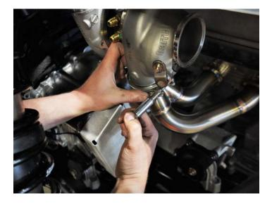
Using a square, line up the exhaust housing outlet 90 degrees from the valve cover as shown; then tighten down V-band clamp
