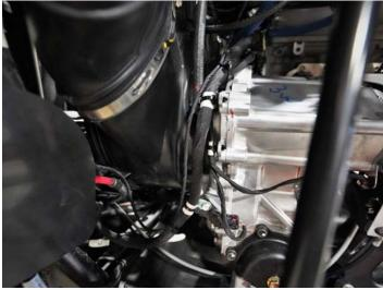
Attach positive wire from the fan harness to the upper side of the starter solenoid for 12V constant power. The negative side of the fan harness follows the factory harness across the front of the engine towards the passenger side of the vehicle to the chassis ground.
