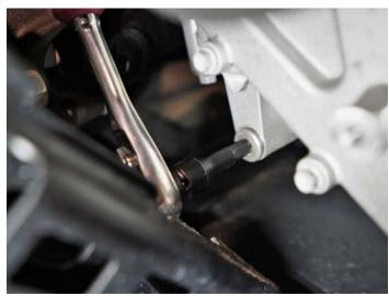
Loosely assemble oil line as shown and install into engine in place of previously removed plug.
