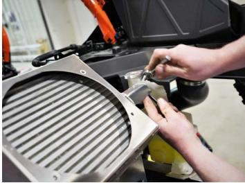
Set the lower coolant bottle bracket in place and center punch the hole into the chassis
