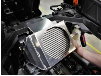
Reach behind boondocker plate and mark two additional intercooler mounting holes with a marker then remove intercooler.
