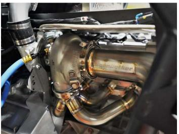
Install the second water line onto the backside of turbocharger as shown.
