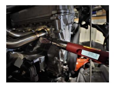
Set turbocharger in place and install V-band clamp loosely
