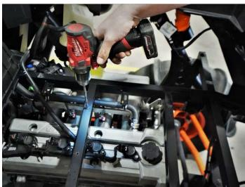
Reinstall intercooler and secure with 2 T40 Torx screws and 2 6mm bolts, nuts and washers provided with the RAGE turbo kit.
