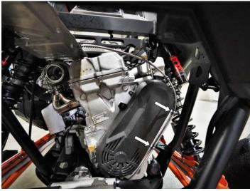
Route oil feed line up to turbo along the top edge of the heat shield. Secure with supplied darts and zip ties as shown. (¼" drill bit to install darts)
