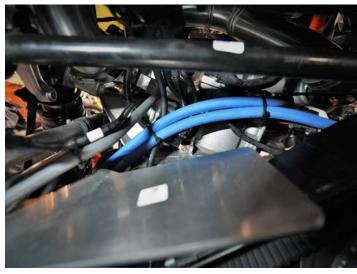
Pinch off oil cooler feed hose at both ends.
