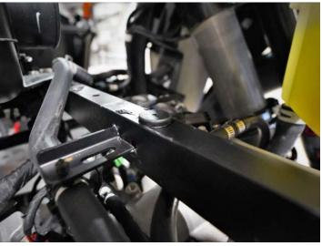
Reinstall cold air intake tube permanently and tighten clamps
