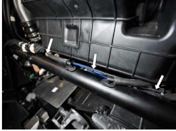
Attach ground wire to chassis ground bolt then secure harness with zip ties as necessary. Make sure to avoid sharp edges and abrasive surfaces when securing the harness.
