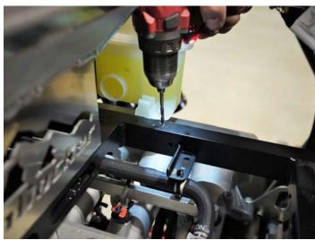
Rivet into place using supplied large head 3/16" Rivet
