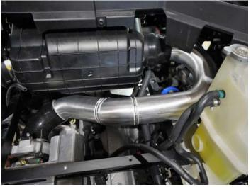
Mark the frame where the center of the cold air intake tube runs over the chassis. Remove the cold air intake tube.
