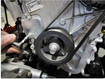
Install billet timing chain tensioner cover with oil drain installed and torque to specification 80 in-lbs
