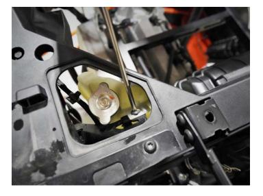
Just behind the factory coolant bottle location, measure  $1\,\%''$  from the rearmost edge of the plastic and 1'' up from the bottom edge and mark as shown.
