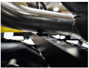
Remove 2 T40 Torx screws from above airbox.
