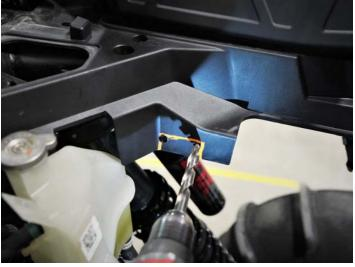
Finish cutting out the rectangle with an air saw or similar and debur as necessary
