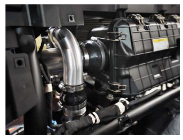
Install the hot side charge tube between the turbo and intercooler (Note: Short leg faces towards the turbo)
