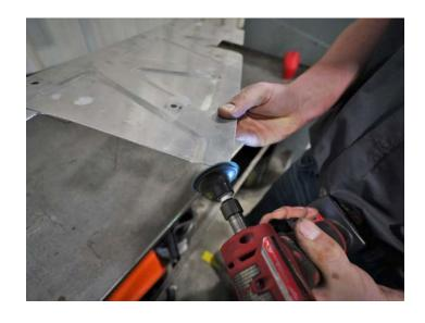
Reinstall heat shield in chassis using provided 8mm self tapping bolts.
