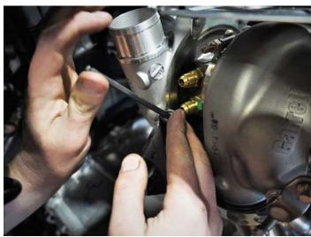
Install downpipe through from the rear of the vehicle as shown.
