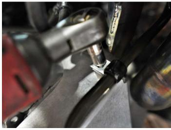
Install wastegate actuator on turbo bracket and tighten down nuts. Adjust the extension rod until it slides on the wastegate arm freely then go two full turns tighter. Install actuator E clip. Connect boost reference line from the turbo compressor housing to the wastegate actuator and secure with zip tie.
