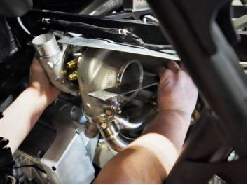
Remove 15mm bolt from transmission and install turbo bracket as shown.
