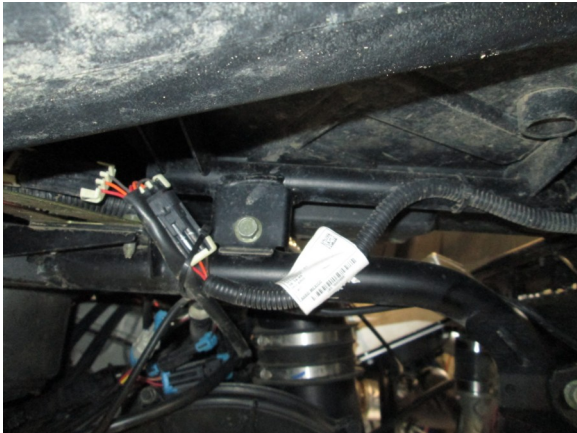
51. POWERING UP THE FAN Route the fan power harness from the fan and "T" into the taillight power harness located under the rear fender on the drivers side.
