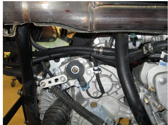
54. Look over all the hose routing to make sure the clamps are tight and there are no kinks or sharp bends in the hoses. Make sure to keep hoses away from sharp objects. Zip tie hoses.
