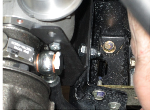
20. Route the 15" water line from the inside of the turbo to the 90 degree coming from the thermostat.
