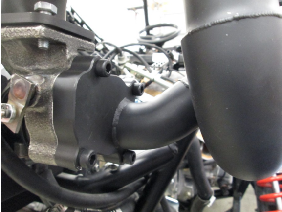
37. INSTALL TURBO OUTLET Fasten the turbo outlet to the turbo using the 8mm x 30mm allen head bolts.
