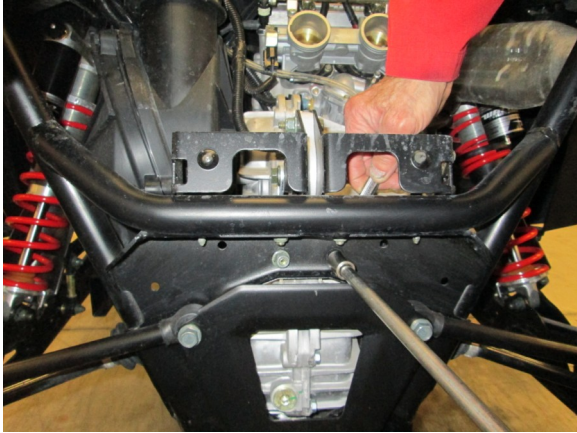
13. PREPPING THE STOCK MUFFLER BRACKET Remove the nuts from the lower rear engine mount bolts.
