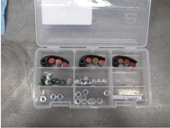
67. Install preloaded clutch weights
