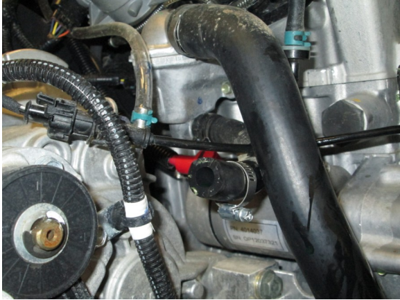
19. Rotate the 90 degree bend coming from the thermostat toward the rear of the machine.
