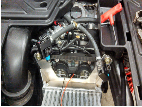
49. INSTALLING THE FUEL RAILS Apply assembly lubricant to the upper o-rings on the fuel injectors and insert them into the fuel rails.
