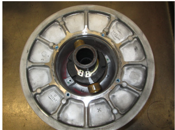
58. Remove bolts from helix, remove helix.
