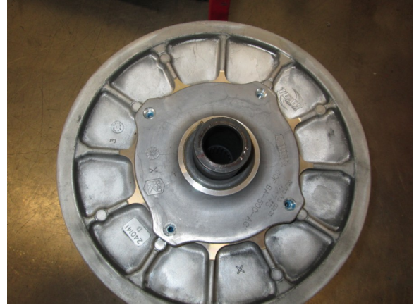
62. Reinstall the factory helix, Be sure to reindex to the marks made previously on step 59. Use blue locktite when reinstalling the factory screws.
