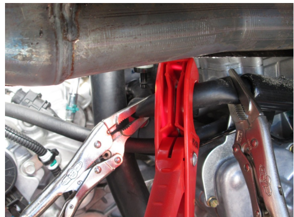
18. INSTALLING WATER LINES Follow the factory coolant line from the thermostat lamp each side of the 90 degree bend with vise grips. Make a cut after the 90 degree bend.
