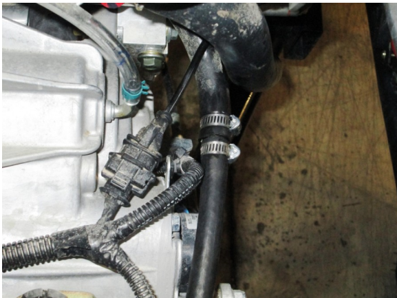
21. Trim line as needed, then install the 3/8" barbed union and fasten with 2 #6 hose clamps.
