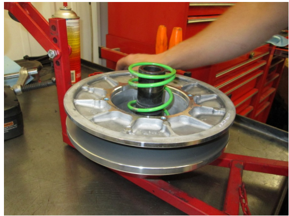
60. Replace stock spring with the provided Green/ silver spring. Roller holder is indexed to inner spindle. Install using the press.
