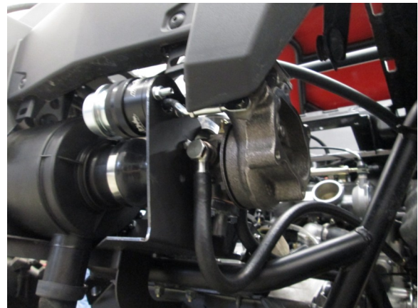
22. Route the 24" water line to the outside of the turbo to the open end of the coolant line cut in step 18.
