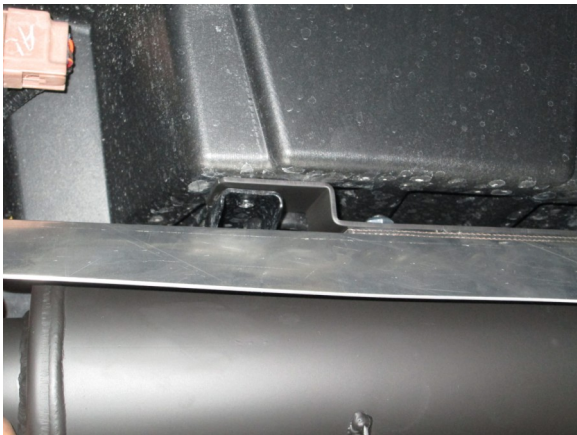
41. Pry the bed off of the mounting bracket and slide the muffler mounting tabs in between the bed and the bed mounting bracket. Loosen addition bed bolts if needed.
