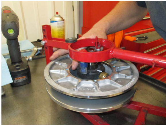
59. Get clutch press and remove snap ring. Make sure you mark the position of the sheaves, rollers and helix for reinstallation.
