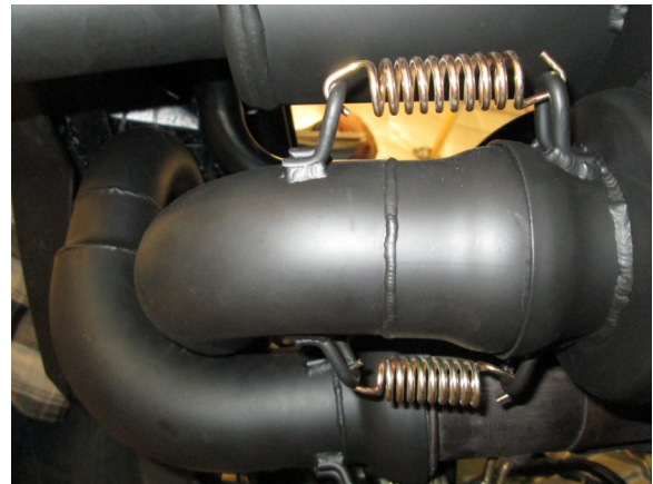
42. Align the muffler to the turbo inlet, outlet and tie down support bracket holes. Reinstall the support brackets and fasten the muffler to the outlet using the 2 provided gold springs.
