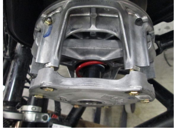
68. Install the red w/black and gold primary spring. Reinstall the clutch belt and clutch cover. Tighten all bolt to factory specs. Reinstall clutch cover and shock.
