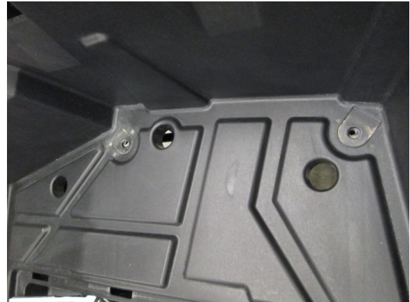
40. Remove the 2 passenger side tie down support brackets from the inside of the bed.
