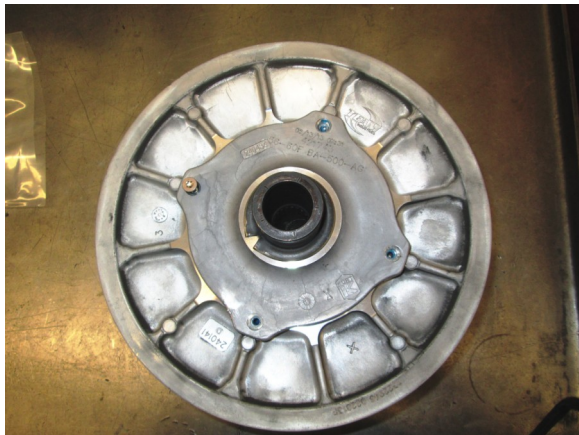
57. Remove the belt and secondary clutch.
