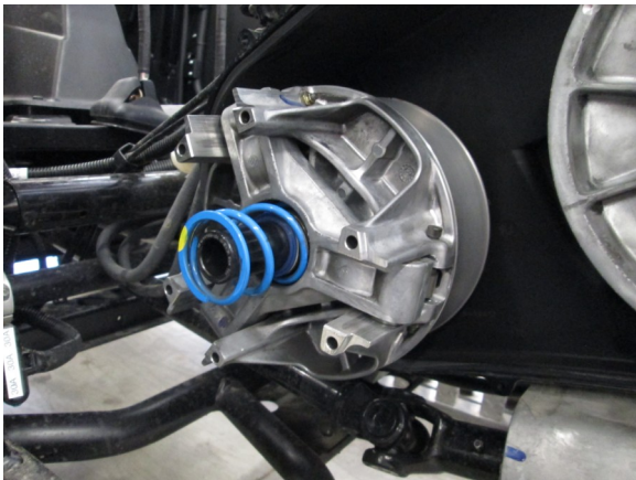
65. Remove clutch cover.
