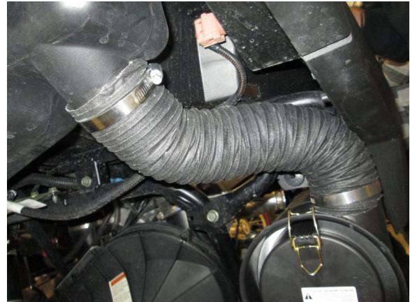
52. PLUMBING THE AIR CLEANER Install the provided intake hose from the Donaldson air cleaner to the factory air intake.
