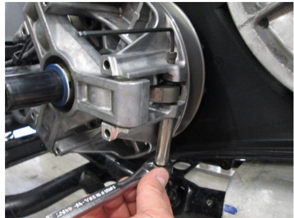
66. Remove clutch weights.
