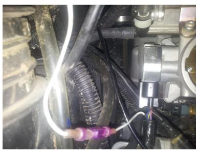
3. Tap the White wire to the Green Wire on TPS connector using supplied Heat Shrink Butt Connector. Shrink the ends using a heat gun.
