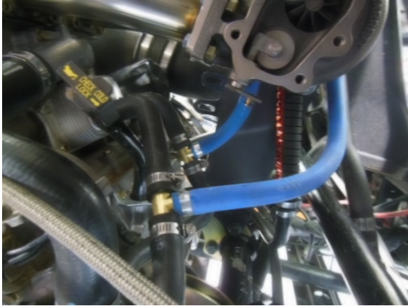
7. Cut engine oil cooler coolant hoses at mid point and T turbo coolant hose into each hose.
