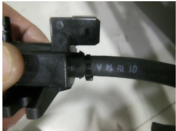
30. Connect 3/16" boost hose from charge tube fitting to metal fitting on boost solenoid. Secure hose to solenoid with zip tie.
