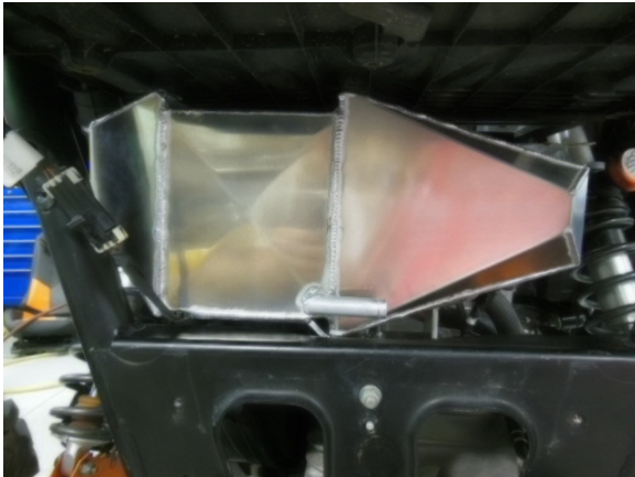
15. Install air box intercooler assembly. Adjust transmission bracket to position air box assembly so that there is clearance on all sides and corners.
