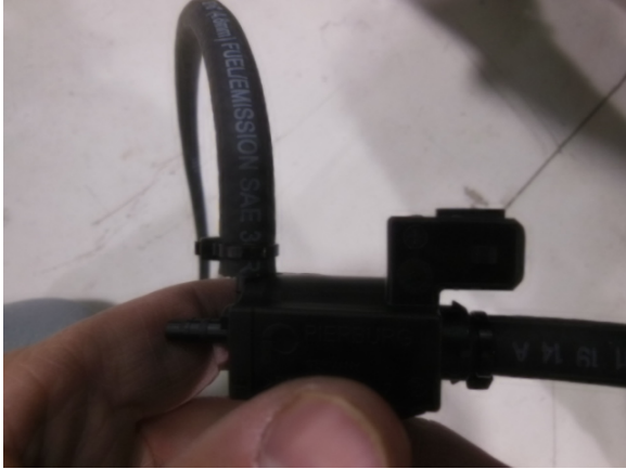
31. Connect 3/16" boost hose from waste gate actuator fitting to perpendicular plastic fitting on boost solenoid. Secure hose to solenoid with zip tie.
