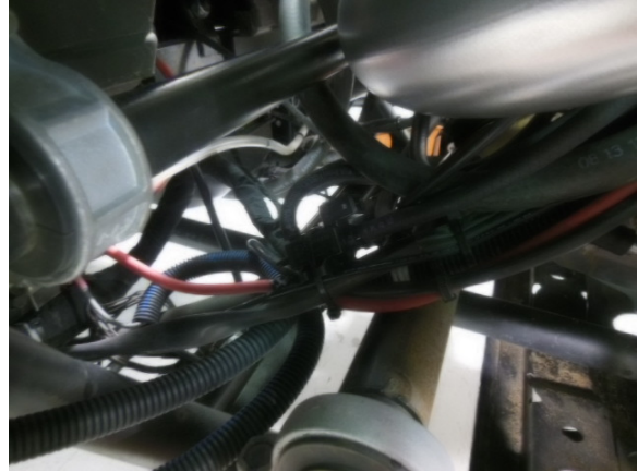
32. Secure boost solenoid with a zip tie to stock harness bellow sway bar.
