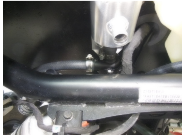
20. Remove belly pans and install coolant hose to water pump.
