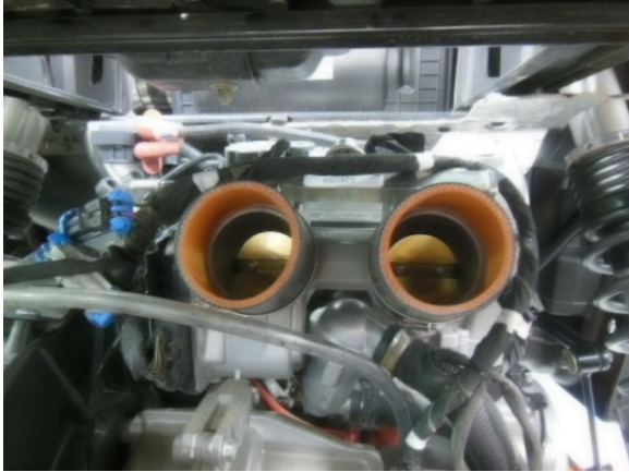
13. Install silicone hose to throttle bodies and secure with hose clamps.
