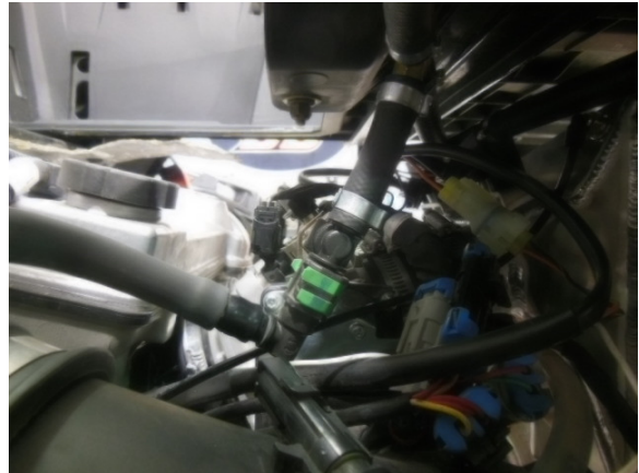
28. Connect stock fuel line to auxiliary connector.
