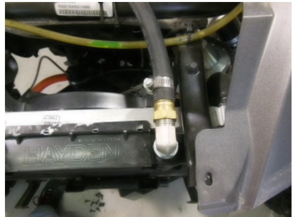
22. Connect remaining coolant hose to water cooler.
