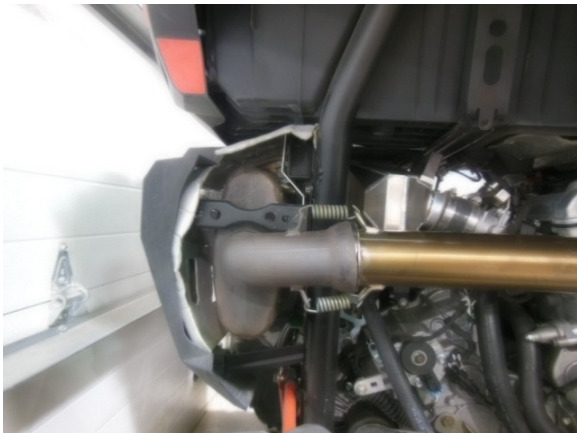
33. Install turbo outlet pipe and muffler.
