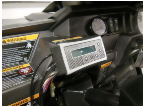
34. Install BoonDocker Control Box as per control box instructions.
