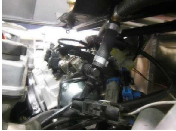
26. Connect auxiliary fuel line to stock fuel rail.
