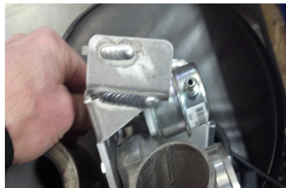
54. Route 3/16" line from 90 fitting on boost solenoid to the boost actuator on turbo bracket. NOTE: make sure to use small zip ties on ALL 3/16" hose connections to prevent blow off..
