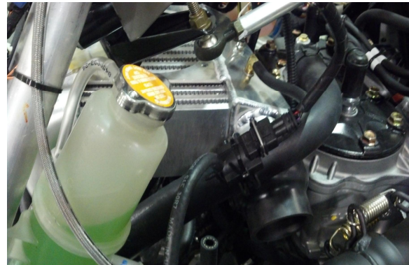
52. Install electronic boost solenoid using Velcro and zip tie to secure to coolant hose. Route 3/16" line from brass fitting to top of solenoid .
