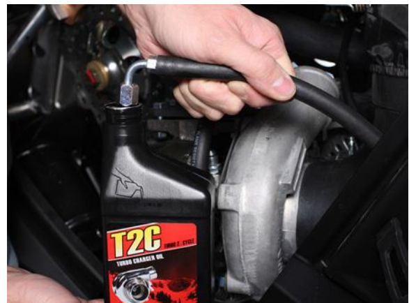
66. Start the Snowmobile to verify that the oil pump has power and the oil pump is pumping oil, when verified install the oil fitting on the turbo and tighten down.
