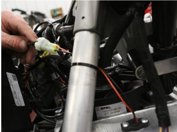
49. Locate the temp sensor wiring (located in rear of inner-cooler or in silicone air box) route and plug into control box harness secure with zip ties.
