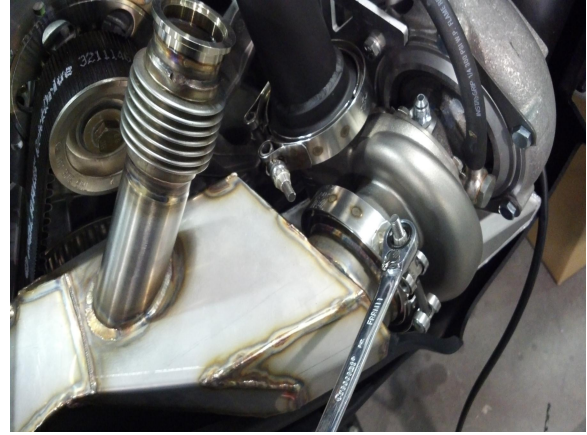
32. Install stainless muffer into tunnel and attach to turbo using v-band clamp make sure to properly align, seat, snug v-band do not tighten all the way.
