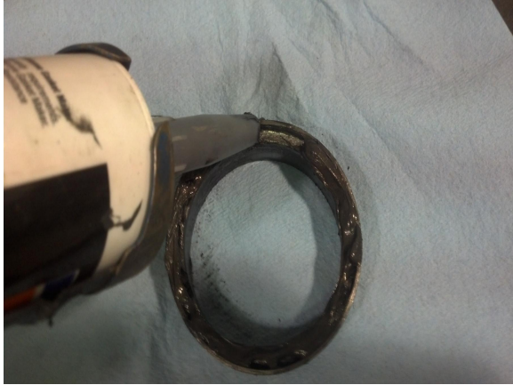
19. Remove pipe and exhaust donut. Silicone both sides of donut to ensure proper seal to Y-pipe and Pipe.
