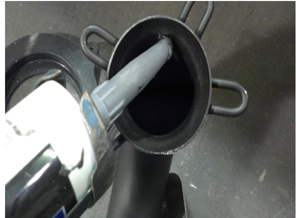
22. Run a bead of silicone on the bell of the turbo inlet pipe.
