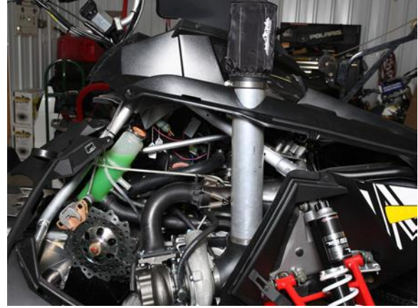
62. Install the aluminum pipe on the intake elbow, secure with a hose clamp. Install air filter on the pipe outside the hood and secure with supplied hose clamps
