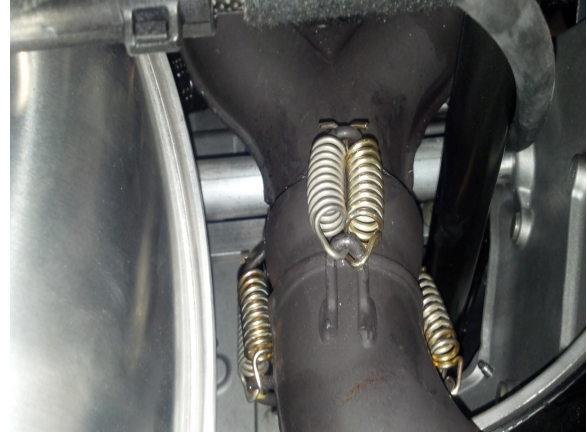
20. Spring pipe to Y-pipe using stock and supplied springs, double up springs on all spring tabs, this will prevent a boost leak. (Note: if sled is not building proper boost check donuts for seal)
