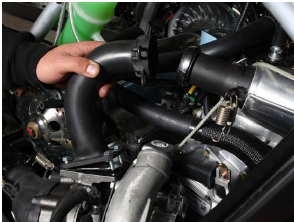
23. Install turbo flange gasket between turbo and inlet and bolt in place using the 4 supplied bolts and top lock nuts.
