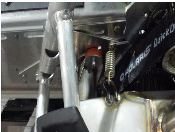
35. Spring muffer into place using short exhaust spring. (At this time finish riveting the kick plat in place, use inside rivet to adjust distance between muffer and kick plate)
