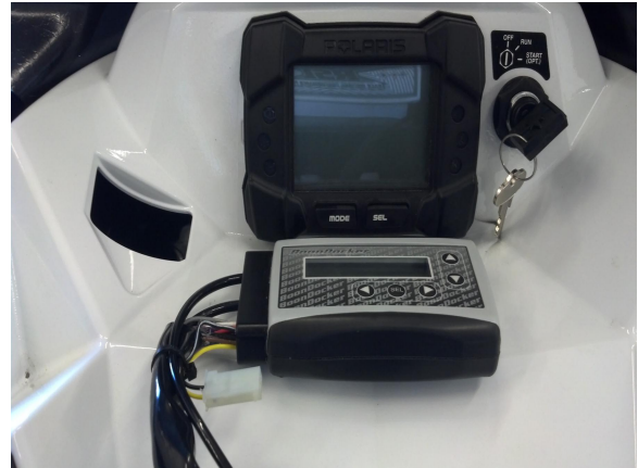
64. Reinstall-Fuel Tank, seat and Hood . Attach the control box using supplied Velcro Route the Boost pressure line from the control box to the push to connect fitting on the Air box or Cooler.
