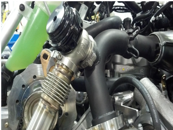
33. Install Tial external waste gate, rotate turbo inlet and muffer for proper alignment using supplied clamps snug waste gate into place do not tighten yet.
