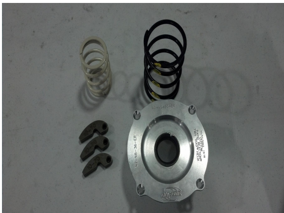
65. Install the Clutch Kit , Primary spring, and clutch weights, Install Secondary spring and Helix. Recommended helix start: 40-46-36, if less RPM desired 42-48-36 Faster up shift.
