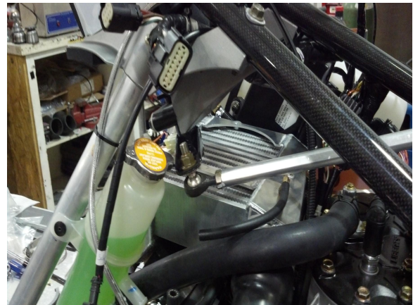
46. Install Torque building inner-cooler, (Tech tip, moving steering post may make install easier.) Adjust for clearance from cylinder head, electrical wiring, fuel filter, fan, and chassis before tightening.
