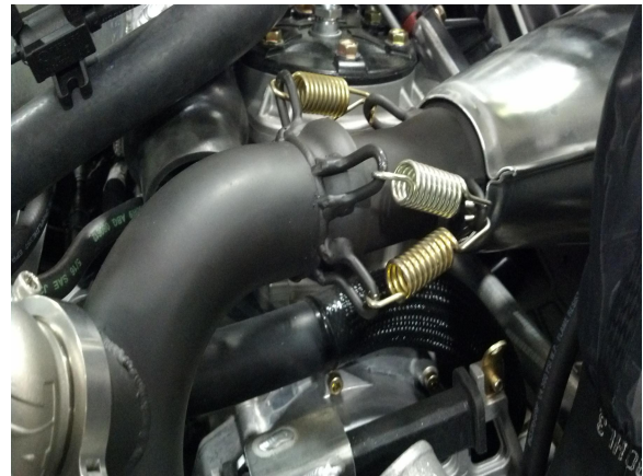
24. Spring inlet into place using the 4 long exhaust springs. Install springs long side towards pipe so springs do not touch.
