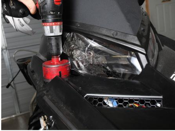
61. Using a 3ø hole saw drill a 3ø hole in the hood.
