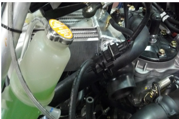
53. Locate solenoid power connector from the control box, follow stock wire harness over steering linkage over to boost solenoid and plug in secure with zip ties.
