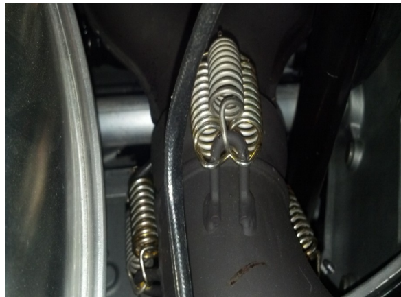
28. Install springs from pipe to Y-pipe 2-springs on side spring tabs and 3-springs on top spring tab.
