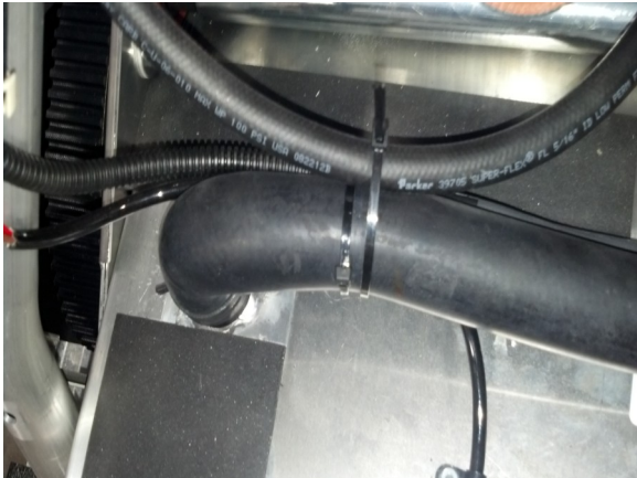
57. At this time check all routing! Check all fuel lines, wiring, and hose, make sure everything is properly secured and zip tied to prevent rubbing and chaffing!
