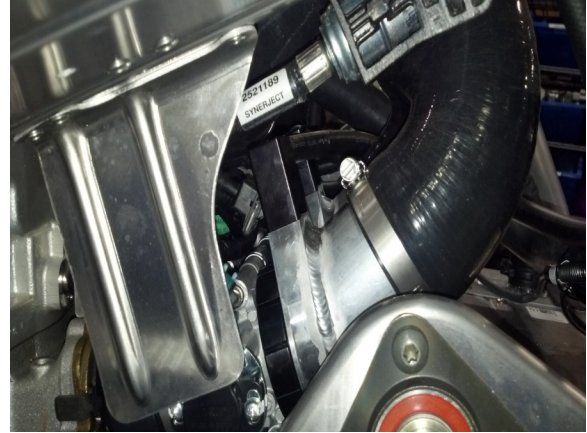
44. Install Torque building silicone air box, make sure not to slide on to far for proper jackshaft clearance. Tighten hose clamps.
