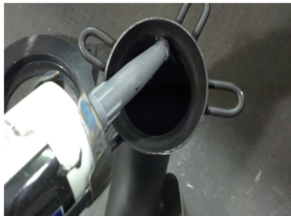
30. Run a bead of silicone on inside of the bell of turbo inlet pipe. Bolt inlet to turbo using 4 bolts and 4 hole gasket . If installing stainless Tial see next step.
