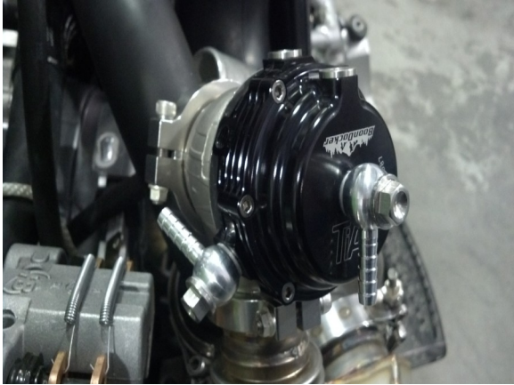
55. Install fittings on the waste gate as shown, Top cap 1-vent and 1-plug . Below Diaphragm 1-pressure Fitting, and 2-plugs, and leave the n2o ports empty.
