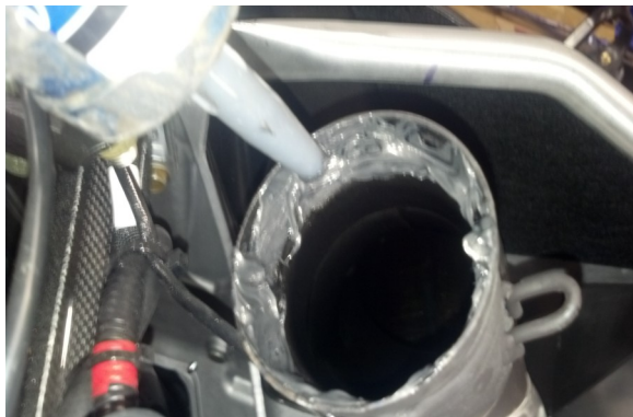
27. Run a bead of silicone on the inside of the flange on the exhaust pipe.
