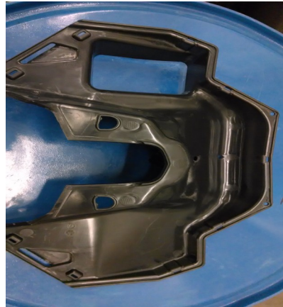
58. Remove the stock air intake plenum from under side of the hood. NOTE: heat on the tabs will help prevent breaking the tabs. Remove all internal ducting.
