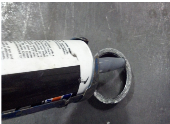
29. Run a bead of silicone on inside of the small exhaust donut and install on pipe
