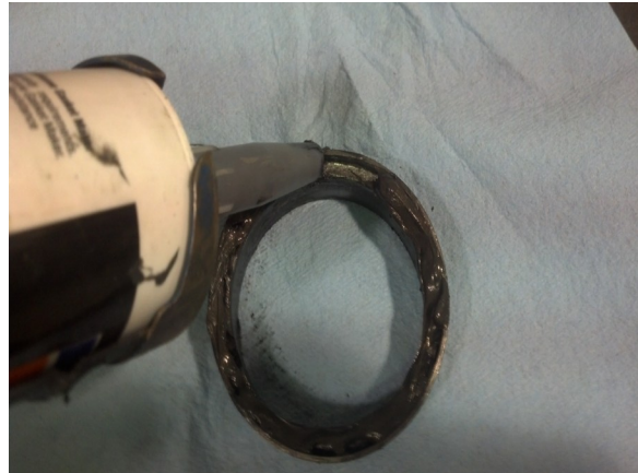
26. Remove the stock pipe from Y-pipe, remove the exhaust donut and run a bead of silicone around inside and reinstall on Y-pipe, Note: make sure to align notches on Y-pipe to donut
