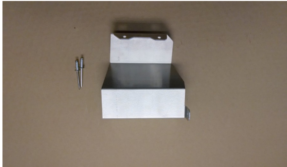
25. Install foot rest kick plate. (Note: install kick plate “only install the 2 lower rivets on top running board at this time”) the last rivet will be installed later to adjust clearance
