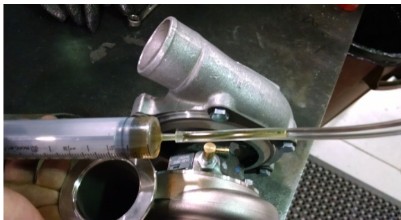
23. Use the 36" supplied oil line and protective sleeve and route to the turbo, avoid sharp edges and heat, zip tie where necessary. Before attaching lines, fill oil lines with injection oil, attach turbo oil line to port labeled #1. Use 7 1/2" supplied line and route from port labeled #2 to PTO crank bearing. Use stock clamps to secure lines to oil fittings. WARNING lines MUST be plugged in proper ports. Prevent engine damage!
