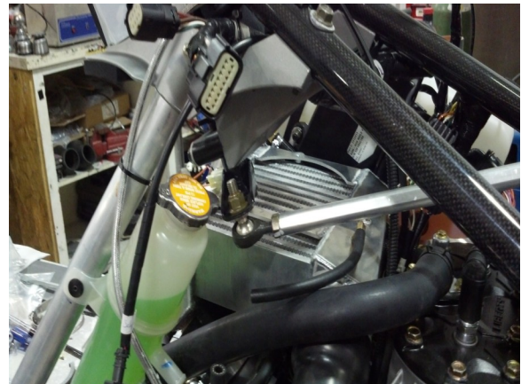
46. Install Torque building inner-cooler, (Tech tip, moving steering post may make install easier.) Adjust for clearance of head, electrical wiring, fuel filter, fan, and chassis before tightening
