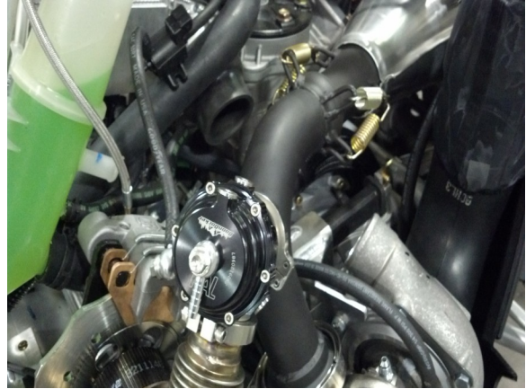
56. Route 3/16" line from the 90 fitting on boost solenoid to air fitting on external waste gate on lower diaphragm .
