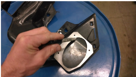
59. Cut out the provided template and position on plenum as shown. Template will follow plenum mold. Trace the oval hole as shown.
