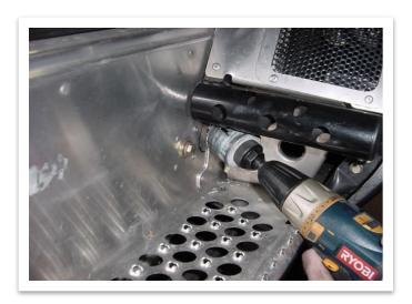
B. Using a 2 ¼" hole saw. Drill the center of the newly traced outlet hole.
