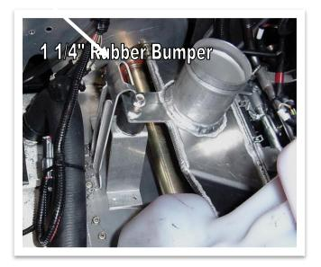
B. Make sure the air box and throttle bodies are slid all the way in place. Using a 3/16" drill bit, drill the 2 holes towards the rear of the sled first (this will keep the bracket from moving while riveting the front holes). Fasten the bracket with the supplied rivets. Now drill and rivet the front holes.
