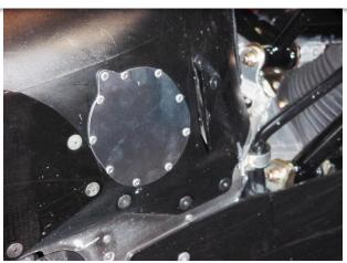
D. Rivet the remaining 9 holes but be sure to set rivet washers on the opposite side of every rivet.
