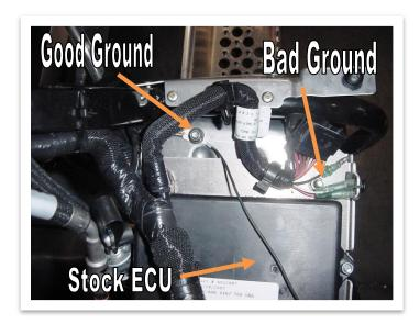
B. Ground the eyelet from the Plug and Play harness to the bolt that is shown above. There are 2 locations to choose from be sure to use the one as shown. The other bolt is not a good ground source. Tip: The good ground will already have a factory eyelet grounded to it. (See picture).
