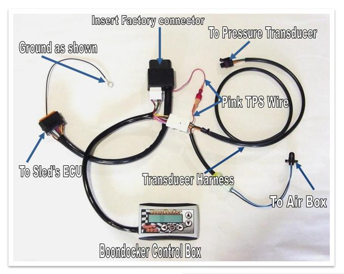
C. To mount the control box find a suitable location with easy visibility and access, you will be using the Boondocker Control Box for tuning and for visual references. Set the control box in place with the provided Velcro.
