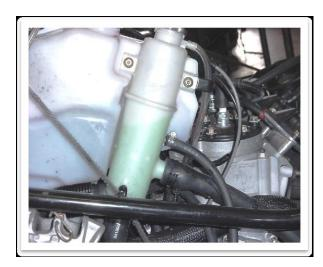
B. Locate the shorter water hose. This hose will mount on the inside of the turbo and route to
