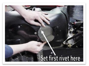
B. Place the block off plate over the outlet hole. Set your first rivet in the existing hole as shown. Be sure to place a rivet washer on the back side of the rivet and then rivet in place. Note: you can also use silicone for a more water proof seal.
