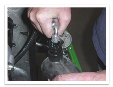
D. After verifying the pump is working, re-install the oil inlet to the turbo.
