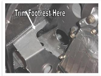
F. Vacuum all shavings from sled and remove the covers from the turbo charger. It is a good idea to double check the turbo for any debris that may have entered the turbo. Vacuum if necessary.
