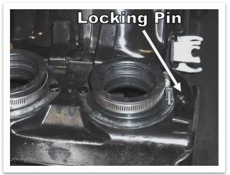
E. Remove the TBAP sensor from the air box, Reconnect it to the factory connector and find a new place to mount it. We chose to zip-tie it to the wiring harness on the clutch cover.
