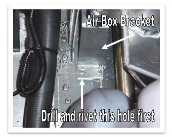
C. After riveting the bracket in place tighten the 5/16 lock nut on top of the air box bracket.
