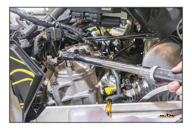
Using a torque wrench, set at 25-ft-lbs, properly tension each head bolt.
