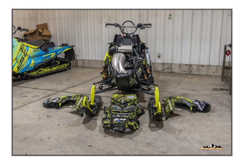
Re-install console panel, with body-panel-darts, clutch tool, hood (be sure to connect intercooler power if applicable), and side panels.
