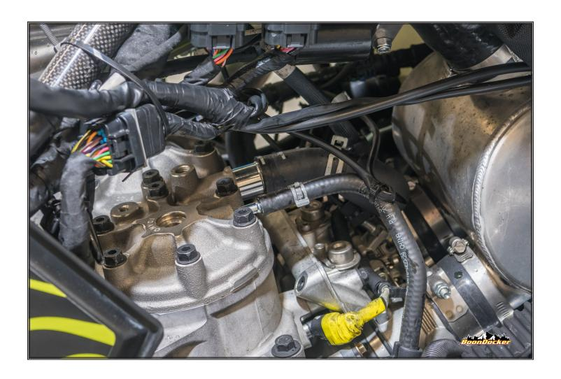
Slide the coolant lines back on to the barbs on the head. You may need to use WD-40 to provide some lubrication. The image is meant to show the operation: please slide the coolant lines ALL-THE-WAY onto the barb, with no "reveal".
