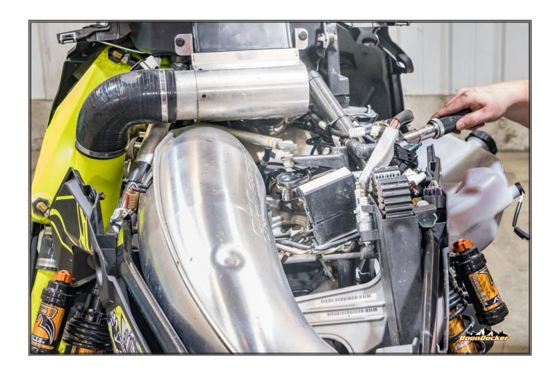
Reinstall the factory "Knock" sensor. Tension the bolt to 14-ft-lbs. Clock the sensor as per the Polaris service manual (see next slide)
