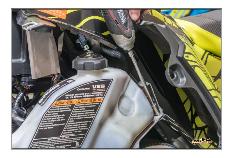
Use a 10mm socket to remove the clutch guard
