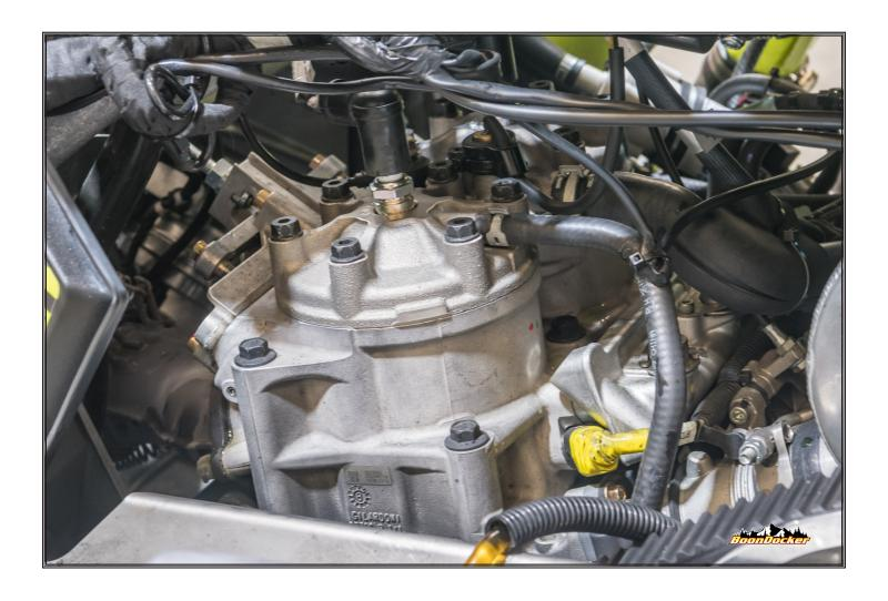
Reinstall spark plugs and spark plug caps. Pay attention to the labeling on the plug wires, identifying PTO and MAG side. Replace any zip-ties cut during installation. Verify routing and ensure all hoses & wires are properly restrained to prevent chaffing.
