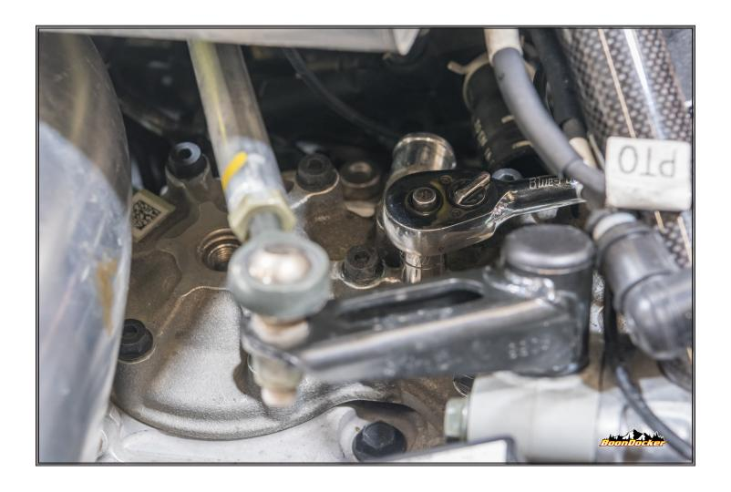
Using a 13mm socket, fully loosen all head bolts. Remove all bolts except the one under the pipe.
