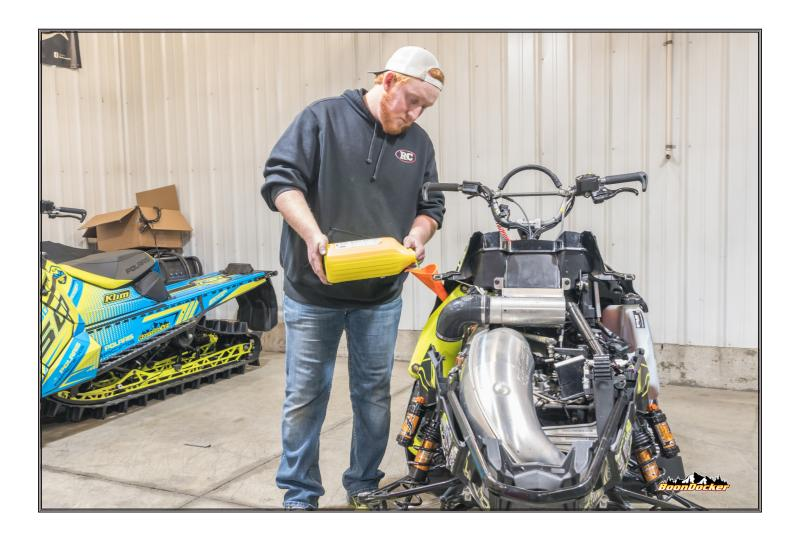
Refill coolant. These heads are self-bleeding. Allow coolant to drain through head. Refill coolant bottle again. Start sled and bring coolant temp to 80F. Check coolant reservoir and add coolant as necessary.
