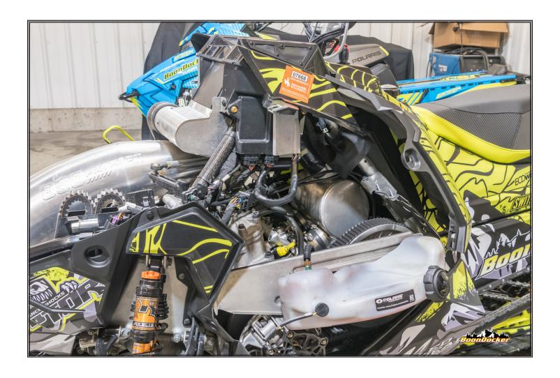
Lay the clutch guard/oil tank to the side. Restrain the tank to prevent damage to tank. Do not strain oil line.
