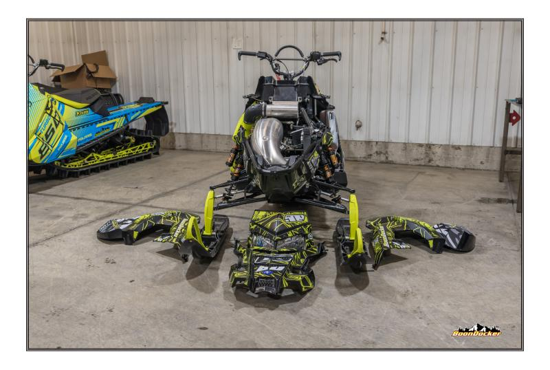
Remove side-panels and hood. If your kit is intercooled, please disconnect power for pump.
