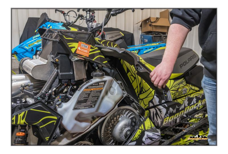
Allow panel to flex, so you can access the bolts that secure the clutch-guard.
