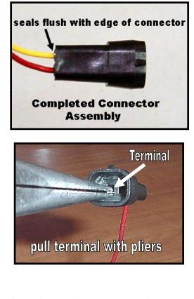
4. If a terminal must be removed, use pliers to carefully push the terminal out of the connector. The terminal can usually be re-inserted one more time. Don't do this unless necessary! The terminal tabs need to be pried up slightly before re-inserting. See photo of terminal at right for tab location. Use a 1.2mm or 0.050" jeweler's screwdriver to pry with. Check to be sure that the wire can resist a slight tug without coming out.
