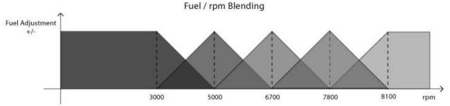
The fuel adjustment rpm ranges are blended as shown in the picture above. This allows for a broader range of adjustments with fewer steps. Each fuel setting is centered at a particular rpm value, in this example: 3000, 5000, 6700, 7800, 8100rpm. Each region is blended with the region below and the region above it as shown. For example, if the rpm is at 4000, the adjustment value will be half the value of the 3000 setting plus half the value of the 5000 setting.
