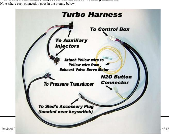
Install the Yellow wire on the Turbo Harness onto the Yellow Exhaust Valve Servo Position Sensor wire as follows:
