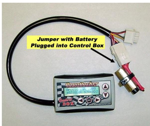
The battery connector can be left plugged in during engine operation, but the nitrous harness (if used) cannot be plugged into the Control Box. The battery will eventually drain if left connected to the box, so it is best to disconnect the battery when not in use.
