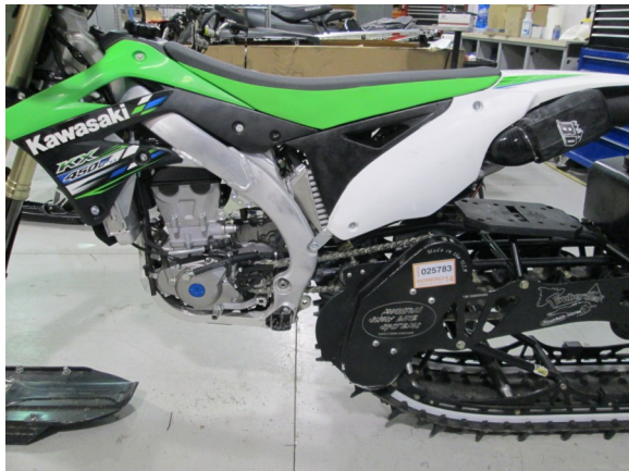
21. Install side panels, and seat.
