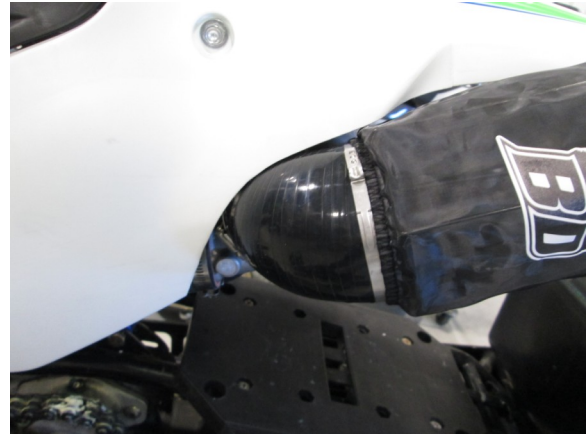
20. Cut left side of rear panel to fit air filter.
