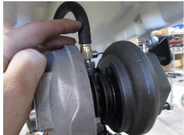
22. Start bike, check oil pressure and check for leaks. You might have to cut co length.
