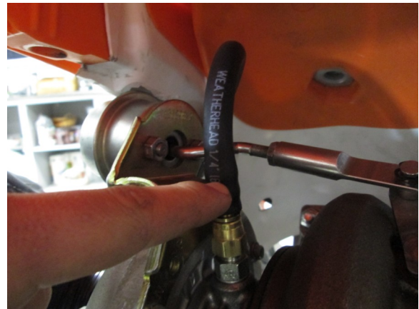
22. Undo oil feed line. Start bike and check to make sure oil is feeding the turbo. Run the line into a oil container. Then put back on & tighten line.
