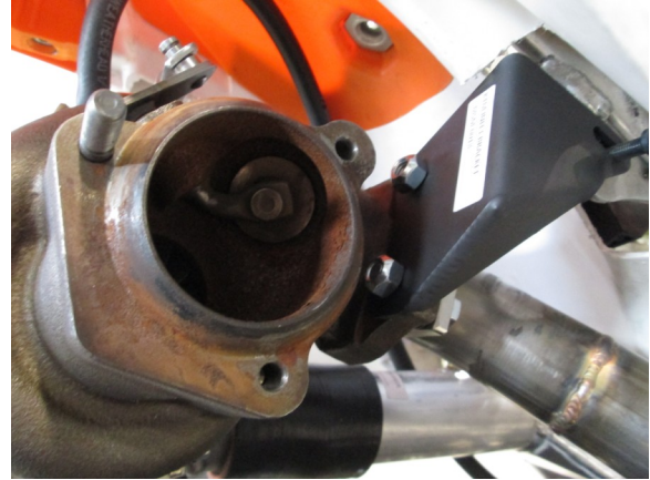
14. Place turbo in place and mount inlet bracket on the sub frame, header inlet and turbo inlet. Place bolts in and nuts on, leave loose.
