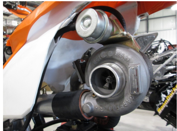
16. Rout oil feed line and drain line to turbo. Tighten drain line clamp and feed line nut. Zip tie boost line to the actuator.
