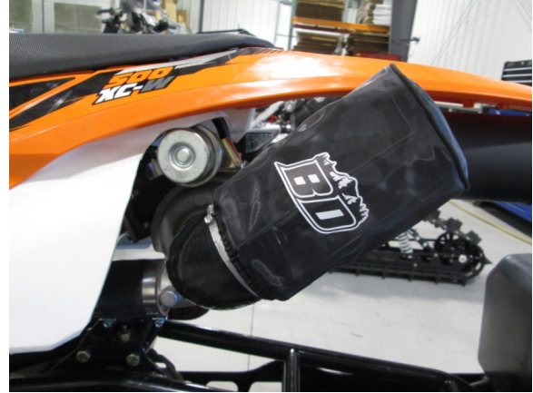
20. Install inlet and air filter, position as shown then clamp down.
