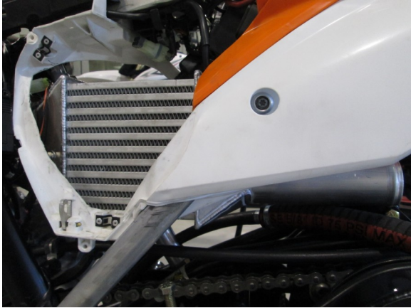
19. Zip tie wire harness, lines and adapters away from intercooler. Tighten all hose clamps and zip tie boost line ends.
