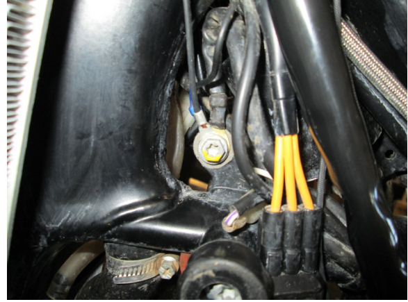
8. Route black ground to the stock ground bolt. Or the battery ground if you have a battery.
