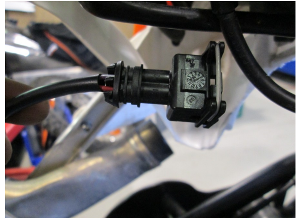
10. The Auxiliary injector connector is similar to the solenoid connector. It is shorter and has a Violet and Red wire.
