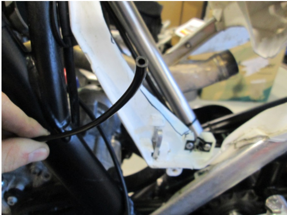
9. Boost line routes with boost solenoid adaptor and hooks into the "push to connect" on the intercooler.
