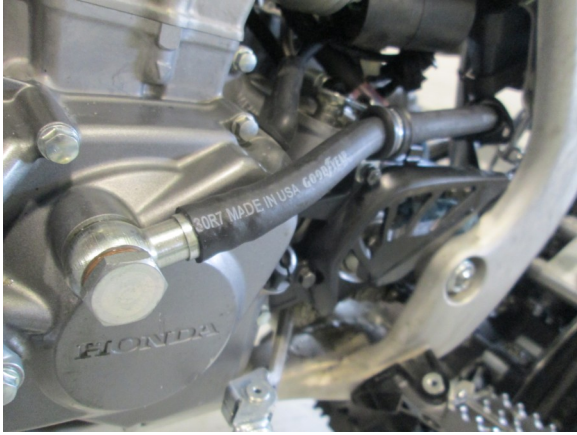
7. On the banjo bolt 2 copper washers on the inside, 1 on the outside by the bolt head. Route along right side of Timbersled frame to the turbo.
