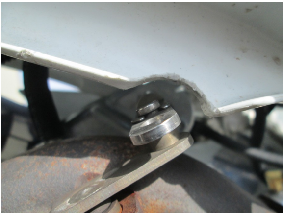
11. Trim fender as shown to clear the waste gate actuator rod.
