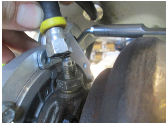
22. Route feed line through hole in the fender to the feed line fitting on the top of the turbo.
