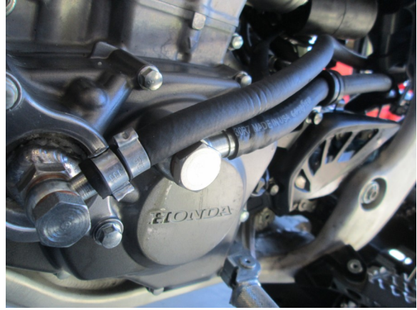
8. Route oil feed line along drain line till the back of the intercooler. Use smaller bolt and copper washers then tighten down on oil filter cover.
