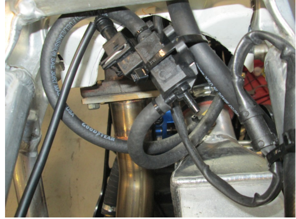
2. The connector with the violet/white and red wires go to the boost solenoid.
