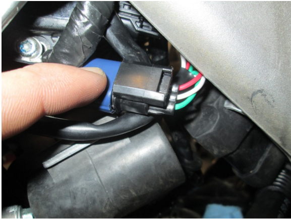
7. Control box adaptor with Red, White and Green wires into the Throttle Position Sensor.
