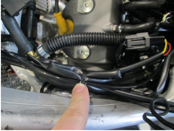
13. Be sure to zip tie wires down to stock harness so there wont be rubbing or melting of the control box harness.
