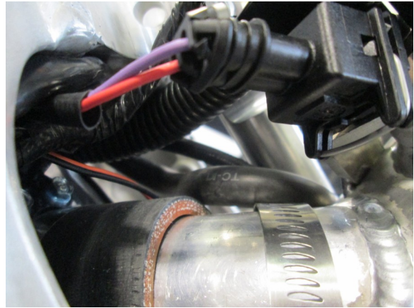
8. The Connector with Red and Purple wires go to the Auxiliary injector on the intercooler.
