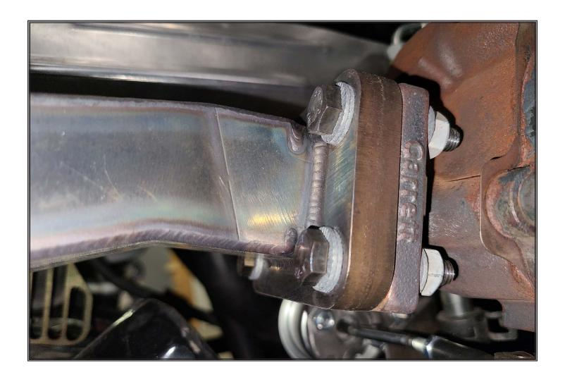
Bolt Turbo to header with supplied bolts, nord lock washers and lock nuts. Note: 4 bolt metal turbo gasket (zip tied to turbo for shipping) goes between header and turbo flanges.
