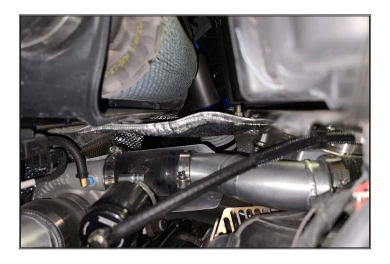
Install S shaped charge tube to turbo using silicone T.
