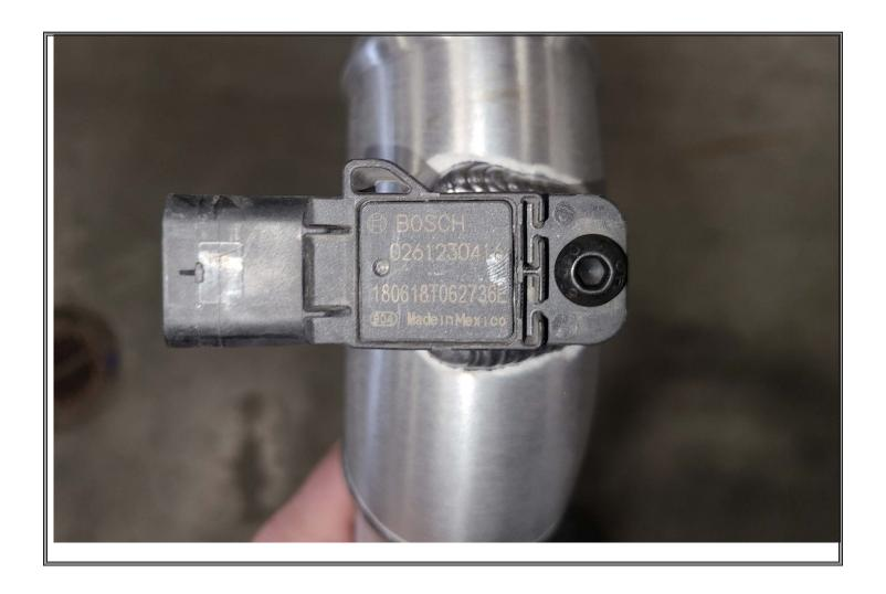
Install MAP sensor from factory charge tube into new charge tube using suplied bolt.
