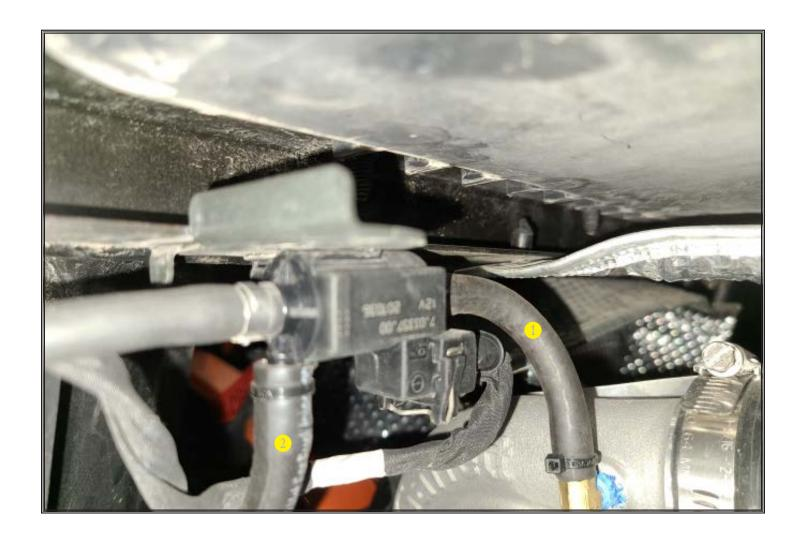
Install suplied Fuel Line 1 to brass 90 on turbo.
