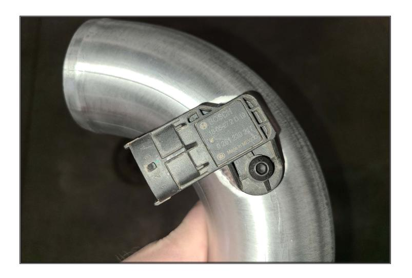
Remove T-BAP sensor from factory intake tube and install on new intake tube using supplied bolt.
