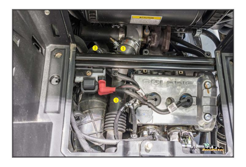
Remove charge tube **1** and BOV **2**Unplug TMAP sensor before removal, take care not to damage clip on connector.
