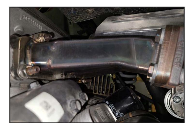
Clean gasket material from exhaust flange surface on head. Install turbo header and new header gasket with factory fasteners.
