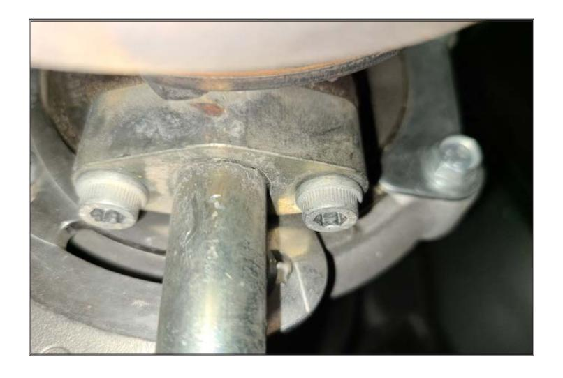
Uninstall factory oil drain from turbo.
