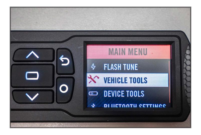
Once your PV3 is attached to your OBDI it will power on displaying it's gauges. Press the select button located between the arrows facing up and down. When you press the select button your main menu will open, use your arrows to highlight "VEHICLE TOOLS" then select it.
