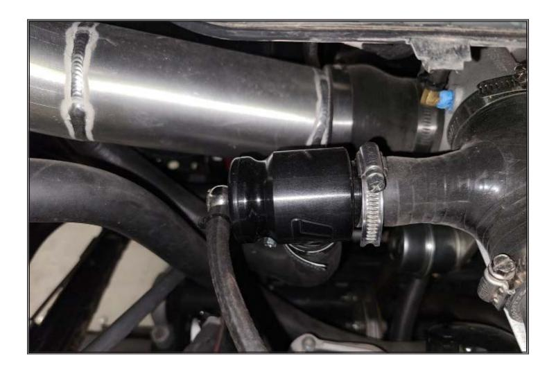
Re-install blow off valve using suplied long Fuel Line 3 (reference kit photo), replace factory BOV hose.
