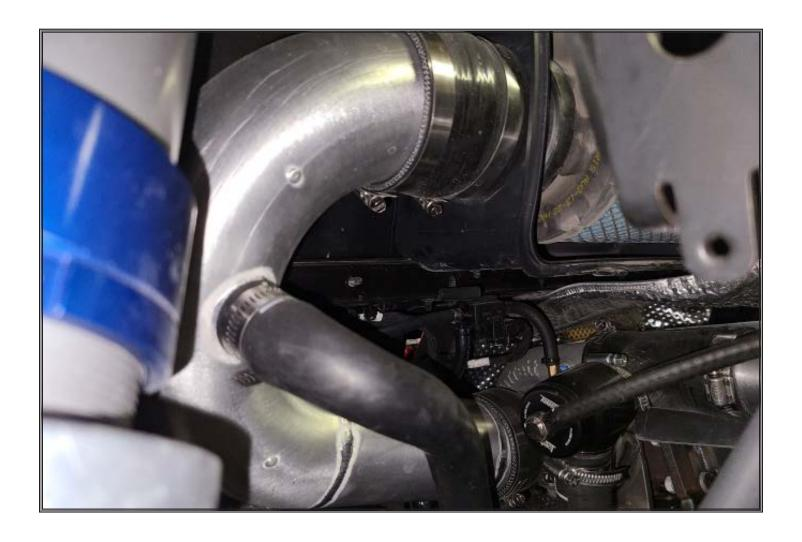
Install Cold Air Intake Tube to factory Airbox and turbo using supplied silicone.
