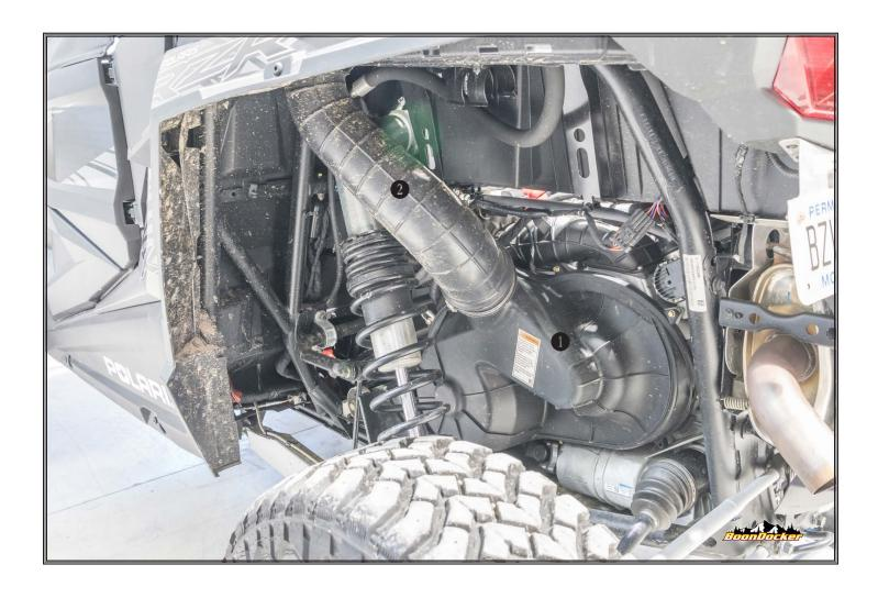
Remove rubber clutch vent **2** and clutch cover **1** as on ssembly, it will drop out the bottom between the trailing arm and frame.
