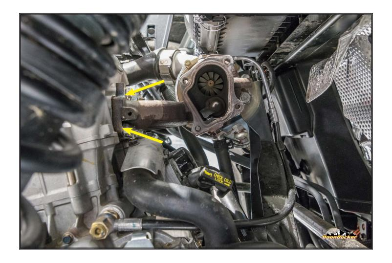
Remove oil feed and drain lines from OEM turbocharger, take care not to damage as they are reused later in installation.
