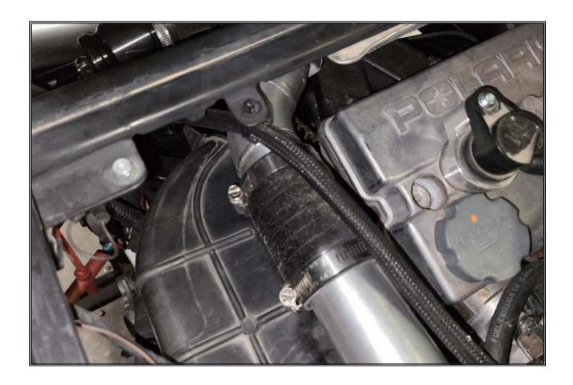
Connect charge tubes together loosely using supplied straight silicone.
