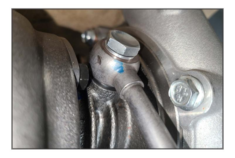
Install factory oil feed line to turbo with suplied banjo bolt and washers.
