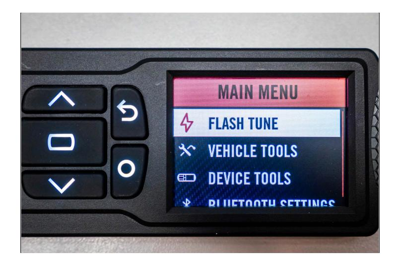
Plug the PV3 into the OBDI port as done previously. Use the buttons to select "Flash Tune"
