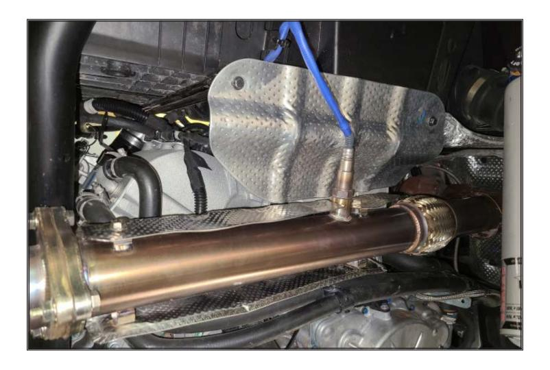
Install both factory down pipe heat shields to new down pipe with suplied flange bolts.
