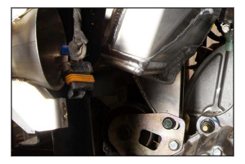
install two supplied bolts between intercooler and bracket.
