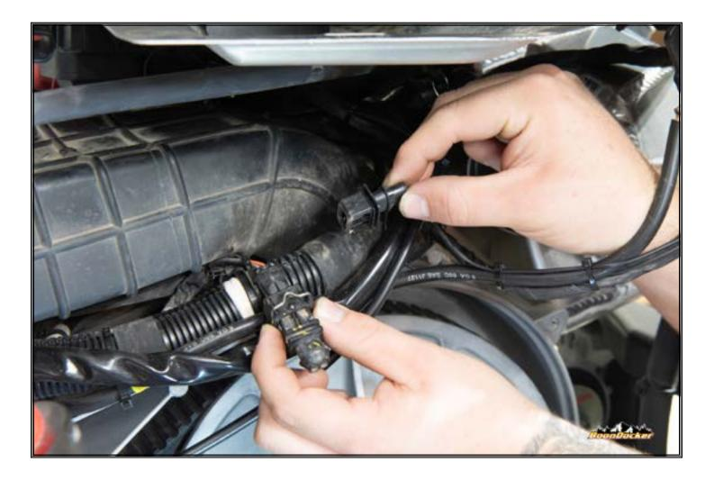
Connect supplied wire harness to water pump.
