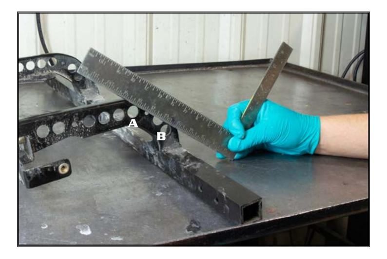
Mark crossbar as shown and cut to provide radiator clearance. We've used a square to line up the tops of these two (A and B) circles.
