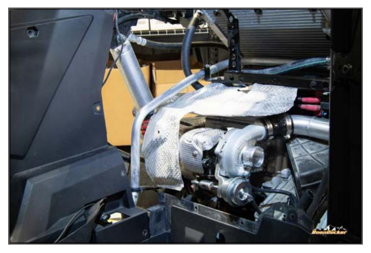
Route ground wire for the water pump to chassis common ground.
