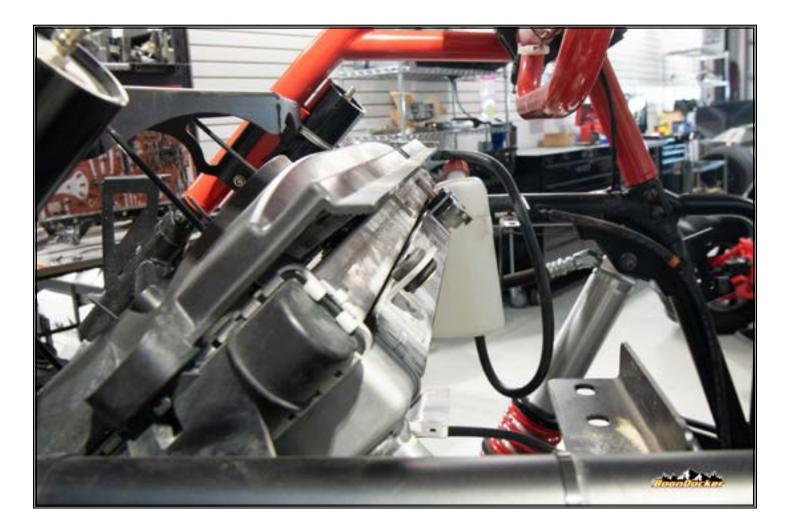
Install foam to ridges to ntercooler radiator to prevent rubbing.
