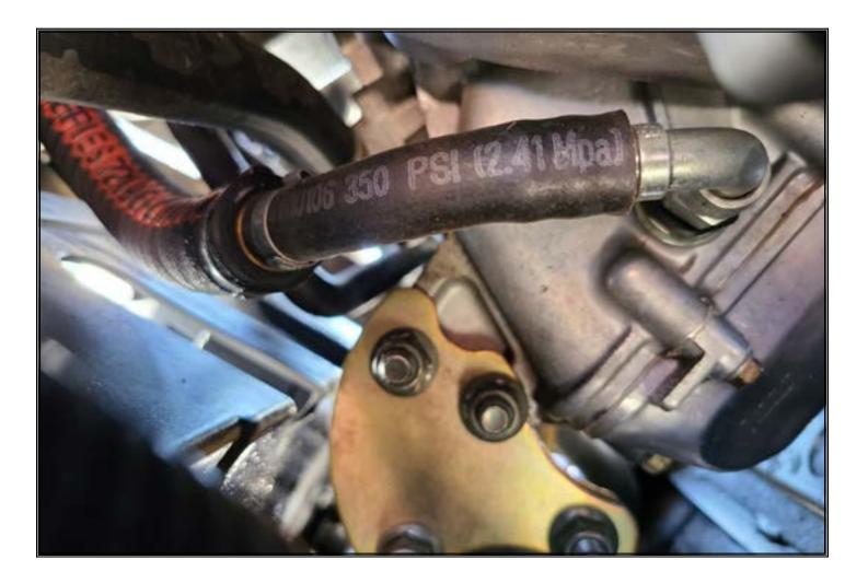
Install oil drain fitting located below and in front of clutch cover.
