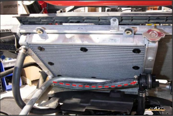
Connect coolant hose to PTO side of intercooler.
