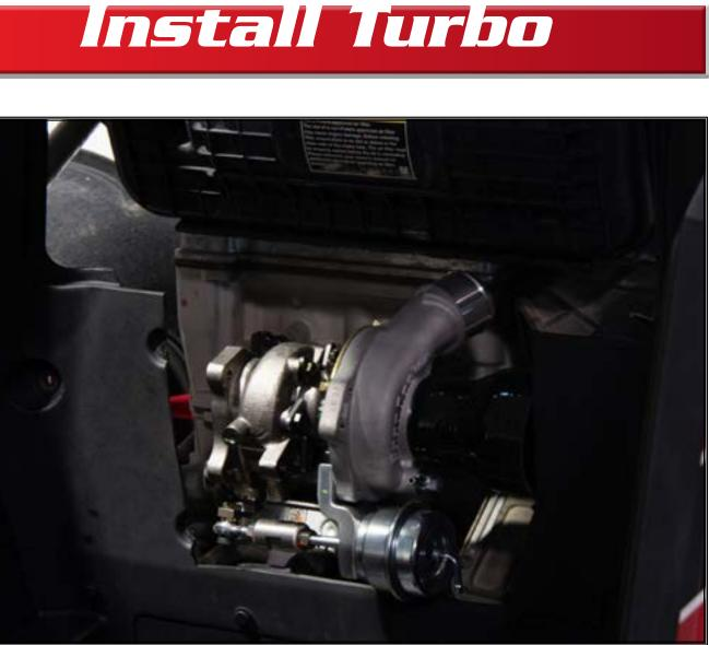
Install blow off valve and filter to BoonDocker Intercooler(A). Install boost reference line from throttle bodies to BOV(B).
