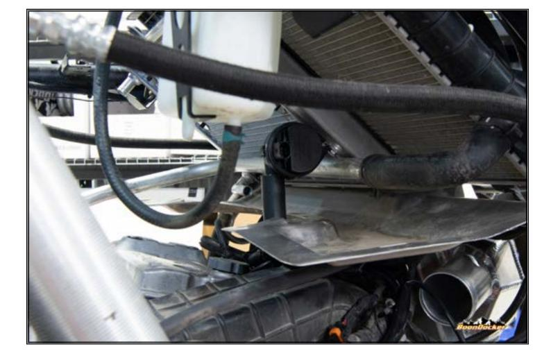
Install water pump and coolant hose hold down to radiator as shown.
