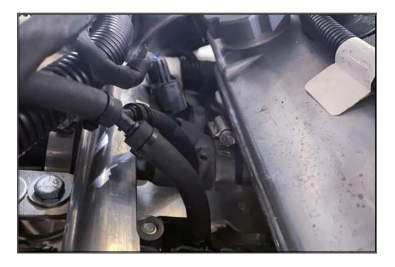
Rotate fuel line as shown and connect to BoonDocker fuel rail. Ensure line is routed in a way that it is not kinked or pinched.
