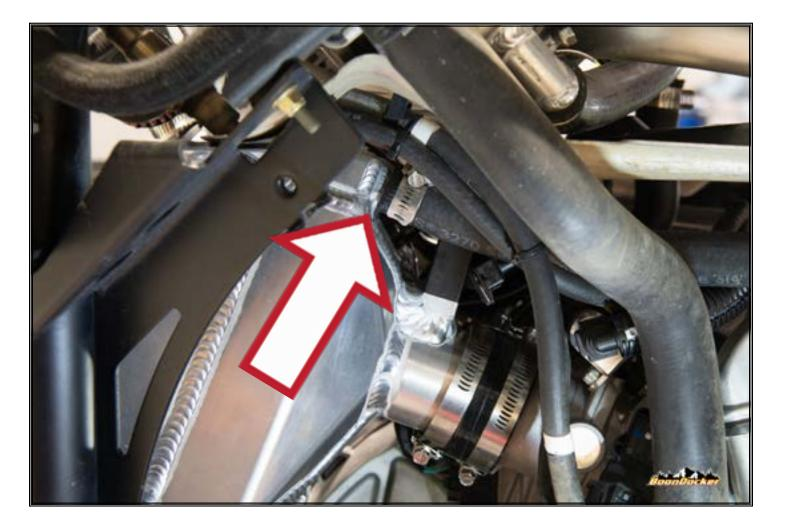
Route coolant hose from top of radiator down to MAG side of intercooler.
