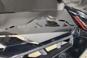
9. On the Right side of the hood, Bolt the previously removed ear to the hood mounting the De-Lite between the ear and the hood.
