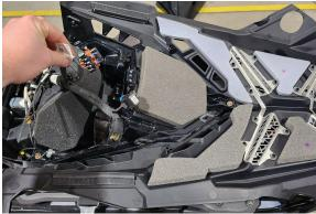
1. Remove the wind deflector from the hood by pulling the deflector away from the hood until the 3 panel clips release from the rubber grommets.
