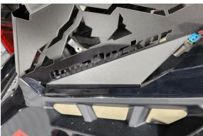
7. Starting on the left side of the hood, Bolt the previously removed ear to the hood mounting the De-Lite between the ear and the hood.
