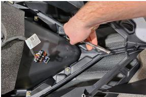
5. Using a t 25 torques remove both left and right ear plastics located at the back of the headlight hole.
