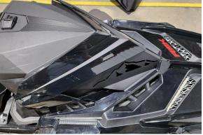
11. Using a t 25 torques Tighten the four gold bolts holding the top of the storage box to the hood.
