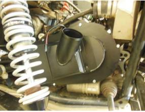
9. Install outer clutch cover. Use the 5/16 hex head bolts with nylon lock nuts to tighten the two clutch covers together. Clear, weatherproof silicone may be used if desired.
