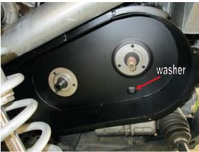
3. Place inner half of cover, front seal guard with lip facing outward and rear washer plate on engine. Apply blue thread lock onto (7) M6 screws and install. The lower screw uses the (1) alum washer.
