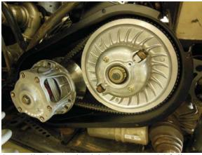
8. Install primary clutch bolt, torque to 96 ft-lbs. Install new secondary clutch bolt, torque to 40 ft-lbs.
