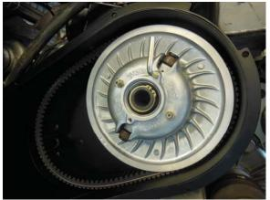
6. With belt on clutch, install secondary clutch onto jackshaft.
