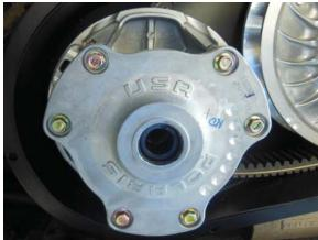
7. Install primary clutch by sliding the belt on to the clutch then slide the clutch onto the tapered drive shaft.
