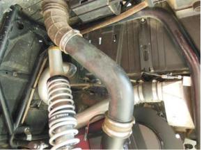
15. Using the included hose clamp, attach the plastic breather hose to the stock breather location.
