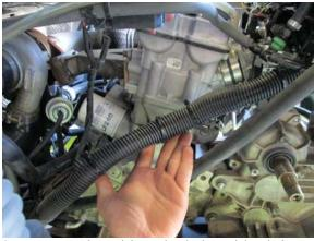
2. Inspect engine wiring, check that wiring is intact and not chaffed. Install protective tubing onto engine wiring and tightly zip tie tubing closed.
