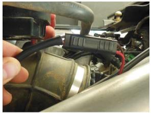
11. Plug the fan connector into the fan harness then carefully route the wires so they do not melt or rub.
