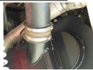
14. Install the 45 degree plastic breather hose onto the clutch cover using the stock rubber connector piece and stock clamps as shown.
