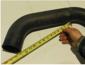
13. Measure 13" from the end of the 45 degree plastic breather tube as shown. Mark then cut the plastic breather tube. You will not need the existing 90 degree piece.
