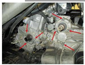
1. Remove the drive belt, primary clutch, secondary clutch, and stock clutch cover. Clean engine area and blow out screw holes.
