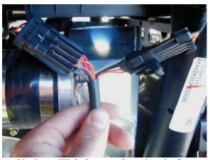
10. Unplug taillight harness then plug the fan harness in line with the taillights as shown.
