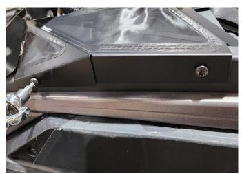
4. Install intake box with factory T40 Bolts.
