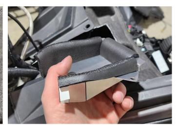
1. Remove hood, plastic center piece & T40 bolts from top of console Shroud.
